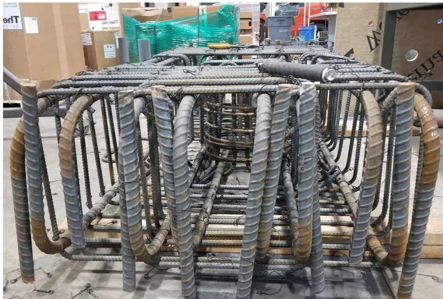
Figure 3.1 Reinforcement cage of footing
