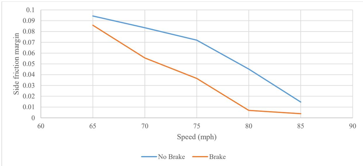
c) The impact of brake application on snowy road surfaces for the semi-trailer truck
