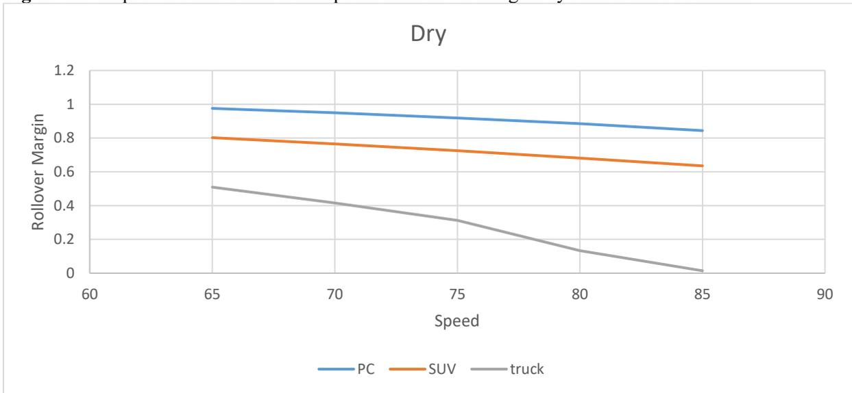
**Figure 3.7** Impact of vehicle type on rollover margins
