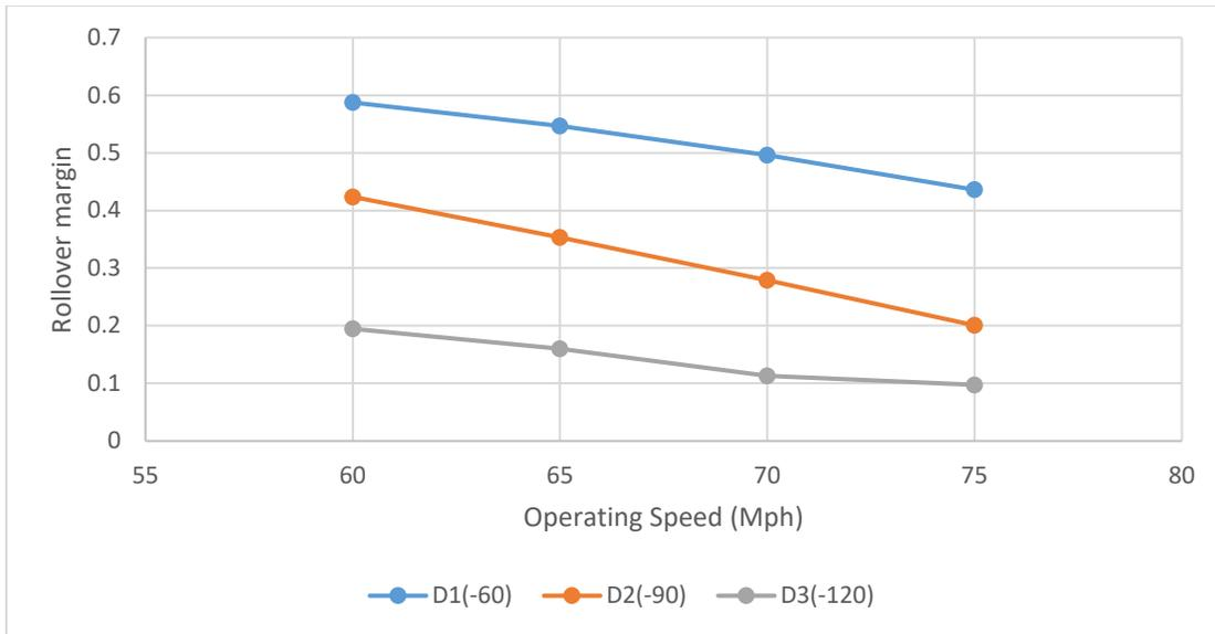
**Figure 5.8** Rollover margins for different crosswind directions
