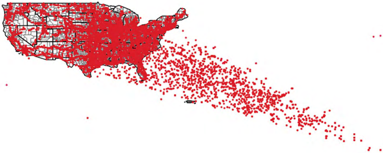
Figure 3.1 Systematic error in the geospatial coordinates of accident locations
