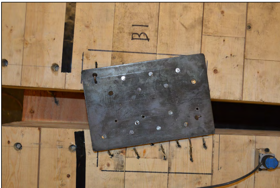
Figure 4.6 Connector B1 after the Test (Top View)
