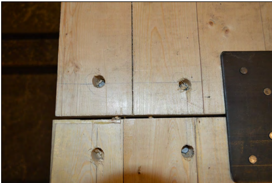
Figure 2.4 SDS Screws into CLT
