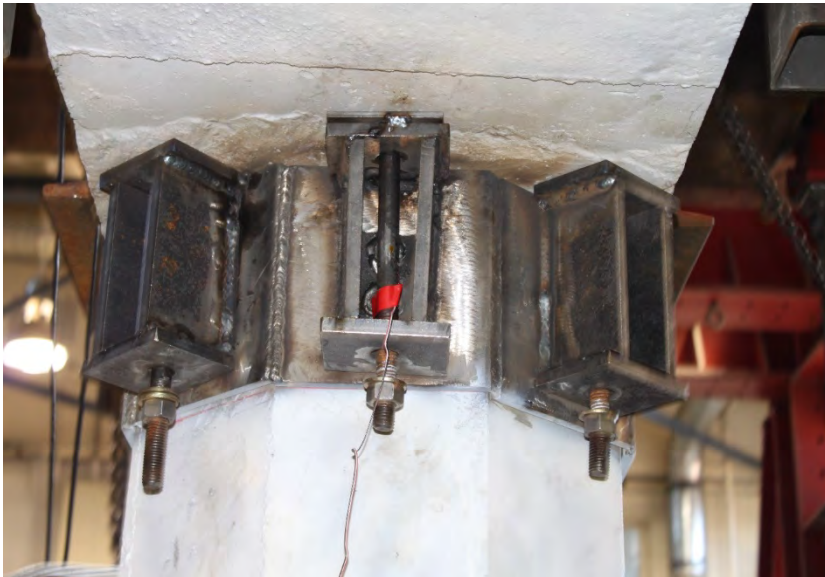
Figure 5.10 Elongation and damage in SLAs
