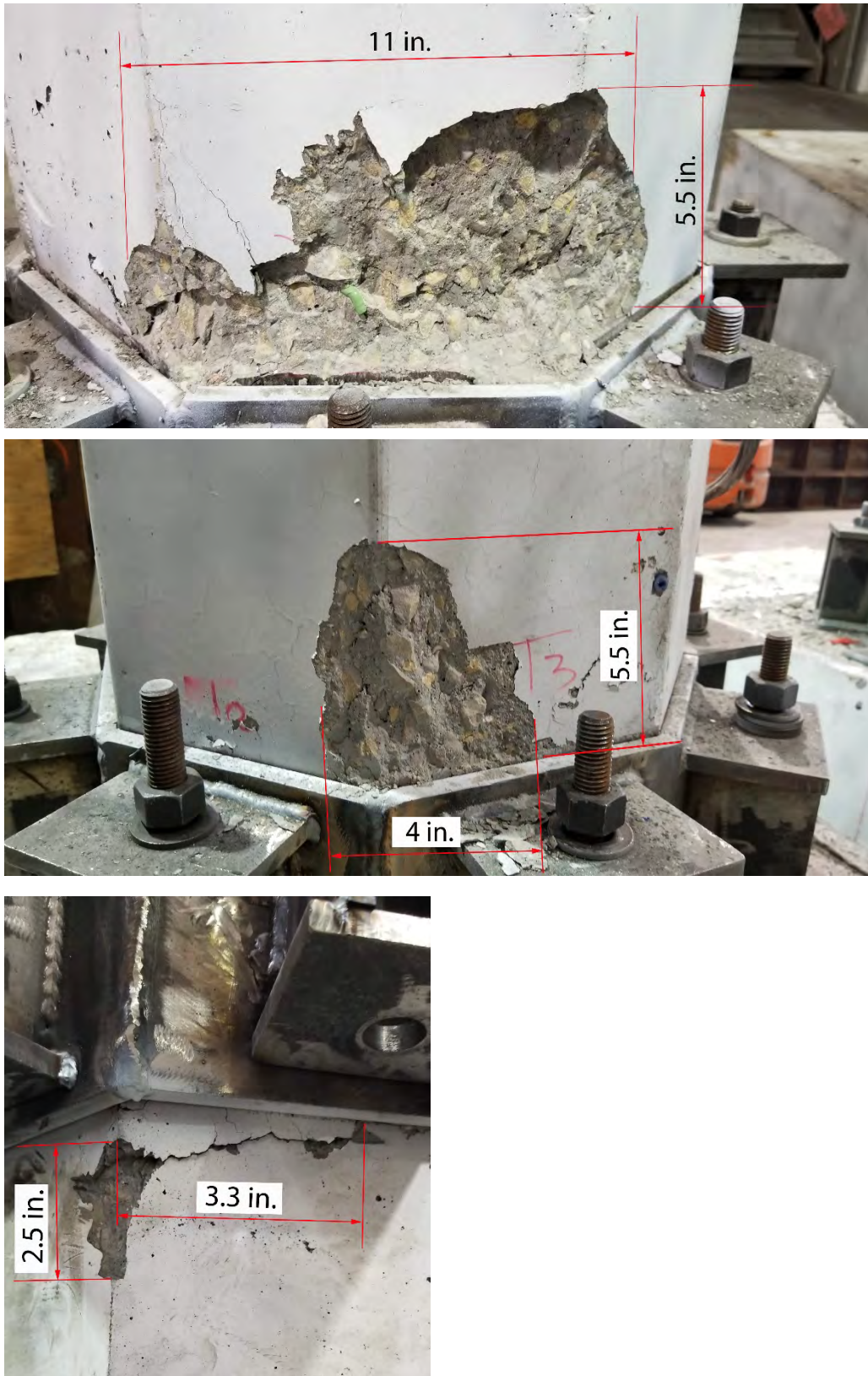
Figure 5.6 Damage in the concrete at the end of the experiment
