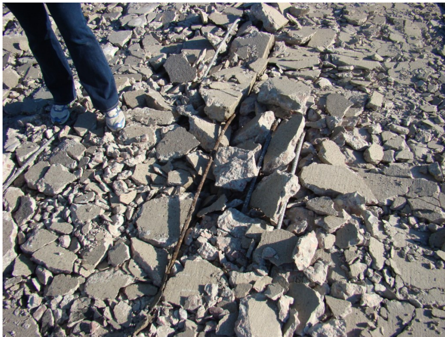
Figure 5.25 Corroded longitudinal reinforcing bar
