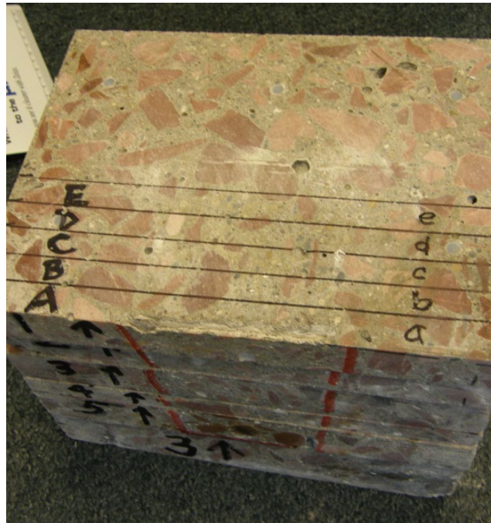
Figure 4.18 Vertical slice scheme for concrete specimen
