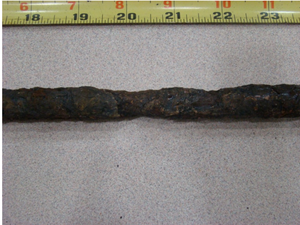
Figure 3.4 Corroded reinforcement removed from degraded CRCP
