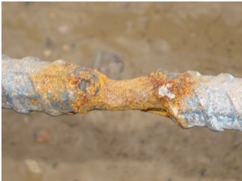
Figure 5.28 Severe loss of cross-sectional area
