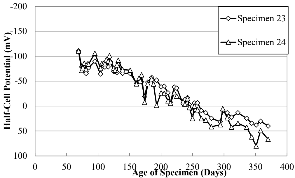
Figure 5.81 Half-cell potential measurements for uncracked, control specimens
