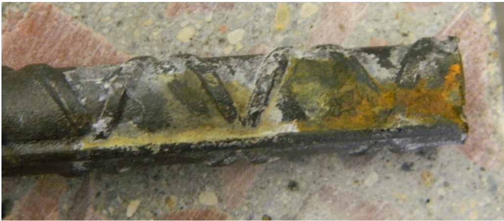
Figure 5.89 Close-up of corrosion of Specimen 16
