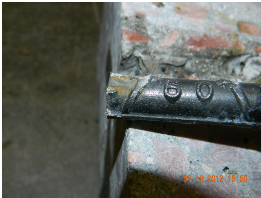
Figure 5.87 Close-up of corrosion of dry, cracked control specimen
