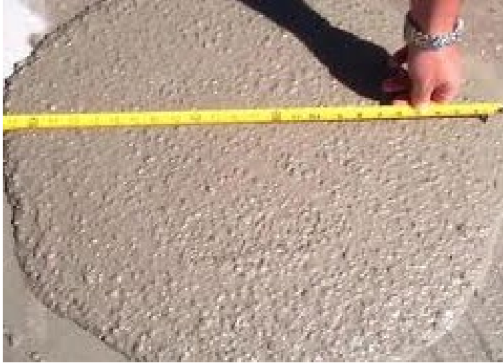
Figure 4.12 Flowability of self-consolidating concrete (SCC) (EAC, 2014)
