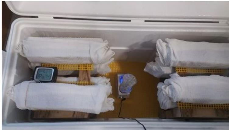
**Figure 4.6** CPT prisms in alternative curing chamber
