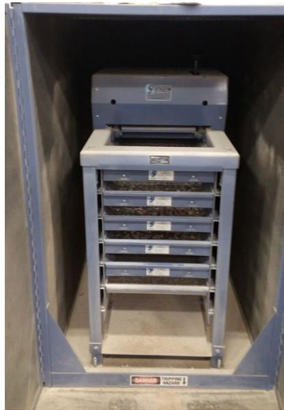
**Figure 3.3** Mechanical screen shaker
