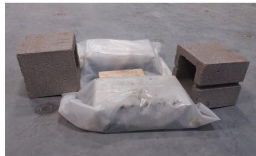
b) Molds wrapped with plastic sheet
