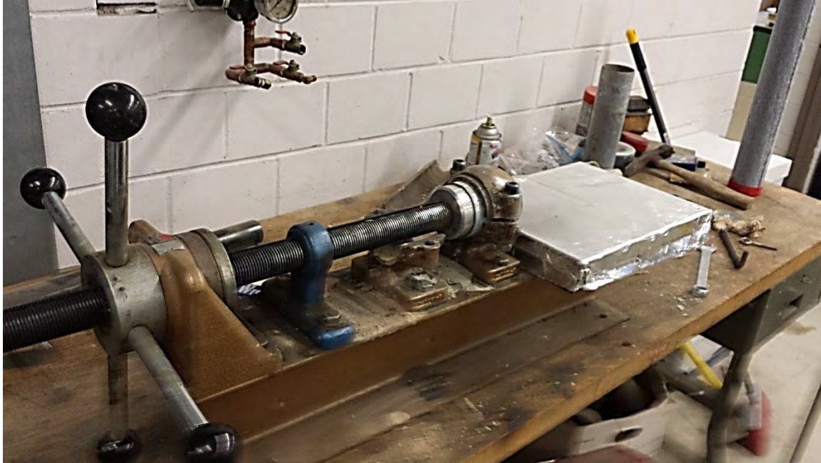
Figure 5.4 Extruding sample from Shelby tube
