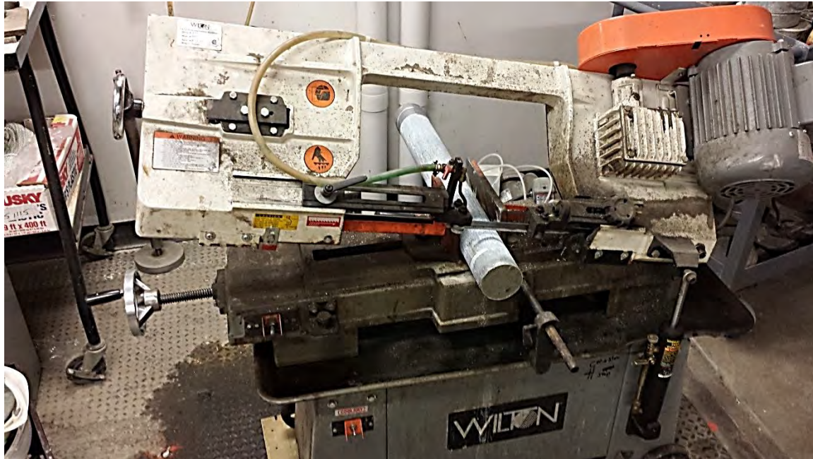
Figure 5.3 Horizontal band saw used to cut samples for testing
