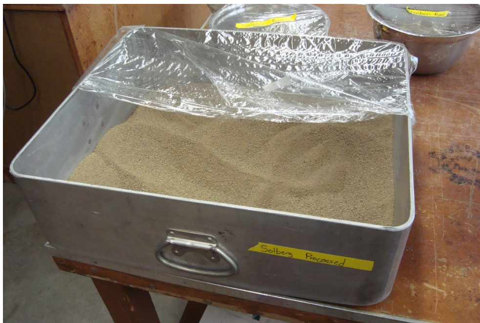
Figure 3.3 A processed soil sample for simulated stormwater runoff creation
