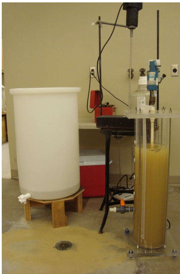
Figure 3.4 The column reactor and holding tank for simulated stormwater runoff
