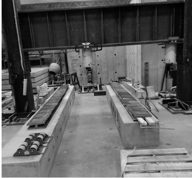
**Figure 4.3.11** Punching shear deck supports
