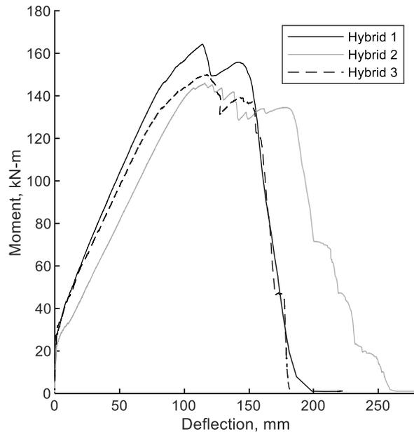
**Figure 5.3.22** Moment-deflection curves for HRC decks (SI)
