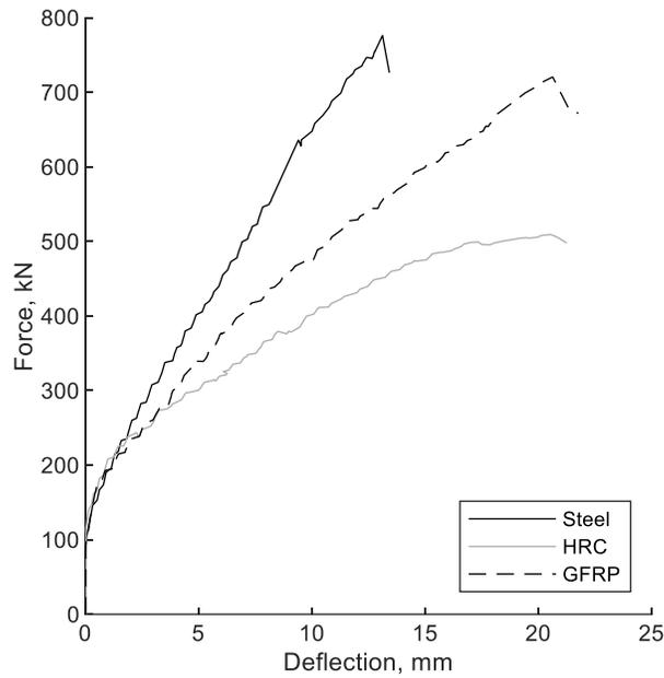
**Figure 6.3.8** Force-deflection curves for punching shear decks (SI)
