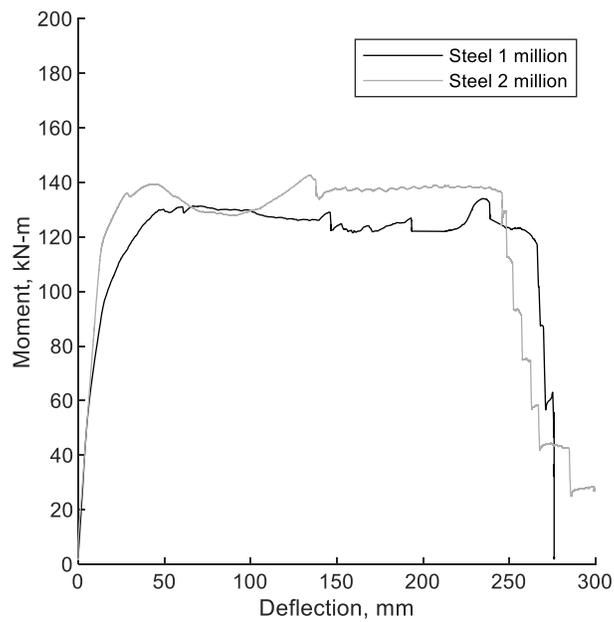
**Figure 5.5.2** Moment-deflection response for post-fatigue steel decks (SI)
