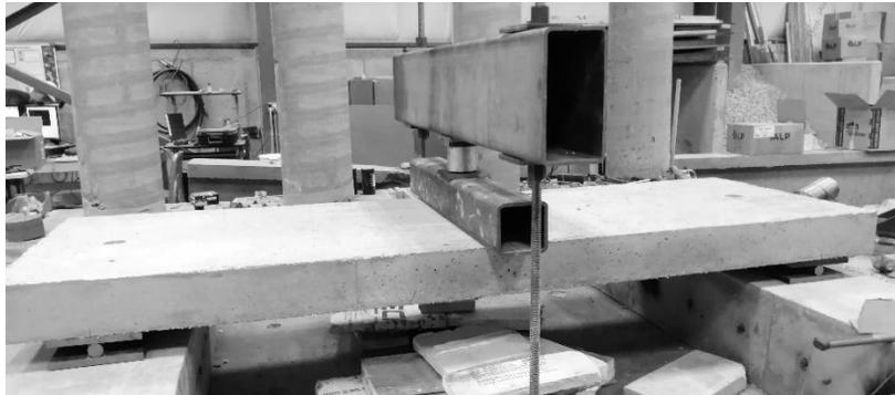
**Figure 3.3.18** Static test after fatigue loading
