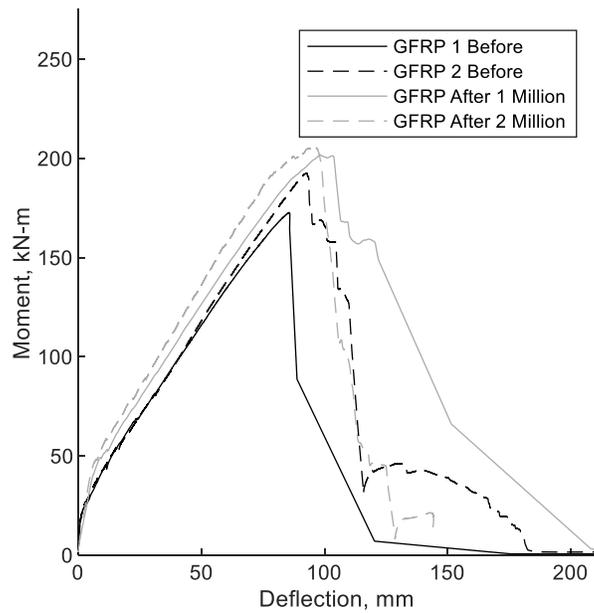
**Figure 5.5.12** Moment-deflection before and after fatigue – GFRP (SI)
