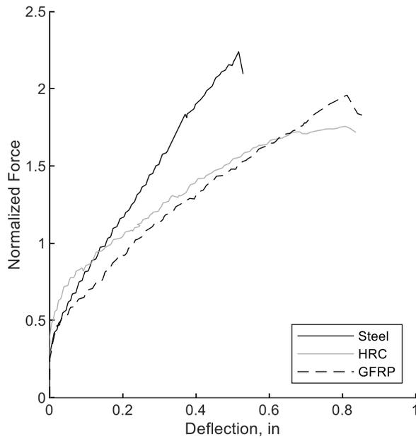
**Figure 8.2.3** Normalized force-deflection of punching shear decks (Imperial)
