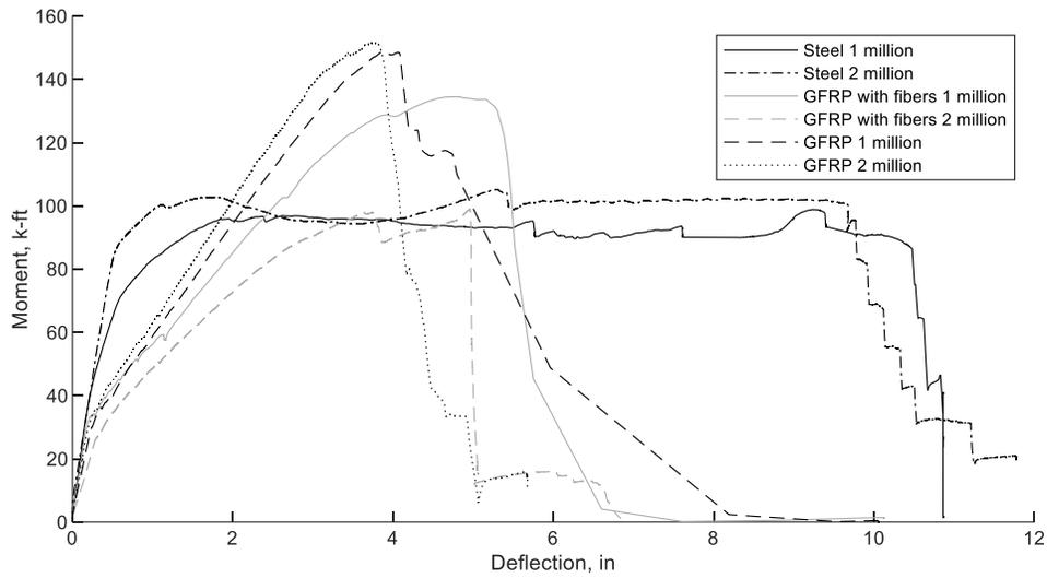
**Figure 5.5.7** Moment-deflection response for post-fatigue decks (Imperial)
