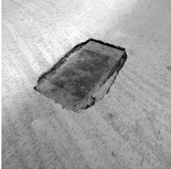
**Figure 8.4.5** Top of steel post-fatigue punching shear deck
