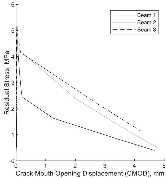
**Figure 6.2.4** Stress-CMOD curve HRC punching shear (SI)
