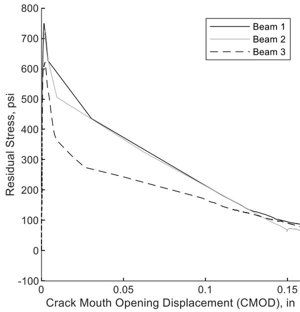
**Figure 5.2.13** Stress-CMOD curve HRC set #2 (Imperial)
