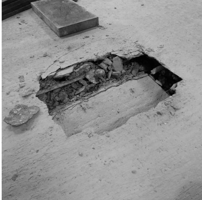
**Figure 8.2.6** Top of GFRP punching shear deck
