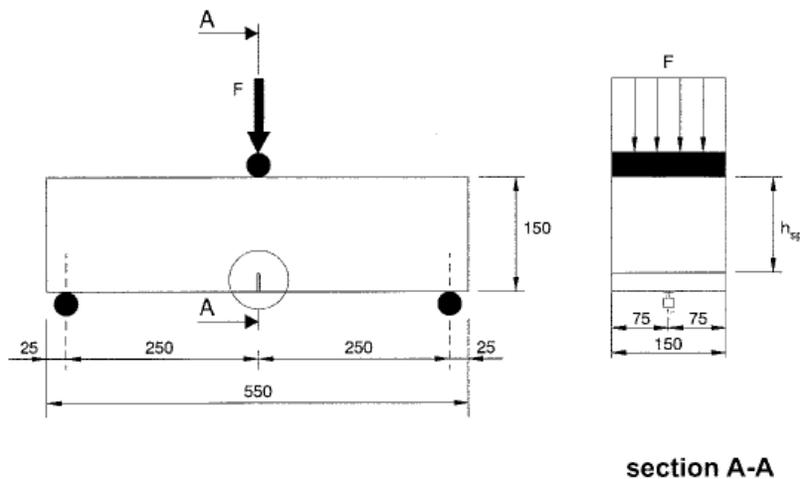
**Figure 2.3.3** EN 14651 beam setup (EN 14651, 2005)
