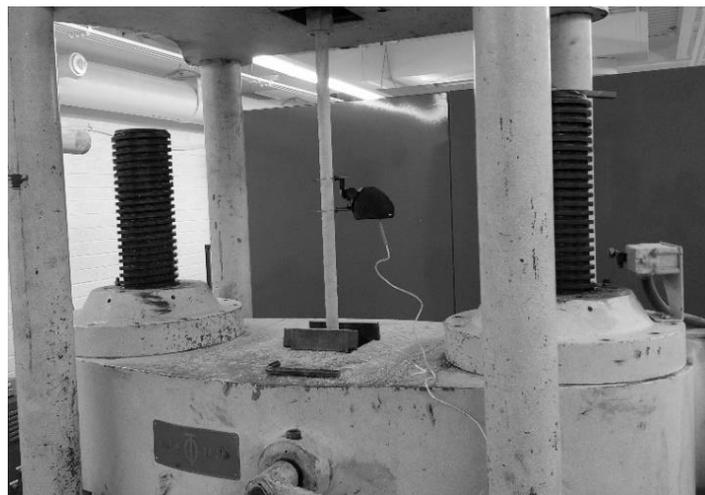
**Figure 3.2.4** GFRP tensile test setup
