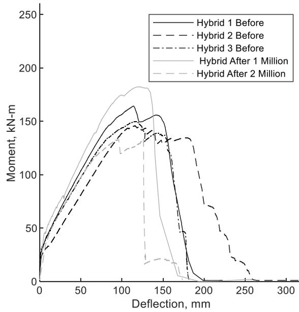
**Figure 5.5.14** Moment-deflection before and after fatigue – HRC (SI)
