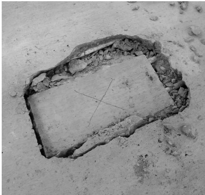
**Figure 8.4.6** Top of GFRP post-fatigue punching shear deck
