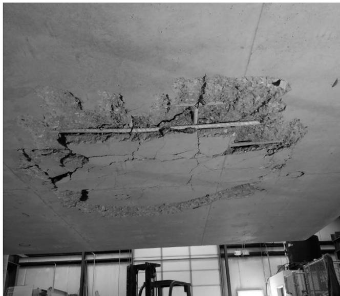
**Figure 8.4.10** Bottom of HRC post-fatigue punching shear deck
