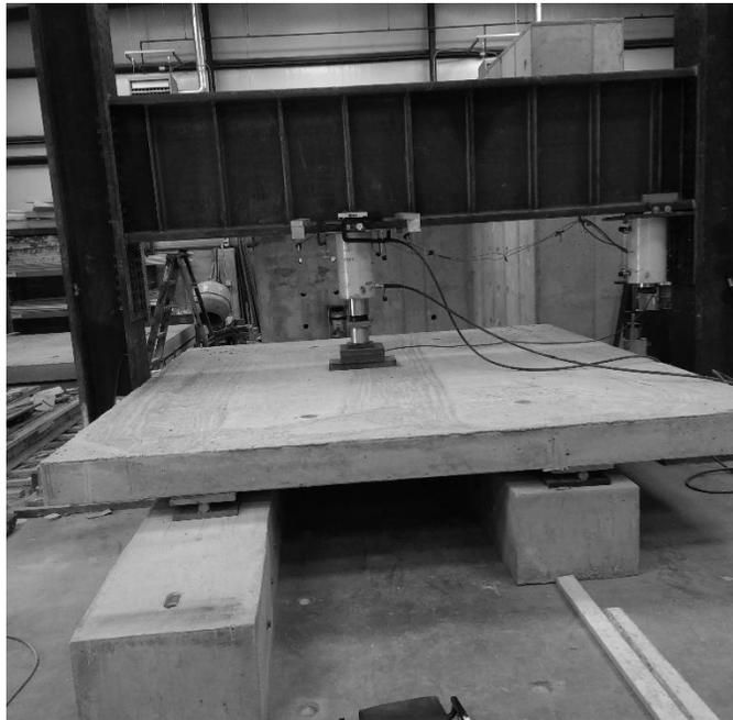
**Figure 4.3.12** Steel punching shear deck static test setup
