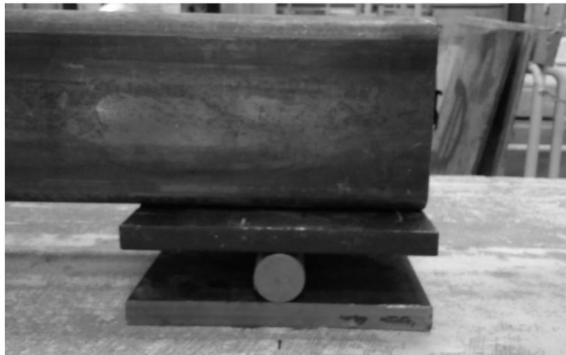
**Figure 3.3.9** Roller support condition (Spreader Beam)
