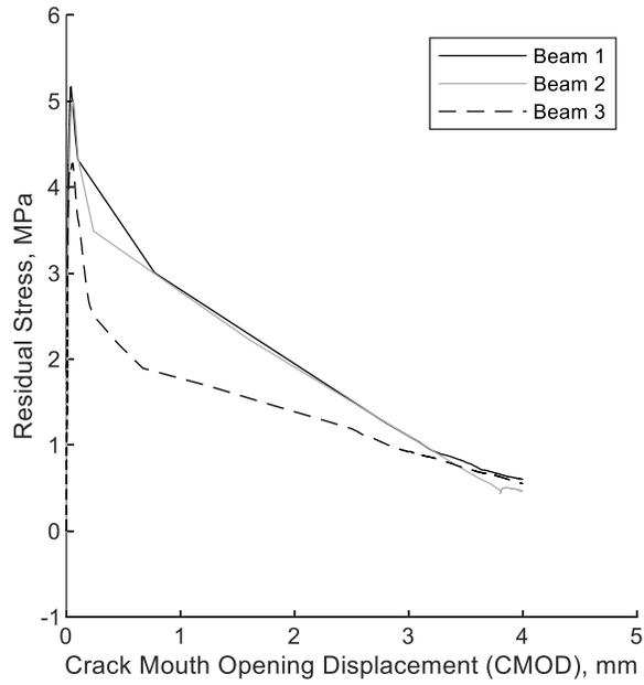
**Figure 5.2.14** Stress-CMOD curve HRC set #2 (SI)
