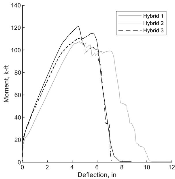
**Figure 5.3.21** Moment-deflection curves for HRC decks (Imperial)
