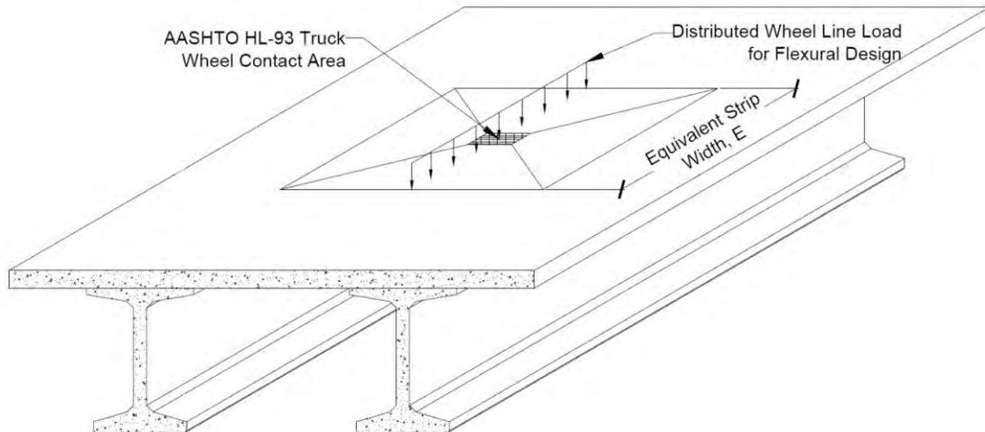
**Figure 3.3.1** Equivalent strip method – wheel load distribution
