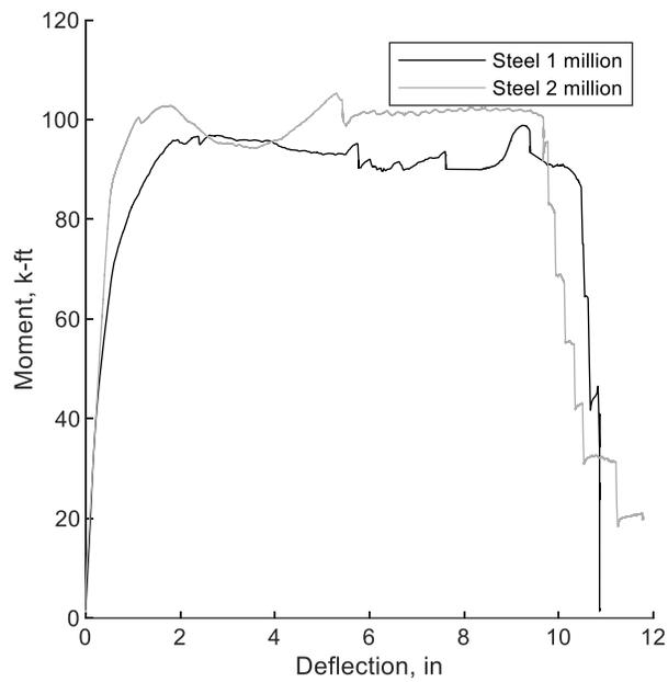
**Figure 5.5.1** Moment-deflection response for post-fatigue steel decks (Imperial)
