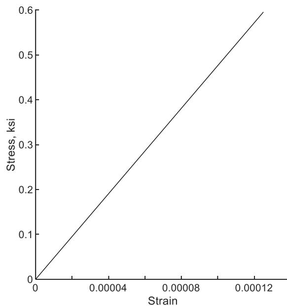
**Figure 7.2.8** Concrete in tension stress-strain constitutive relationship (Imperial)
