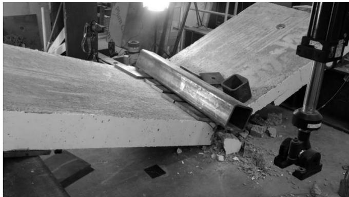
**Figure 7.4.16** GFRP deck at failure
