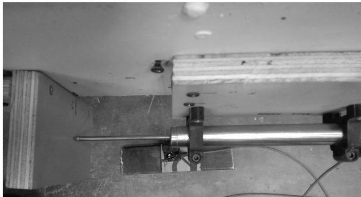
**Figure 3.3.17** LVDT spanning crack at bottom level of deck
