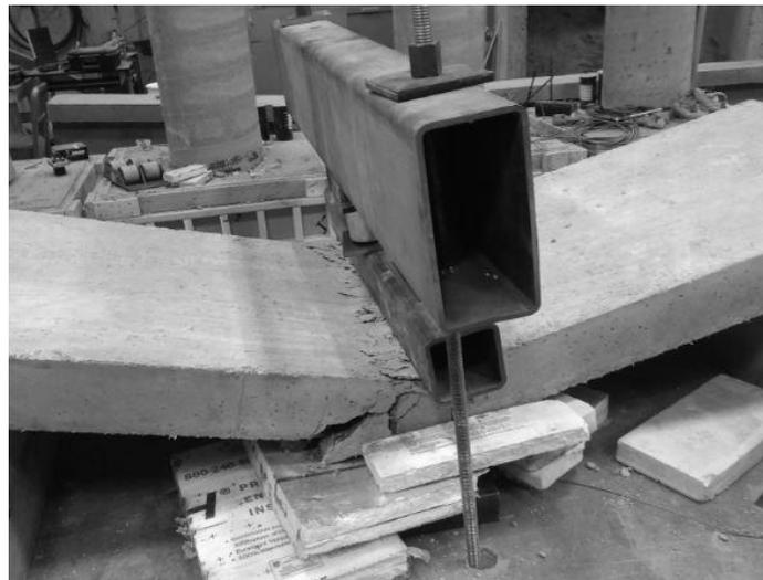
**Figure 7.4.11** HRC failure after 2 million cycles
