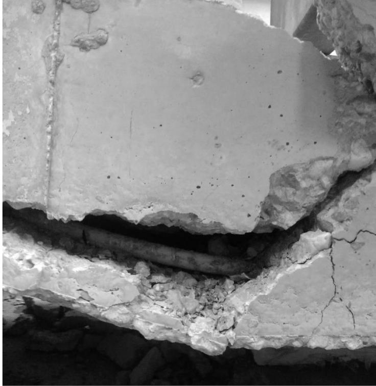
**Figure 7.4.12** Bond failure on GFRP deck post-fatigue
