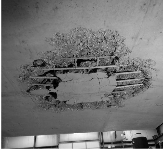
**Figure 8.4.9** Bottom of GFRP post-fatigue punching shear deck
