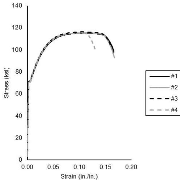
**Figure 5.2.1** Stress-strain curve for steel rebar (Imperial)
