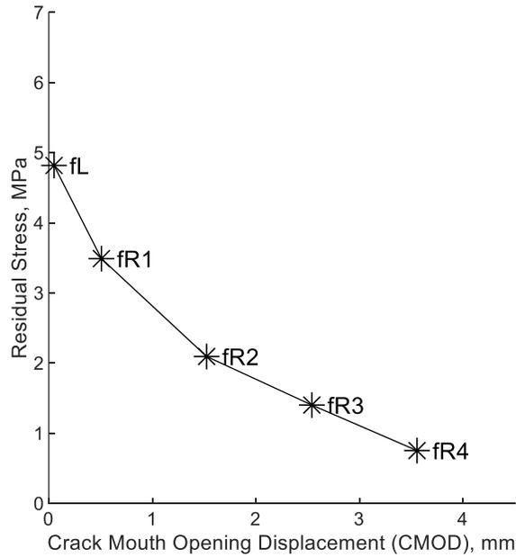
**Figure 5.2.16** Average flexural tensile strength HRC Set #2 (SI)
