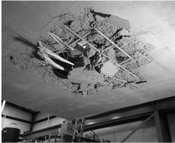
**Figure 8.2.11** Bottom surface of HRC punching shear deck
