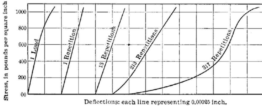
**Figure 2.4.1** Stiffness degradation under cyclic compression, (Van Ornum, 1903)
