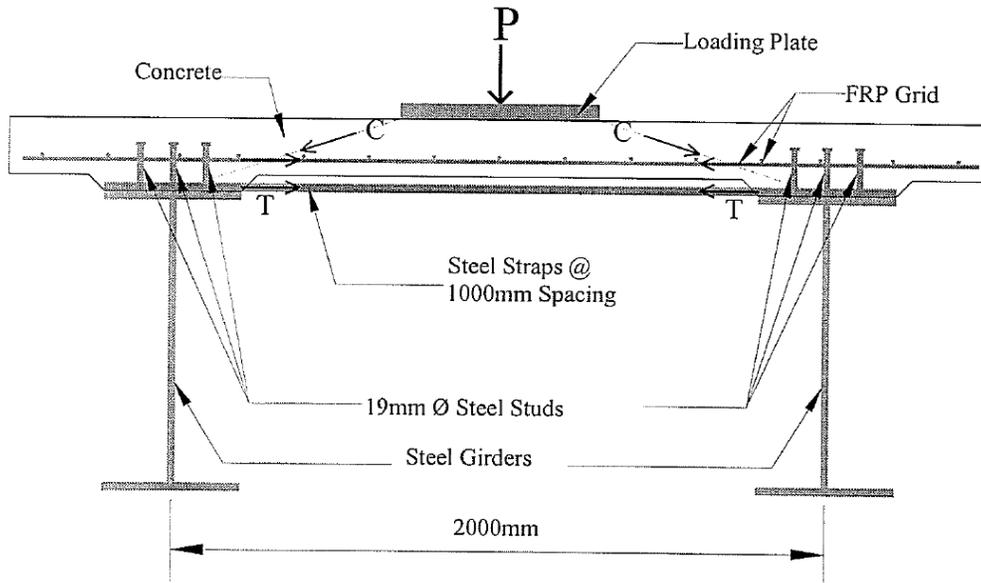
**Figure 2.1.2** Second-generation steel-free bridge decks (Memon, 2005)
