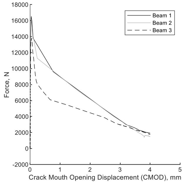
**Figure 5.2.12** Force-CMOD curve HRC set #2 (SI)
