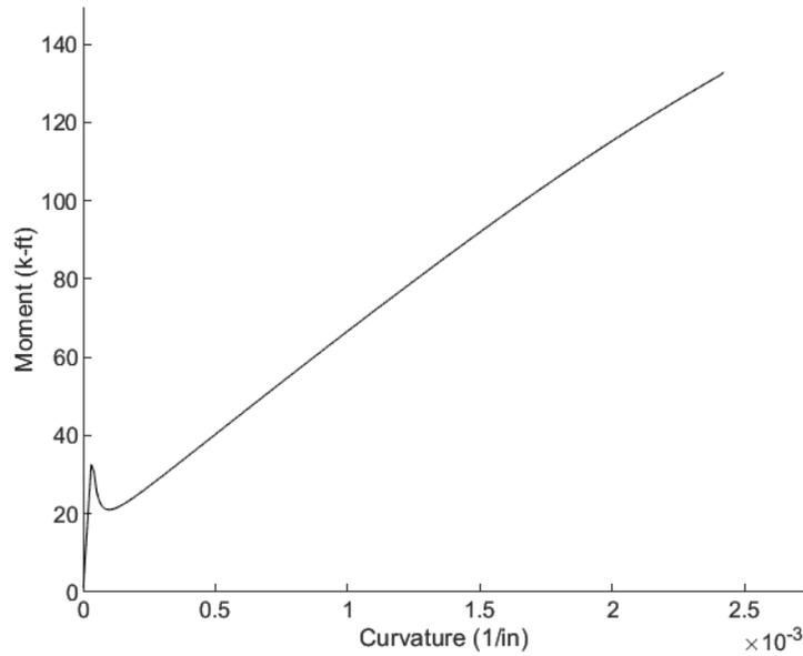
**Figure 7.4.8** HRC set #1 moment-curvature relationship after fatigue
