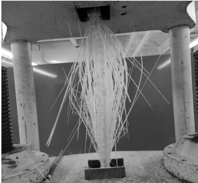
**Figure 3.2.6** Fully ruptured GFRP specimen
