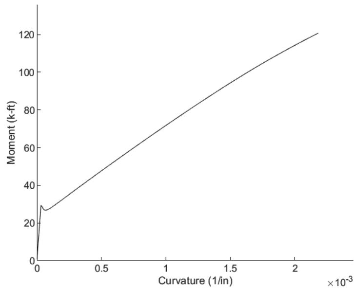
**Figure 7.4.5** HRC set #2 moment-curvature relationship before fatigue
