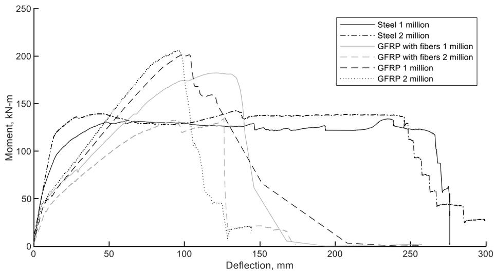
**Figure 5.5.8** Moment-deflection response for post-fatigue decks (SI)
