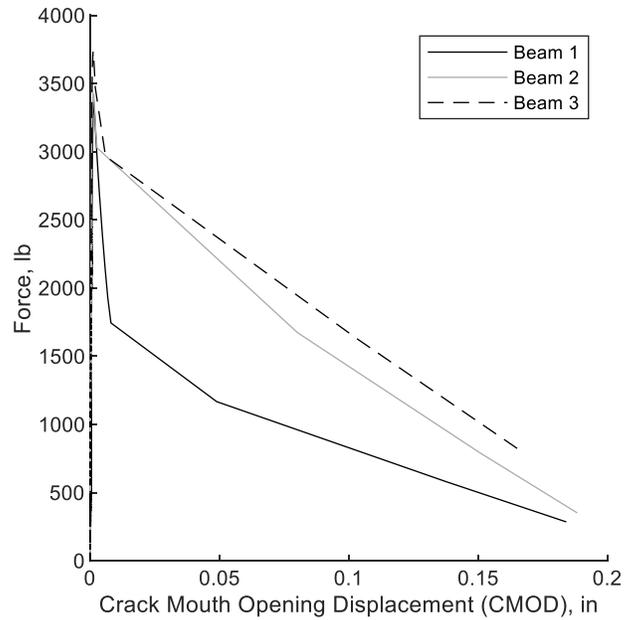
**Figure 6.2.1** Force-CMOD curve HRC punching shear (Imperial)
