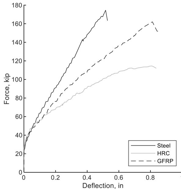
**Figure 6.3.7** Force-deflection curves for punching shear decks (Imperial)
