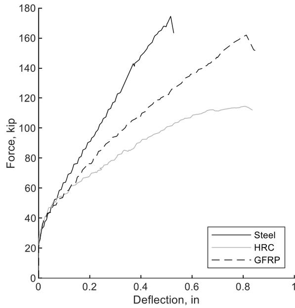
**Figure 8.2.1** Force-deflection of punching shear decks (Imperial)
