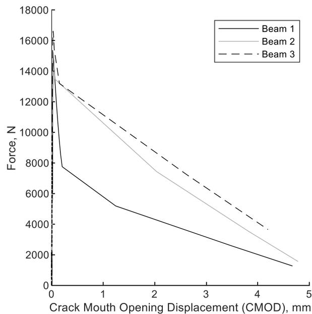
**Figure 6.2.2** Force-CMOD curve HRC punching shear (SI)
