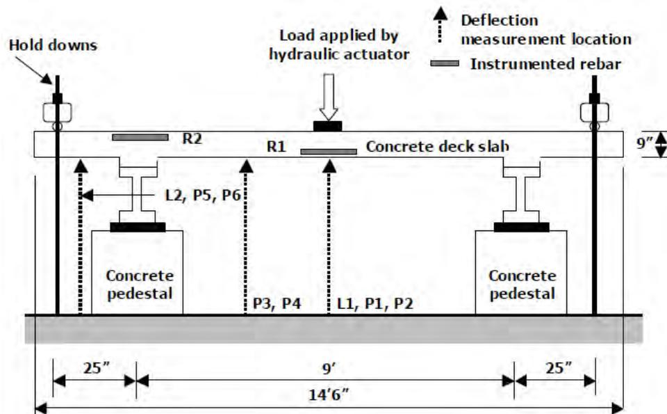
Figure 2.4.6 Static and fatigue setup, (Gopalaratnam et al., 2006)
