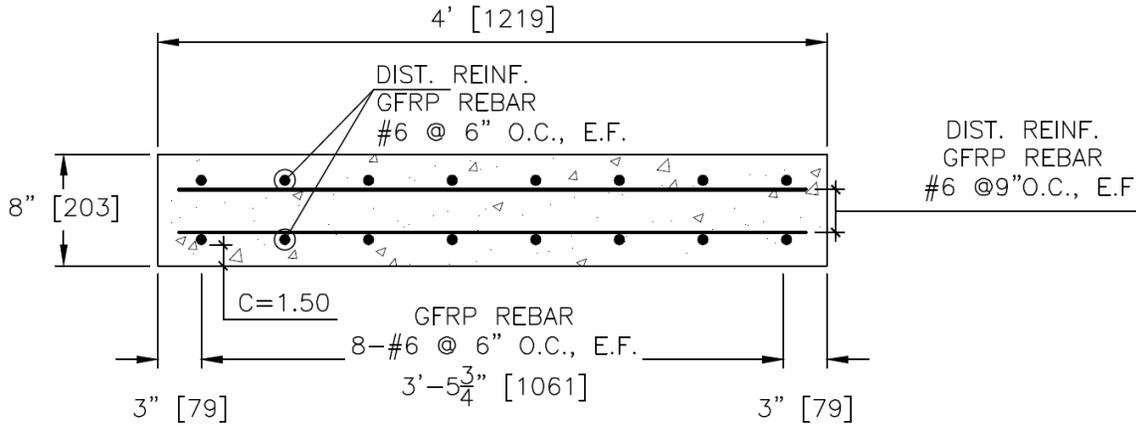
**Figure 3.3.3** GFRP reinforcement layout
