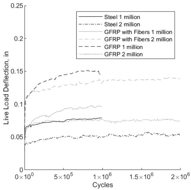
**Figure 7.3.2** Live load deflection – fatigue loading
