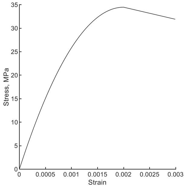
**Figure 7.2.7** Concrete compressive stress-strain constitutive relationship (SI)
