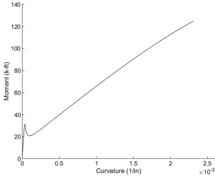
**Figure 7.4.4** HRC set #1 moment-curvature relationship before fatigue
