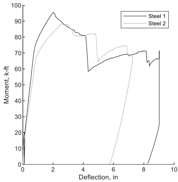
**Figure 5.3.17** Moment-deflection curves for steel-reinforced decks (Imperial)
