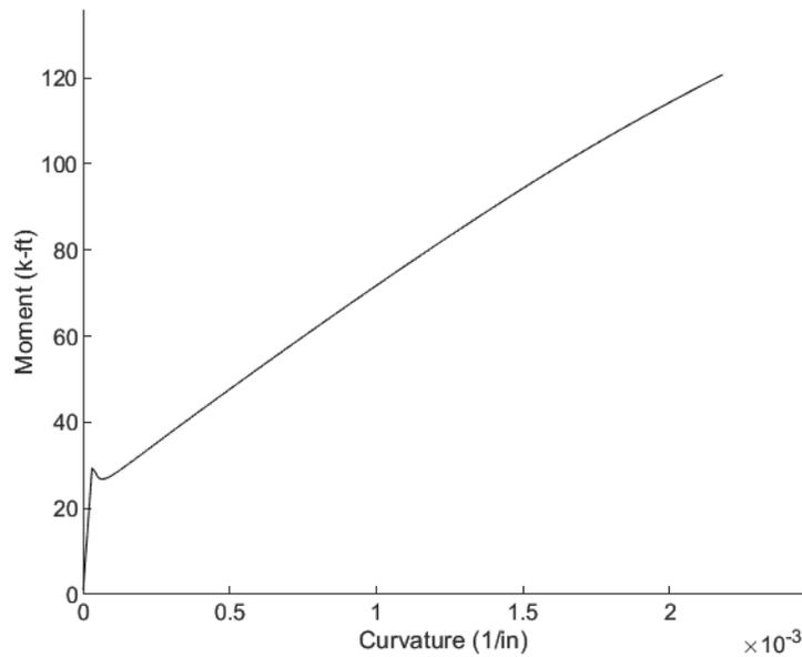
**Figure 7.4.9** HRC set #2 moment-curvature relationship after fatigue
