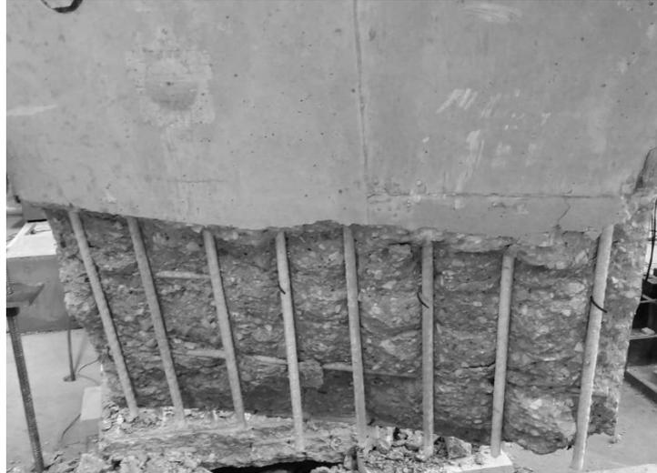
**Figure 7.4.14** Bottom view of GFRP specimen after failure
