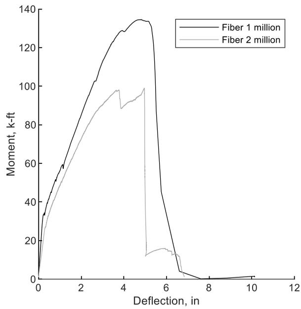
**Figure 5.5.3** Moment-deflection response for post-fatigue HRC decks (Imperial)
