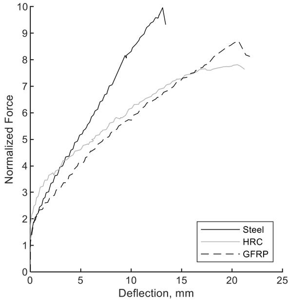
**Figure 8.2.4** Normalized force-deflection of punching shear decks (SI)
