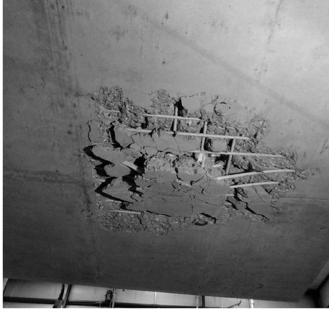
**Figure 8.2.10** Bottom surface of GFRP punching shear deck
