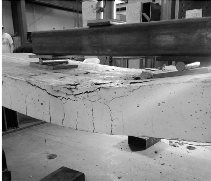
**Figure 7.4.15** Steel deck at failure
