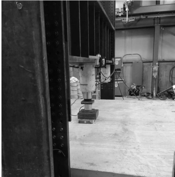
**Figure 4.3.14** HRC punching shear static test setup
