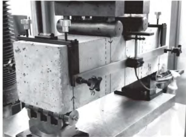
**Figure 2.3.2** ASTM C1609 test setup (ACI Committee 544, 2018)
