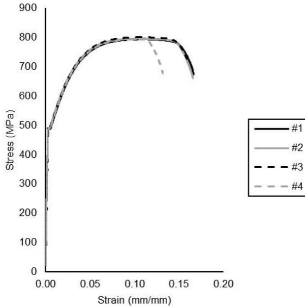
**Figure 5.2.2** Stress-strain curve for steel rebar (SI)
