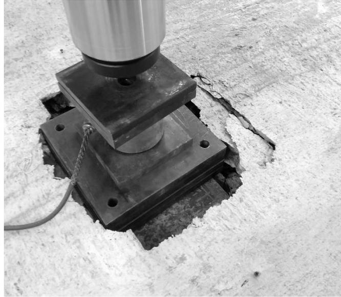
**Figure 8.2.5** Top of steel punching shear deck
