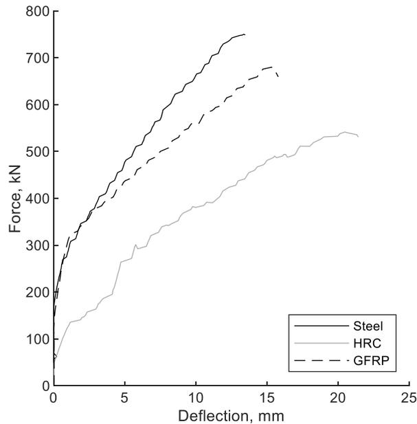
**Figure 6.5.2** Force-deflection for post-fatigue punching shear decks (SI)
