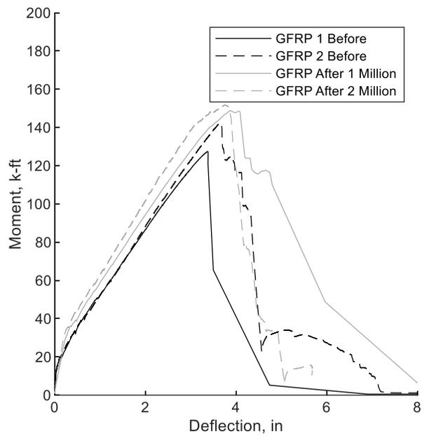
**Figure 5.5.11** Moment-deflection before and after fatigue – GFRP (Imperial)
