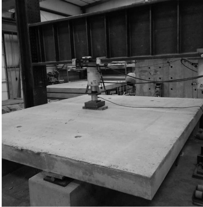
**Figure 4.3.13** GFRP punching shear static test setup
