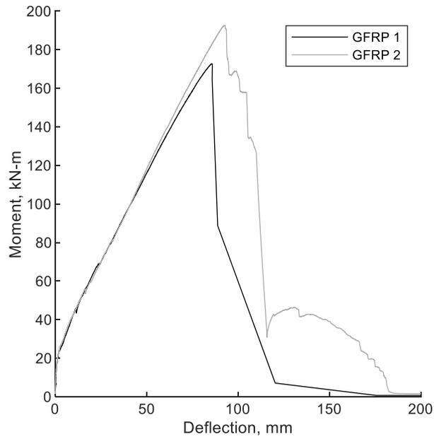
**Figure 5.3.20** Moment-deflection curves for GFRP-reinforced decks (SI)
