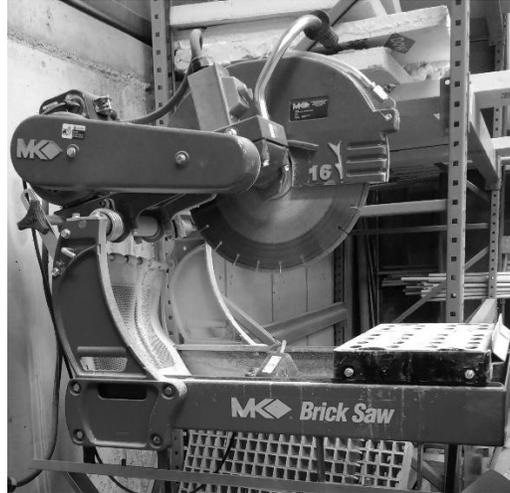
**Figure 3.2.4** Saw used to notch FRC specimens
