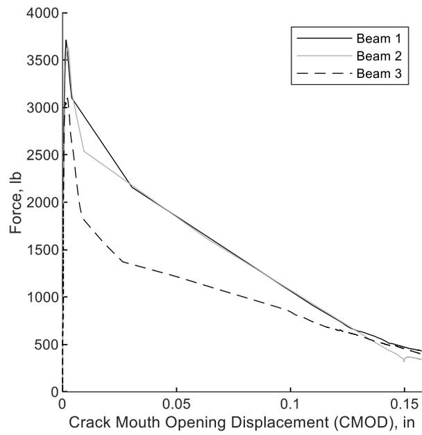
**Figure 5.2.11** Force-CMOD curve HRC set #2 (Imperial)
