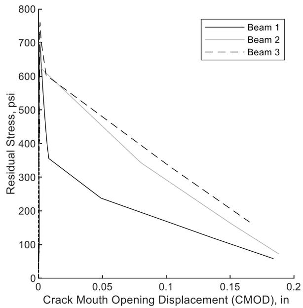
**Figure 6.2.3** Stress-CMOD curve HRC punching shear (Imperial)
