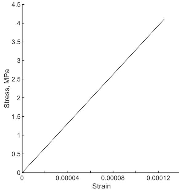
**Figure 7.2.9** Concrete in tension stress-strain constitutive relationship (SI)
