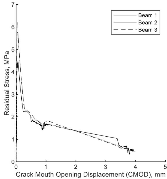
**Figure 5.2.8** Stress-CMOD curve HRC Set #1 (SI)
