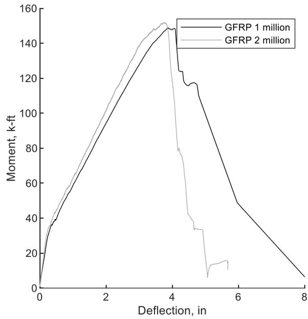
**Figure 5.5.5** Moment-deflection response for post-fatigue GFRP decks (Imperial)
