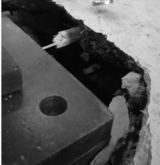
**Figure 8.2.8** Shear rupture of GFRP bar
