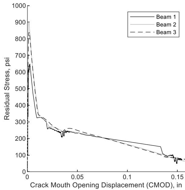
**Figure 5.2.7** Stress-CMOD curve HRC set #1 (Imperial)
