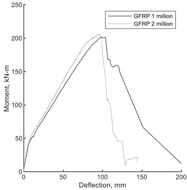
**Figure 5.5.6** Moment-deflection response for post-fatigue GFRP decks (SI)
