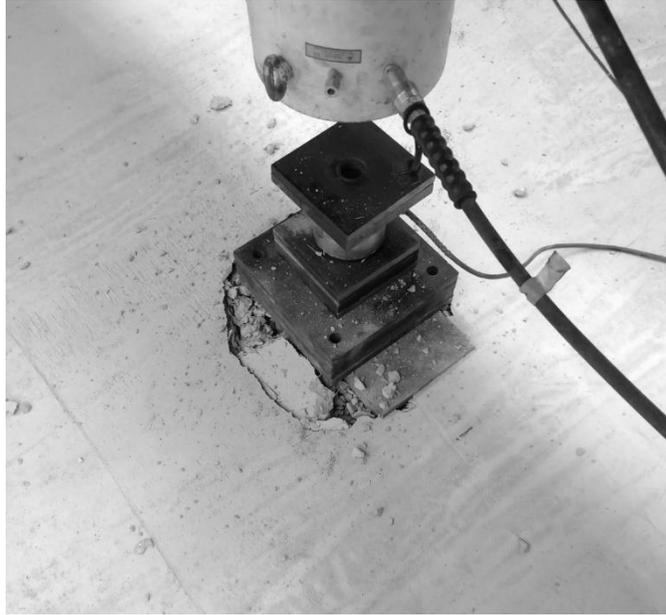
**Figure 8.4.7** Top of HRC post-fatigue punching shear deck
