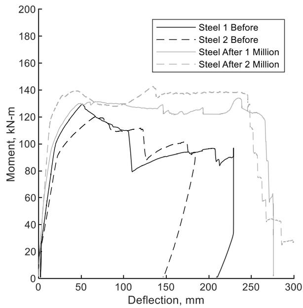
**Figure 5.5.10** Moment-deflection before and after fatigue – steel (SI)
