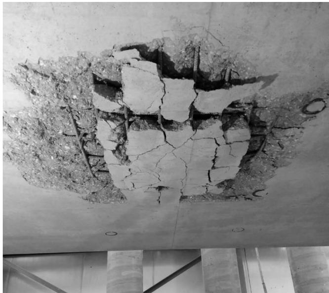
**Figure 8.4.8** Bottom of steel post-fatigue punching shear deck
