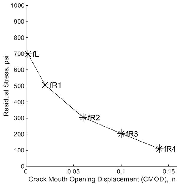
**Figure 5.2.15** Average flexural tensile strength HRC set #2 (Imperial)
