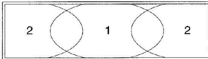
**Figure 3.2.2** Specified pattern to fill up molds (EN 14651, 2005)
