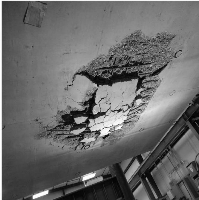
**Figure 8.2.9** Bottom surface of steel punching shear deck
