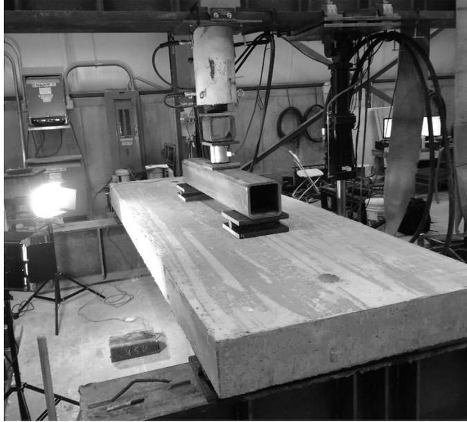
**Figure 3.3.12** Static test setup (steel-reinforced deck)
