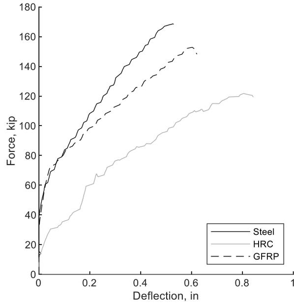
**Figure 6.5.1** Force-deflection for post-fatigue punching shear decks (Imperial)
