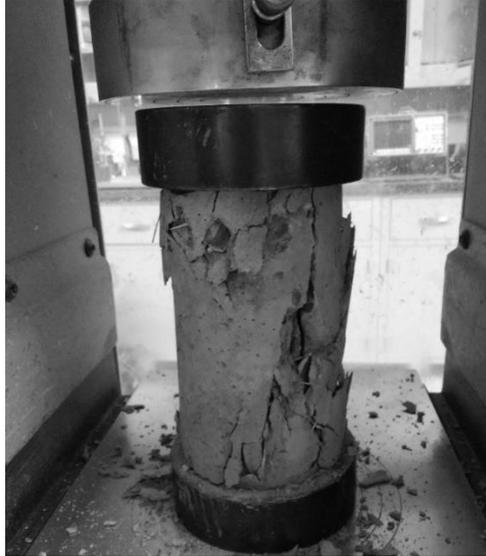
**Figure 3.2.9** Compression test of an FRC cylinder
