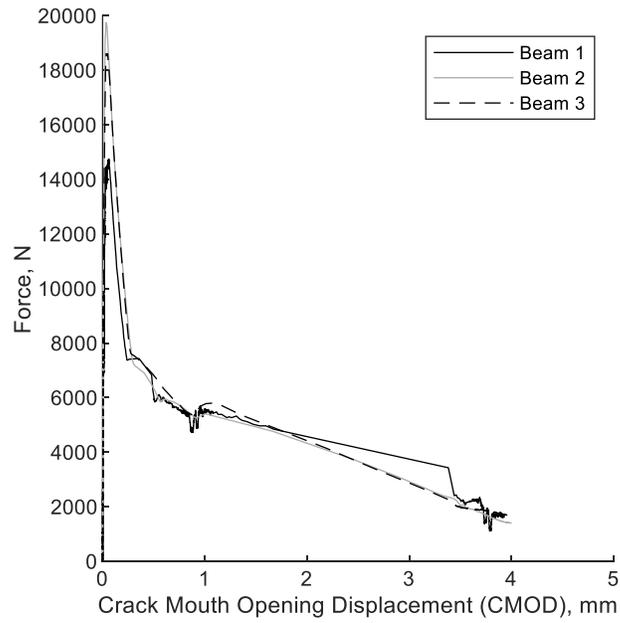
**Figure 5.2.6** Force-CMOD curve HRC set #2 (SI)
