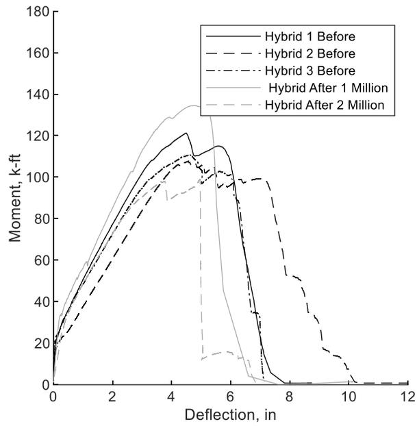
**Figure 5.5.13** Moment-deflection before and after fatigue – HRC (Imperial)
