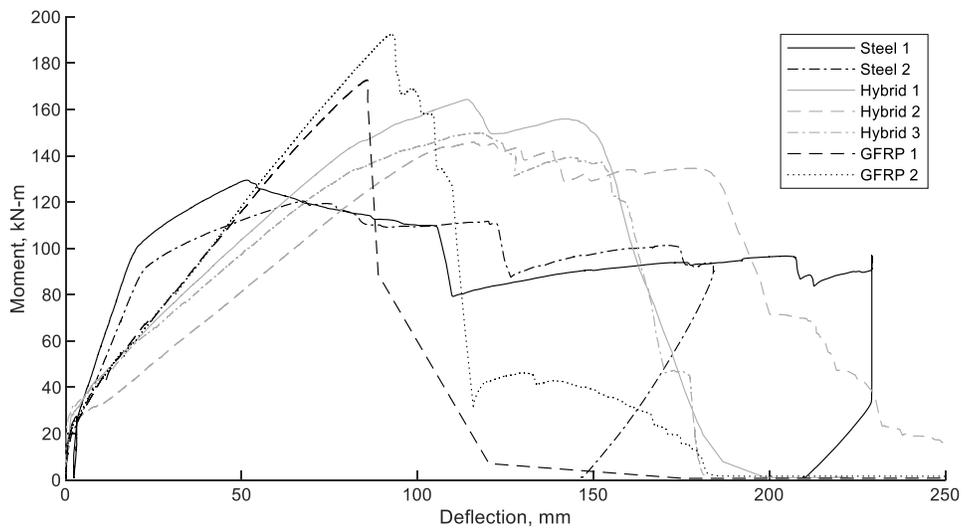
**Figure 5.3.24** Moment-deflection curves for all bridge decks (SI)
