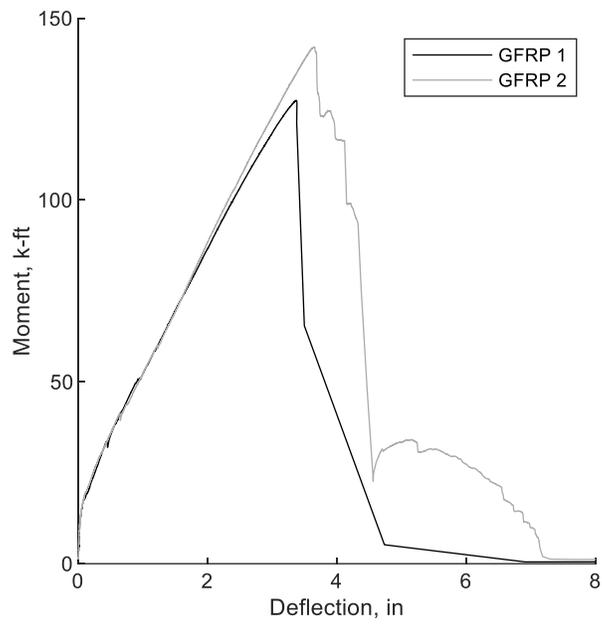
**Figure 5.3.19** Moment-deflection curves for GFRP-reinforced decks (Imperial)
