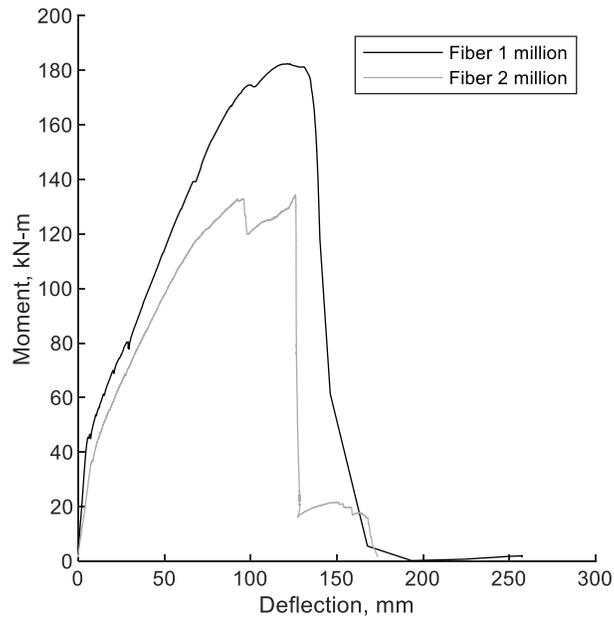
**Figure 5.5.4** Moment-deflection response for post-fatigue HRC decks (SI)
