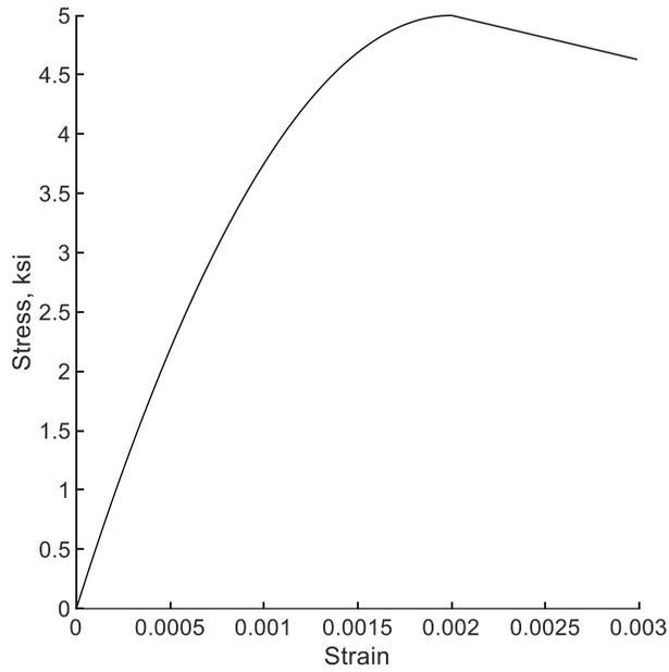
**Figure 7.2.6** Concrete compressive stress-strain constitutive relationship (Imperial)
