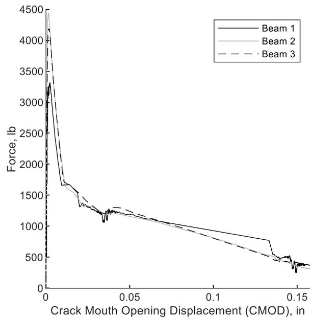
**Figure 5.2.5** Force-CMOD curve HRC set #1 (Imperial)
