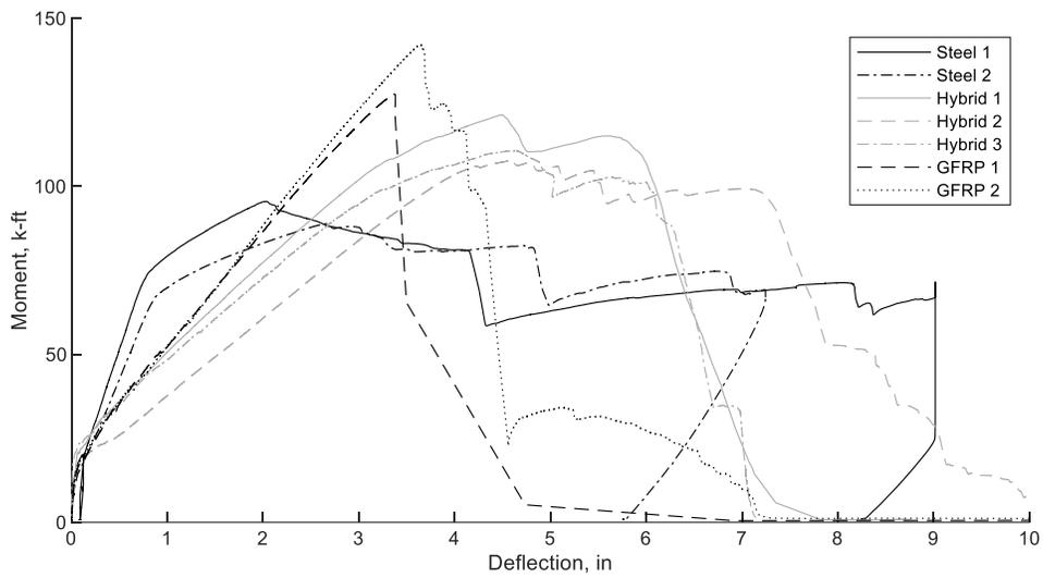
**Figure 5.3.23** Moment-deflection curves for all bridge decks (Imperial)
