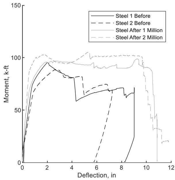
**Figure 5.5.9** Moment-deflection before and after fatigue – steel (Imperial)
