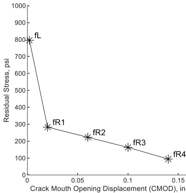
**Figure 5.2.9** Average flexural tensile strength HRC set #1 (Imperial)
