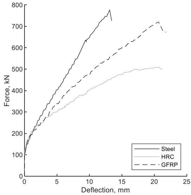
**Figure 8.2.2** Force-deflection of punching shear decks (SI)
