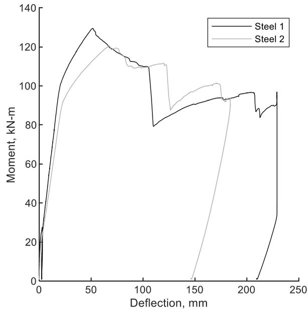
**Figure 5.3.18** Moment-deflection curves for steel-reinforced decks (SI)
