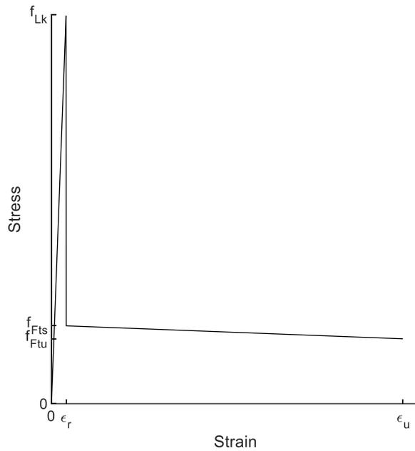
**Figure 7.2.10** FRC in tension stress strain constitutive relationship
