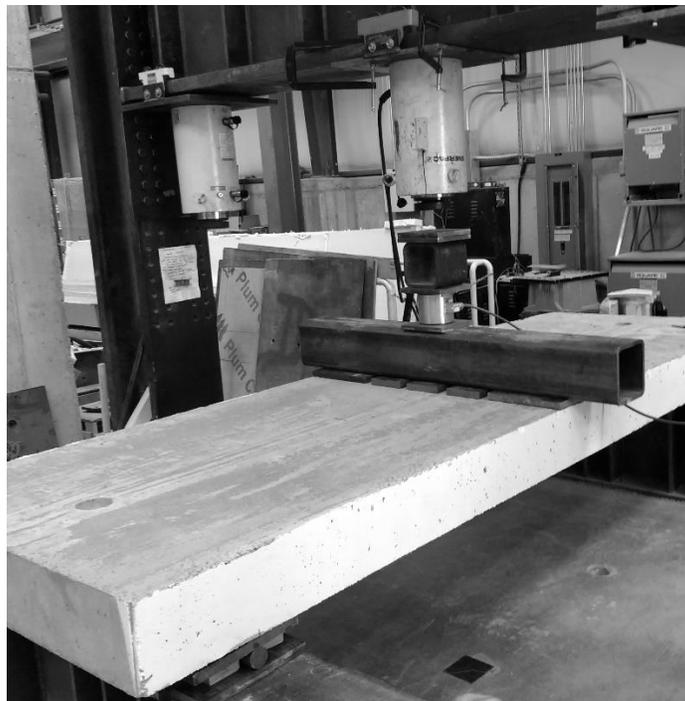
**Figure 3.3.13** Static test with centerline loading (GFRP deck)
