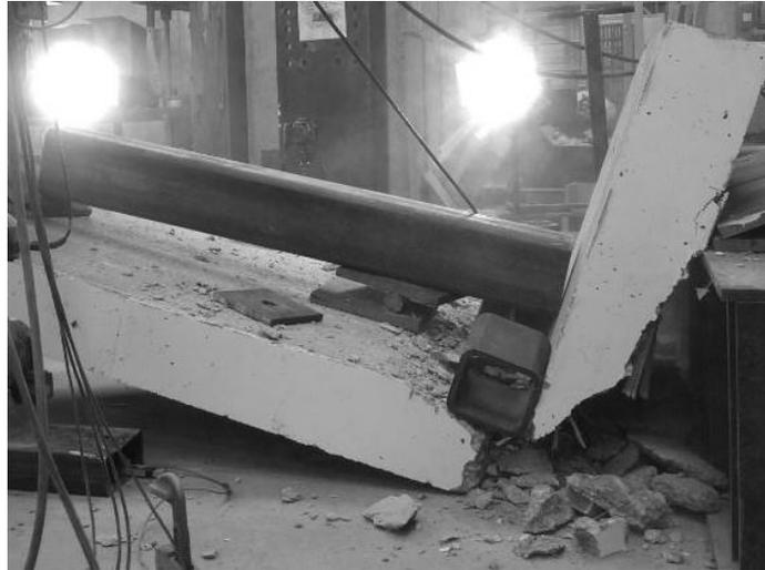
**Figure 7.4.10** Shear failure on first GFRP specimen
