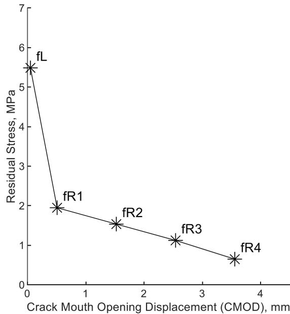
**Figure 5.2.10** Average flexural tensile strength HRC set #1 (SI)
