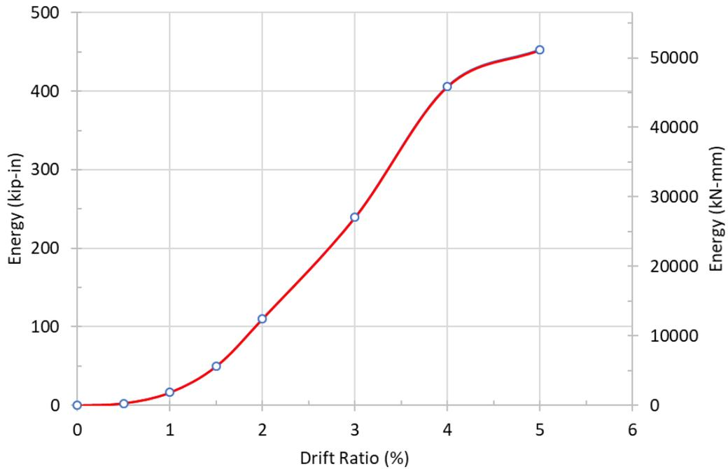
**Figure 7.8** Cumulative hysteretic energy dissipation of specimen ABRP
