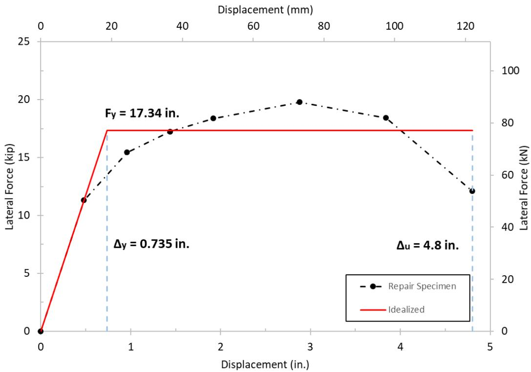
**Figure 7.6** Displacement ductility plot of repaired specimen ABRP
