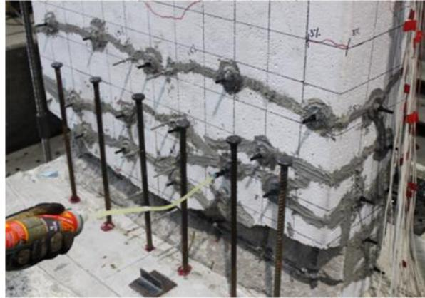
**Figure 8.5** Epoxy injection of cracks for specimen MCRP
