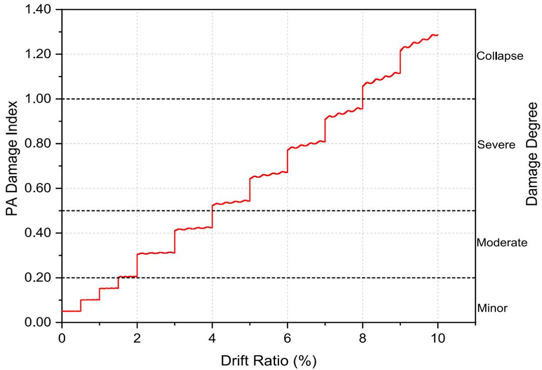
**Figure 4.7** Damage index of modern code compliant specimen
