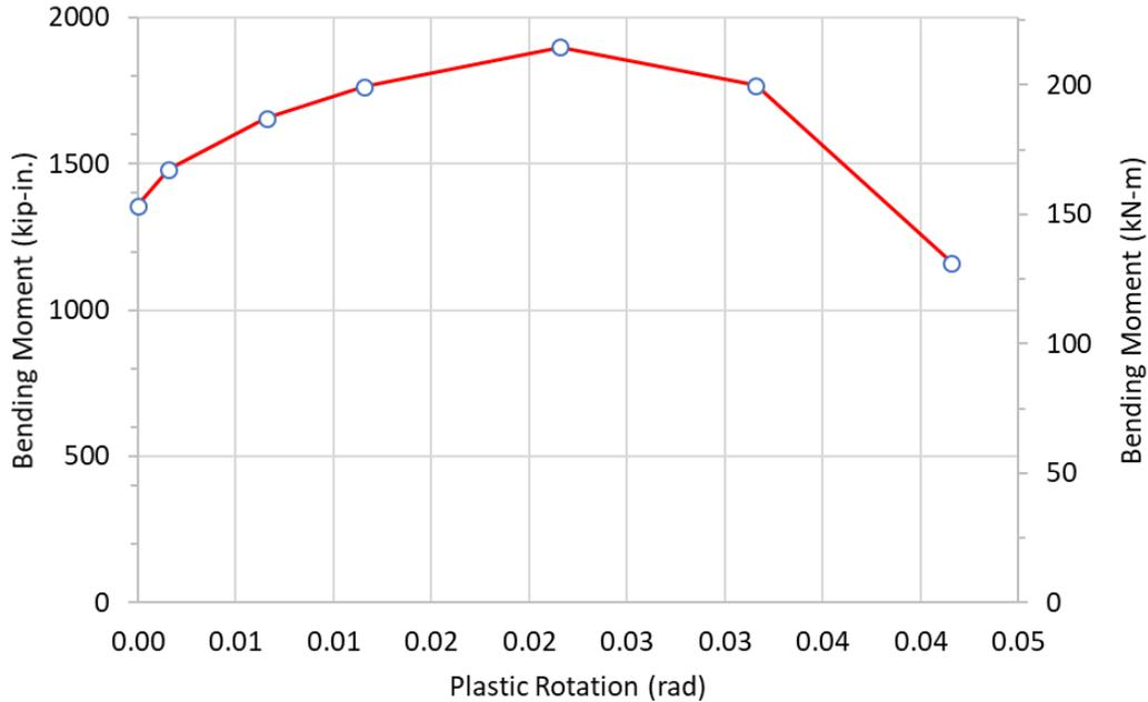
Figure 7.7 Plastic rotation plot of repaired specimen ABRP
