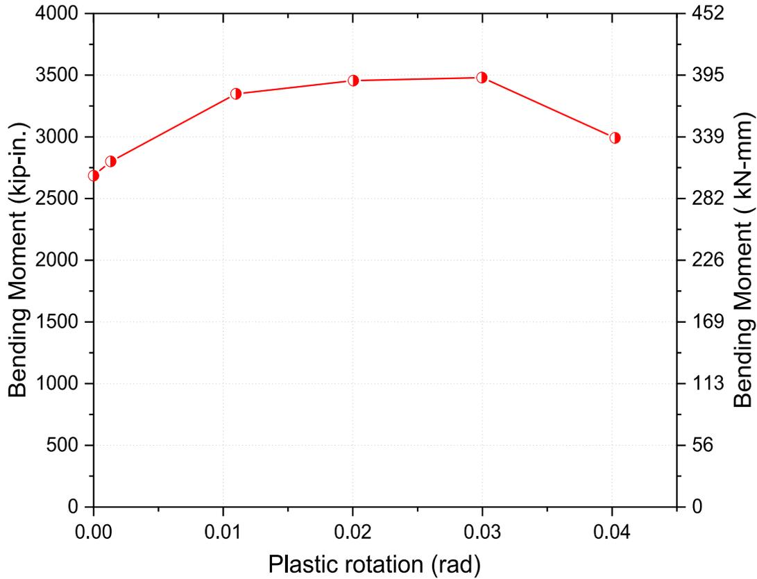
**Figure 8.9** Plastic rotation plot of repaired specimen MCRP
