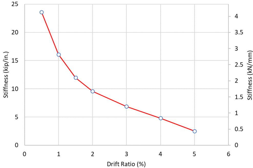
**Figure 7.9** Stiffness deterioration of the repaired specimen ABRP
