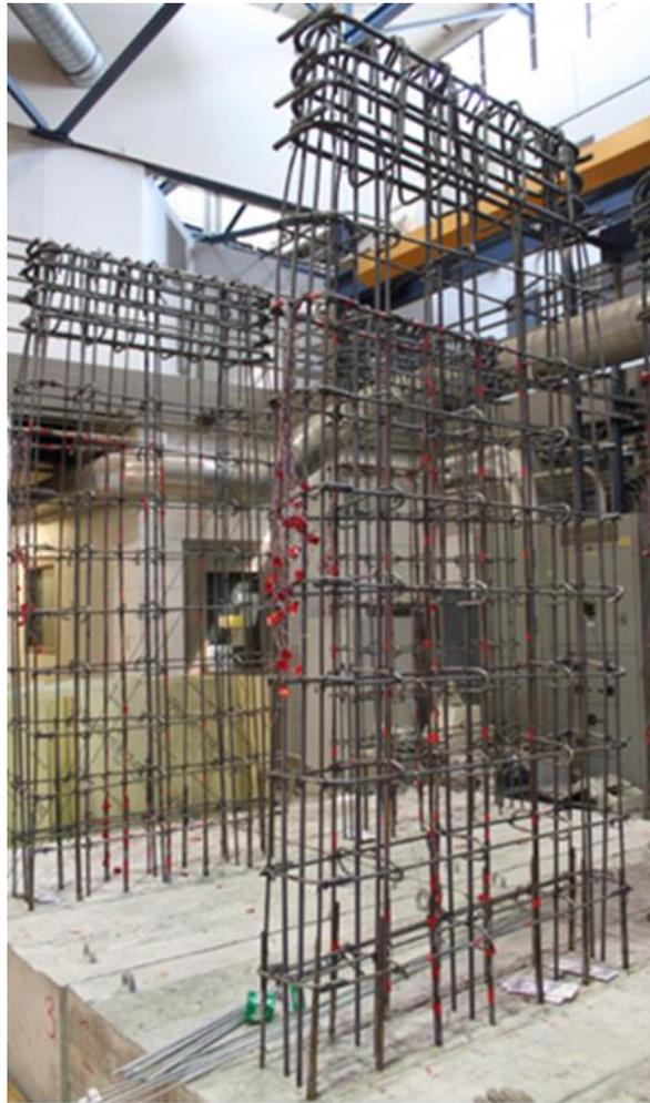
**Figure 2.6** As-built wall pier reinforcement
