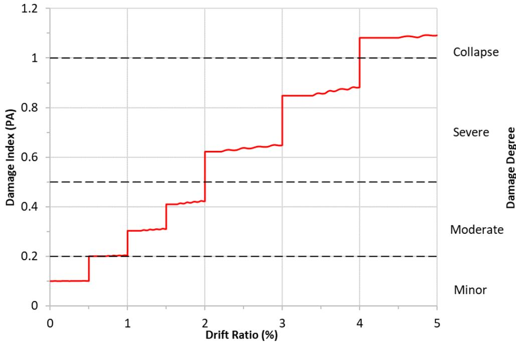
**Figure 7.10** Damage Index of repaired Specimen ABRP
