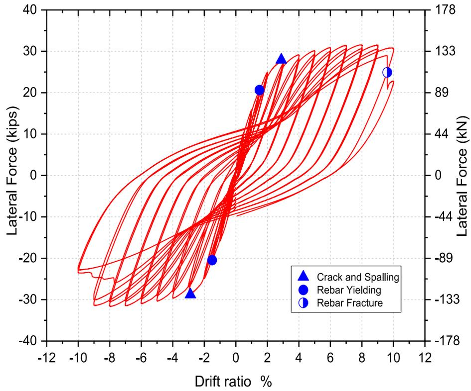
**Figure 4.4** Hysteresis of modern code compliant specimen
