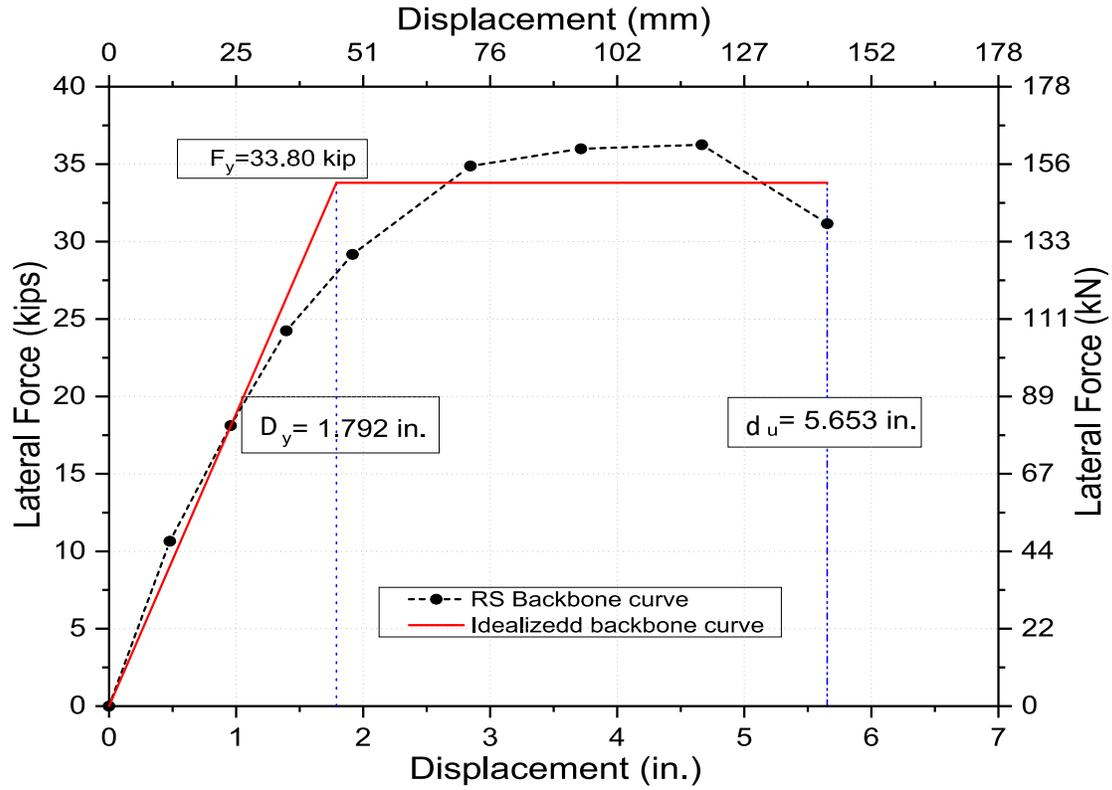
Figure 8.8 Modern code repaired (MCRP) displacement ductility
