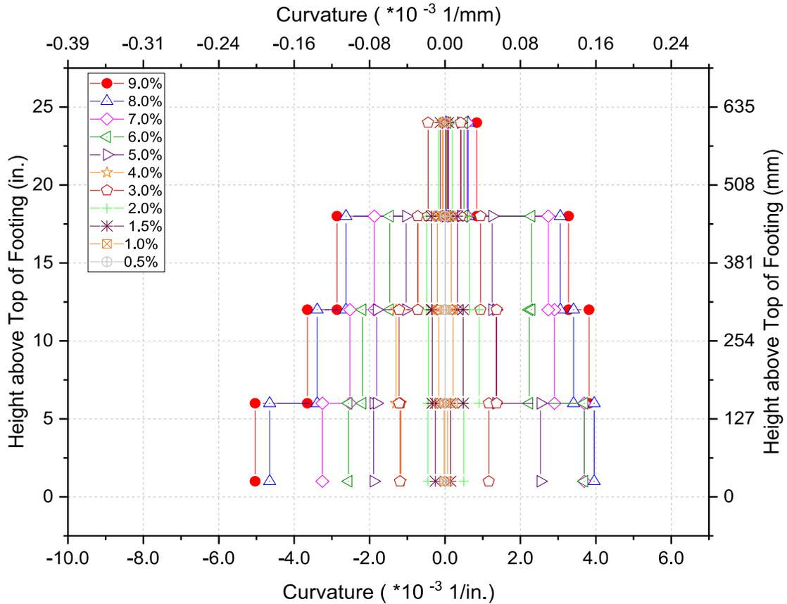
**Figure 4.8** Curvature profile of the modern code-compliant specimen
