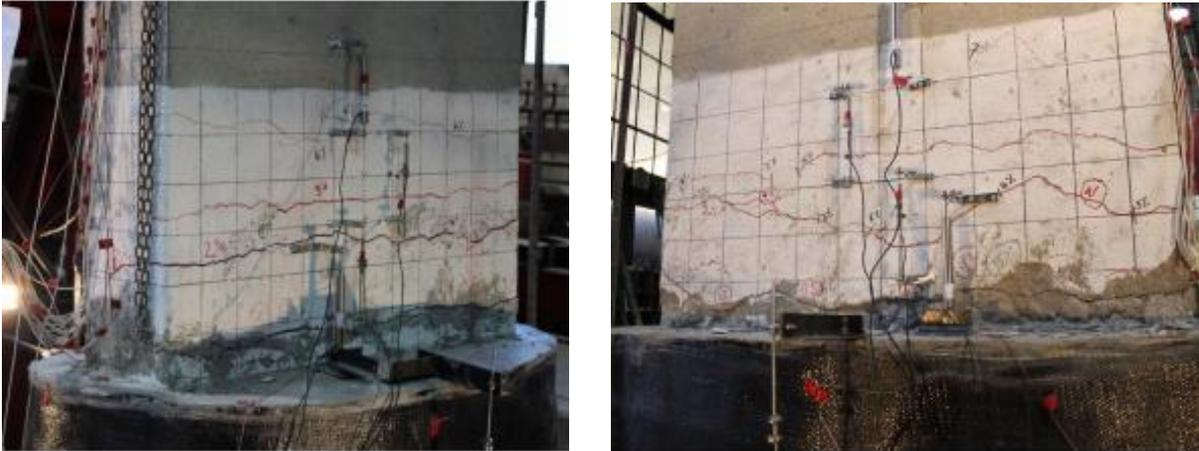
**Figure 8.14** Experimental observation of specimen MCRP at a 5% drift ratio: (a) east side (b) west side
