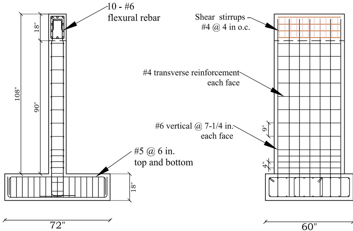
**Figure 2.7** Reinforcement details of current code-compliant specimen
