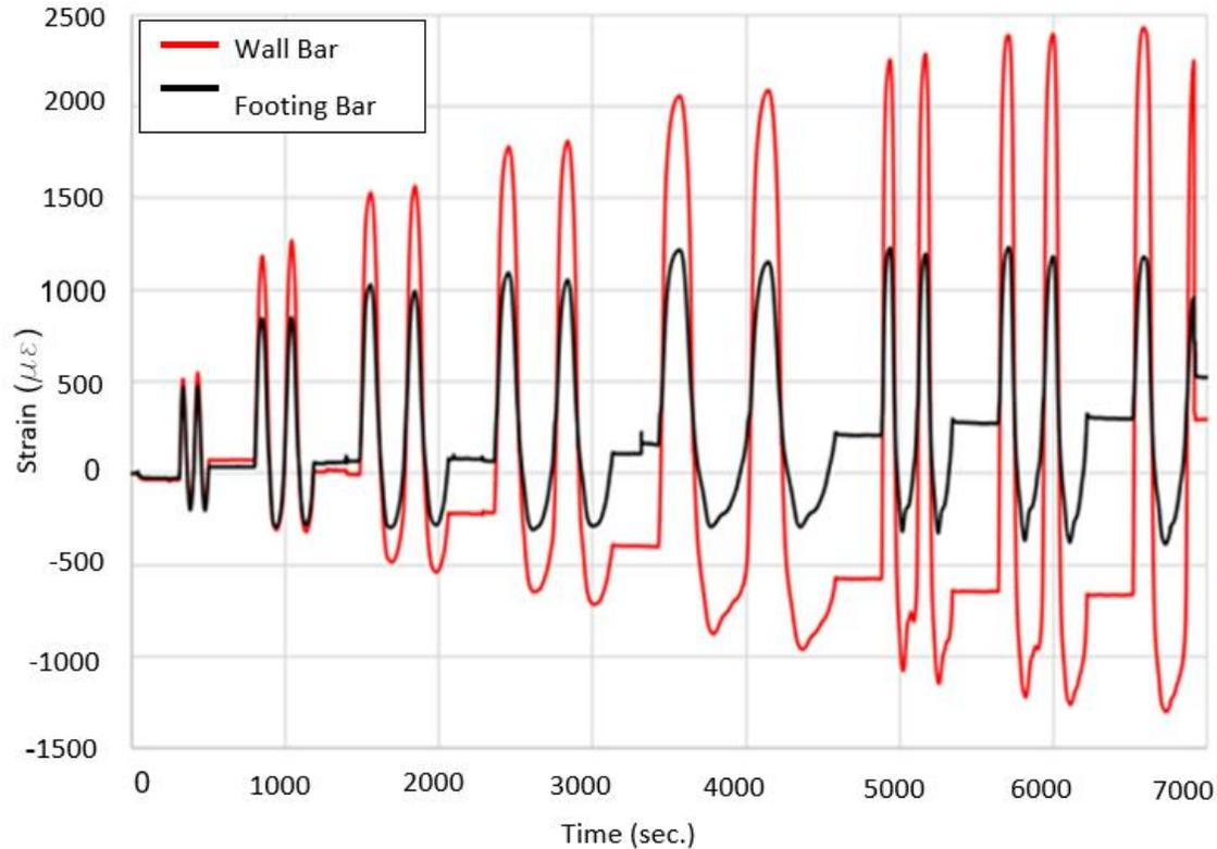
**Figure 3.8** As-built wall pier strain in lap-spliced bars
