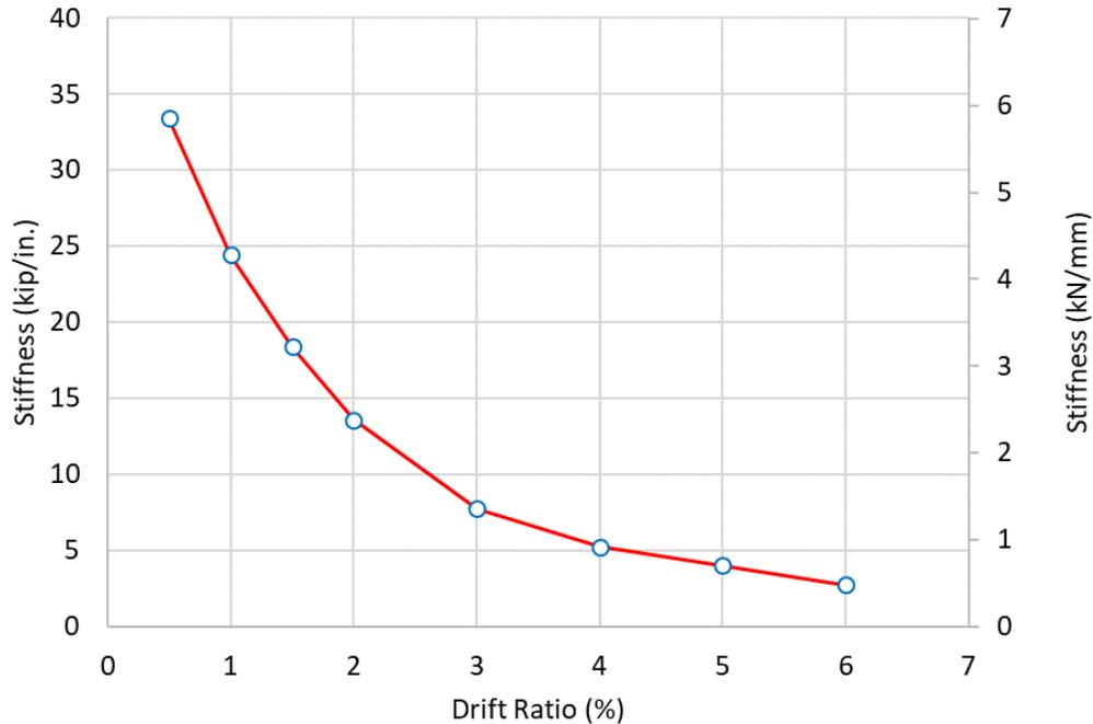
**Figure 5.7** Stiffness deterioration for retrofitted specimen R1
