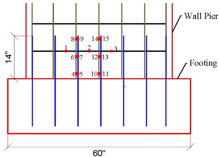
Figure 2.10 As-built wall pier strain gauge set-up
