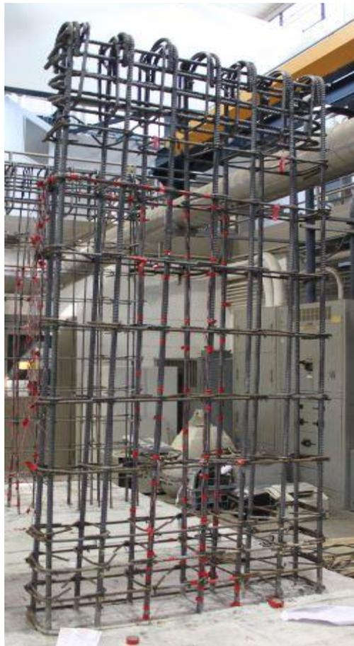
**Figure 2.9** Code compliant wall pier reinforcement
