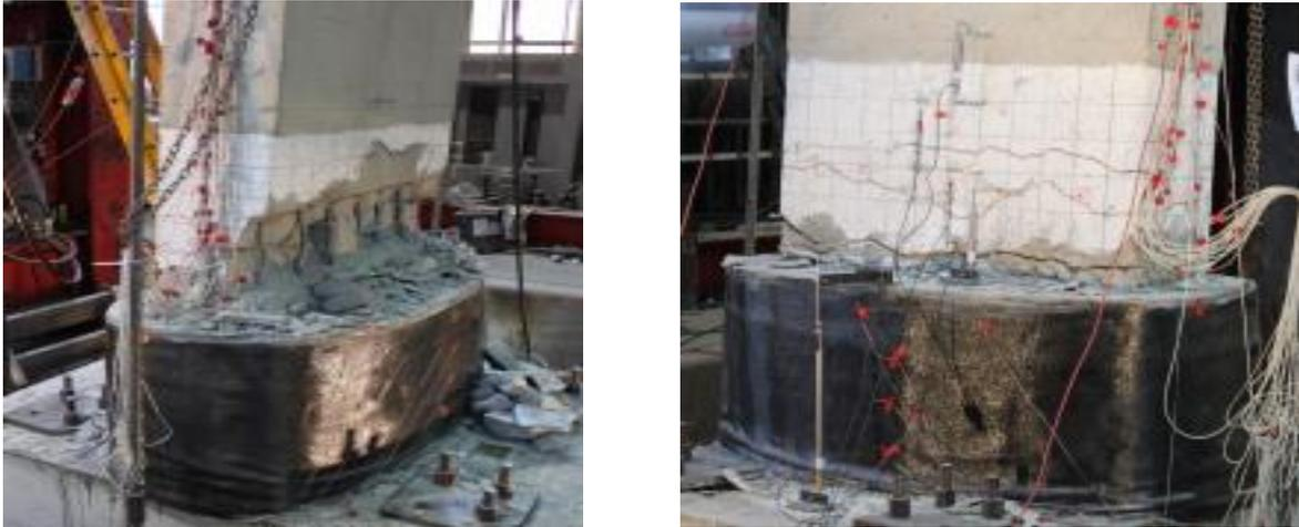
**Figure 8.15** Experimental observation of specimen MCRP at a 6% drift ratio:
