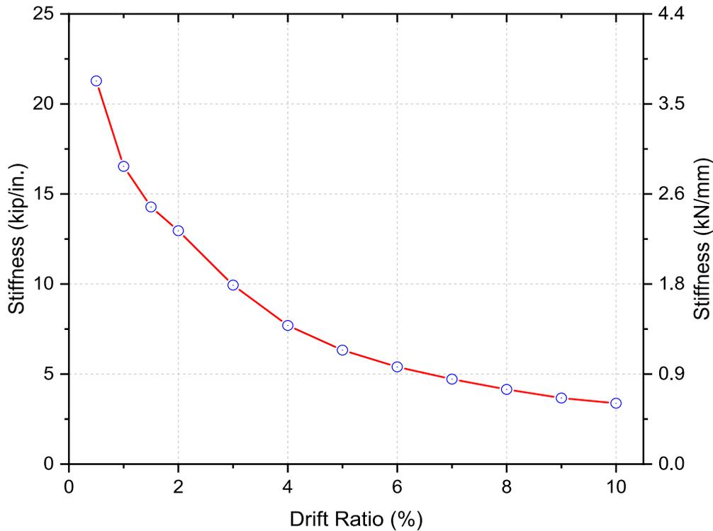
Figure 4.6 Stiffness deterioration of modern code compliant specimen
