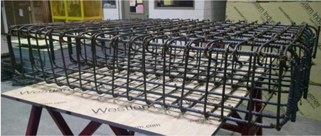
**Figure 2.5** As-built wall footing reinforcement
