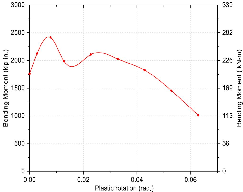
**Figure 6.7** Plastic rotation plot of retrofitted specimen R2
