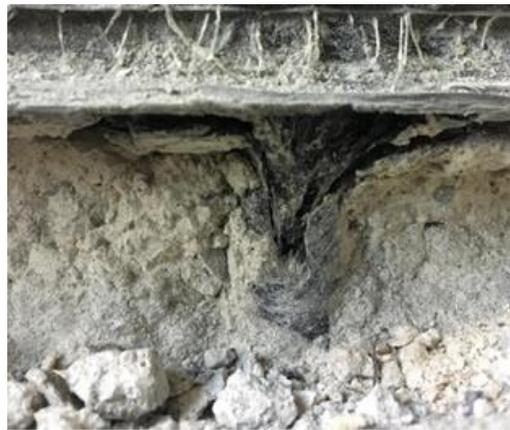
**Figure 5.11** Partial anchor fracture for Specimen R1
