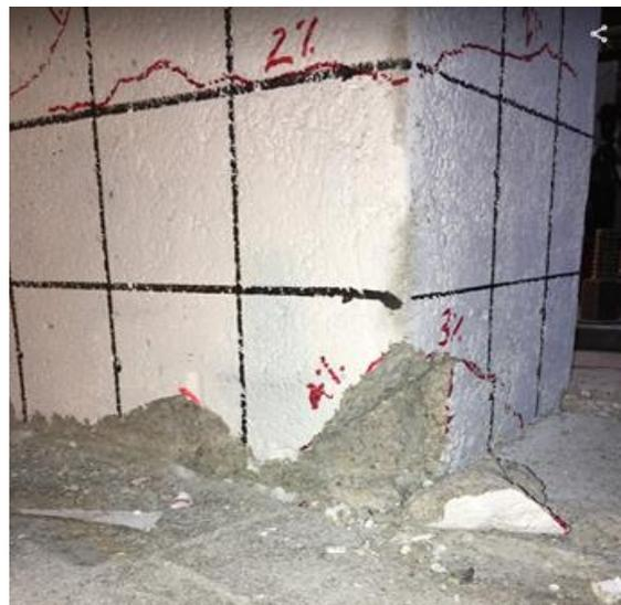
**Figure 3.10** Spalling at 4% drift of as-built wall pier
