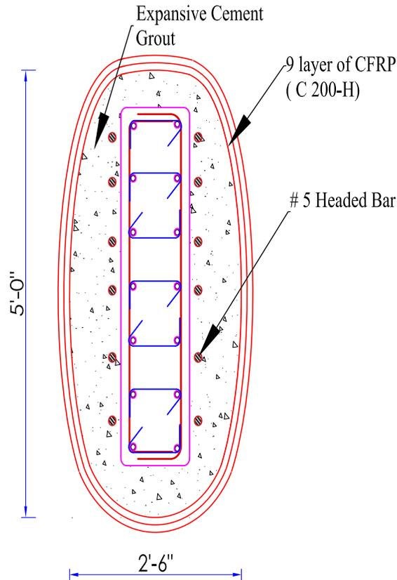
**Figure 8.2** Elliptical cross-section of the repair region for specimen MCRP
