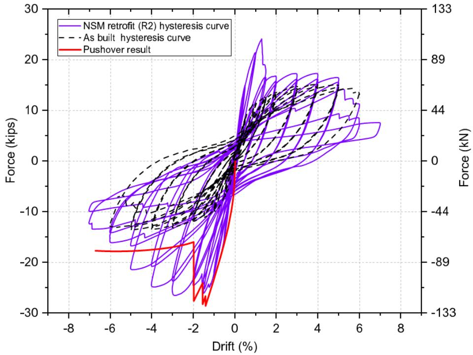
**Figure 6.14** Comparison of pushover results in pull direction considering gradual debonding of CFRP NSM rods from OpenSEES with the experimental results of the retrofitted specimen R2 and the as-built specimen
