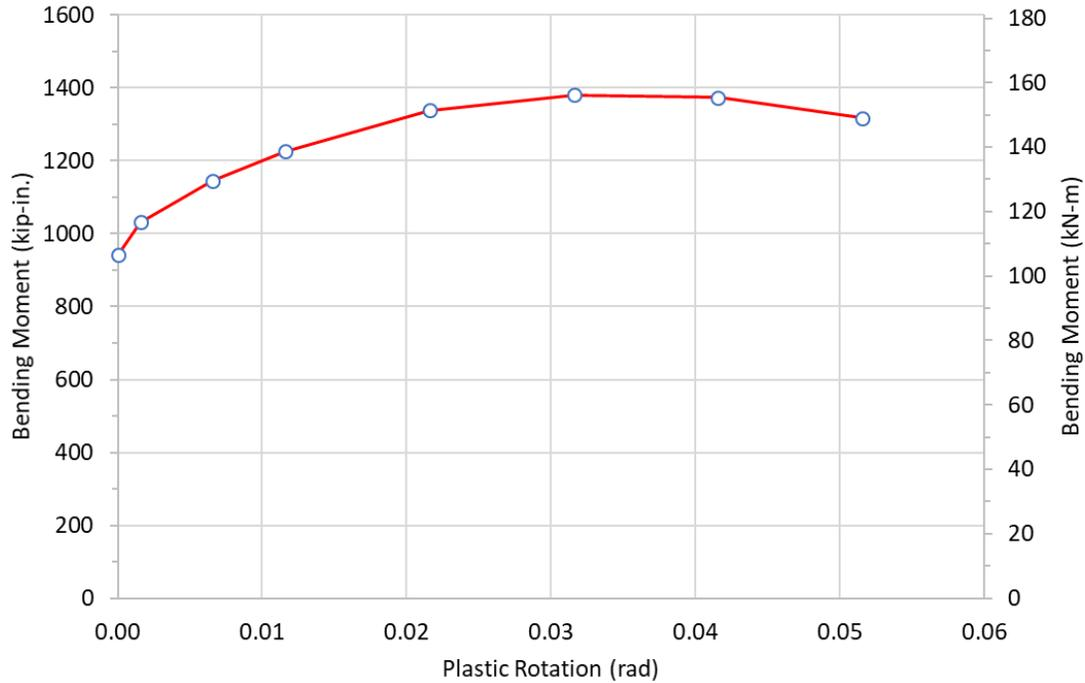
**Figure 3.3** Plastic rotation of as-built wall pier
