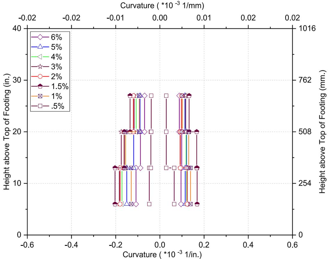
**Figure 6.10** Curvature Profile for Specimen R2
