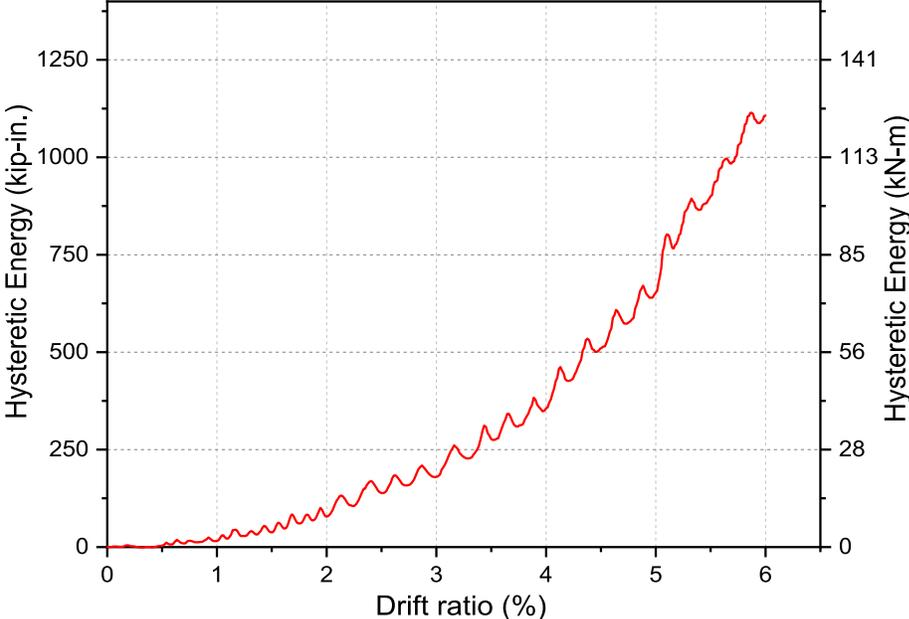
**Figure 8.11** Cumulative energy dissipation of repaired specimen MCRP
