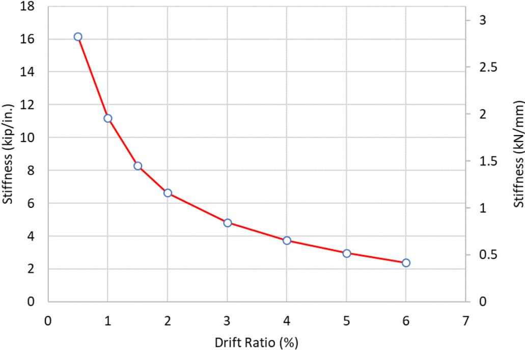
Figure 3.6 Stiffness deterioration of the as-built specimen
