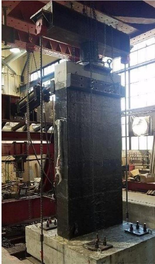
**Figure 6.3** Specimen R2 with the final retrofit application
