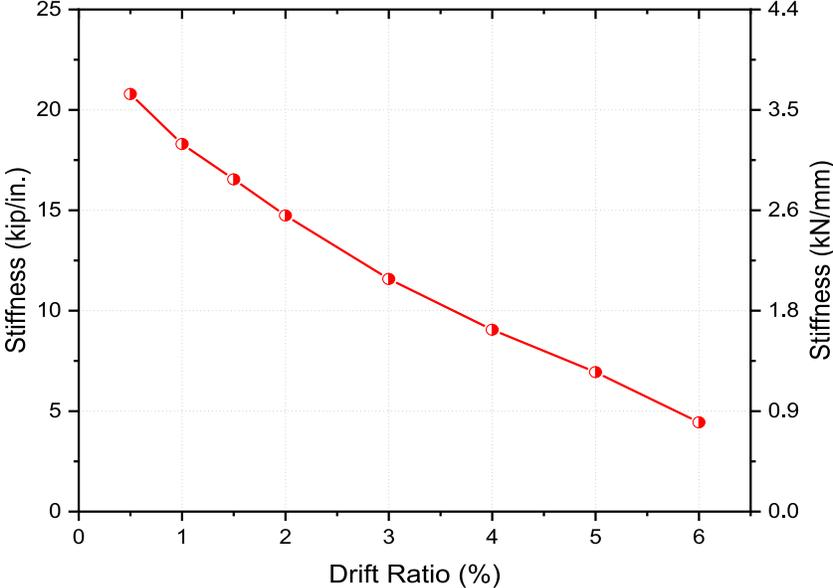
Figure 8.12 Stiffness deterioration of repaired specimen MCRP
