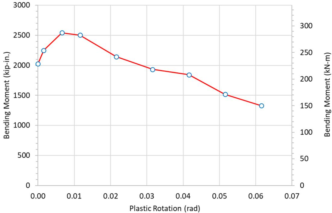
Figure 5.4 Plastic rotation plot for Specimen R1
