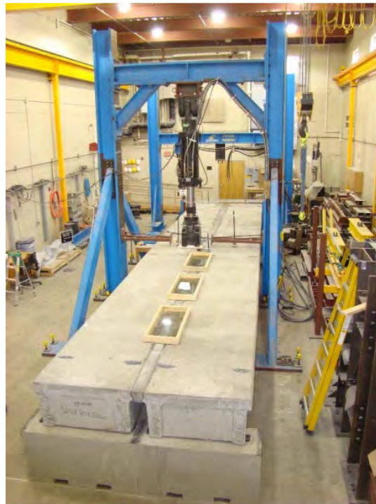
Figure 2.3 Full-Scale Conventional Double-Tee Girder Test Specimen (Konrad, 2014)
