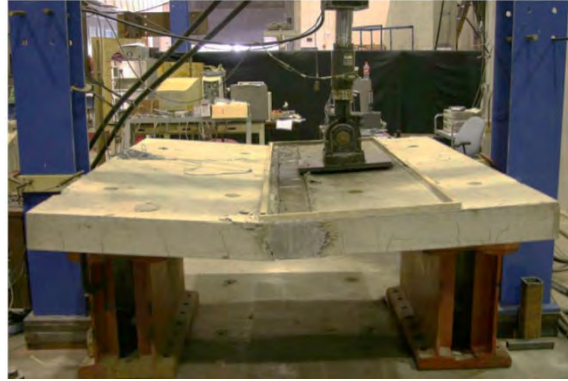
Figure 3.5 Failure of Longitudinal Deck Panel-to-Panel Joint with Straight Bars under Fatigue Loading (Graybeal, 2010)
