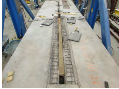
a. Top View, Continuous Joint Segment I Formwork
