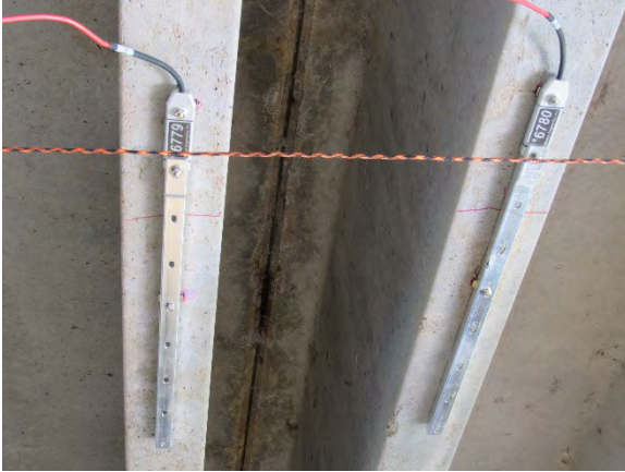
(a) Installation of Strain Gauges with Extension
