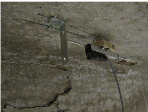
(c) LVDT underneath Flange for Rotations
