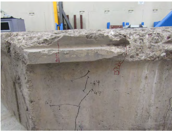
(c) Shear Crack Near North End
