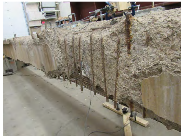
(f) Exposure of Strands and Transverse Bars on Stem of 50-ft (15.24-m) Girder
