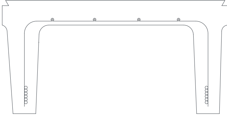
Figure 7.1 Stem Cover Deterioration with Condition State 1 equivalent to Undamaged Section
