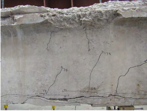
(a) First Flexural Crack at Midspan
