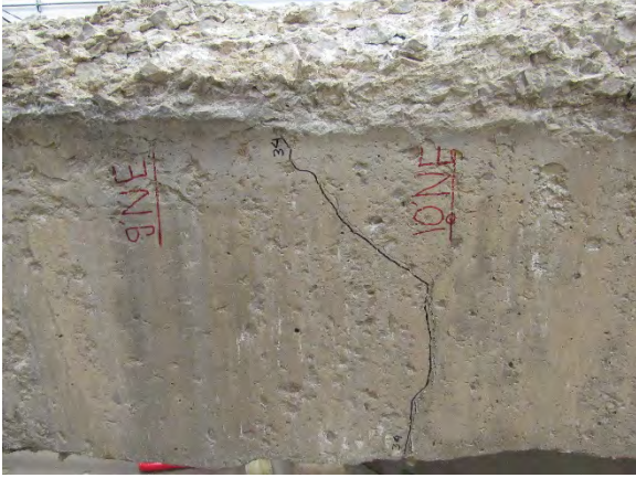
(a) First Shear Crack at North End
