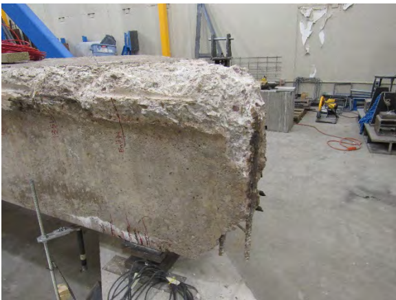
(e) Reinforcement Exposure of 30-ft (9.14-m) Girder
