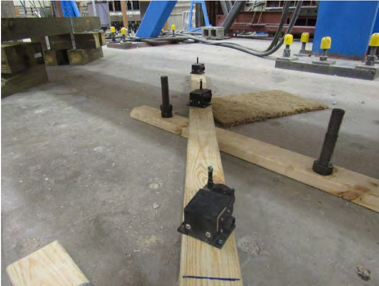
Figure 6.21 String Pot Installation at Midspan of 30-ft (9.14-m) Long Girder
