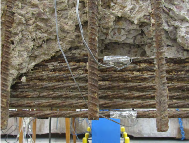
Figure 6.11 Installation of Steel Tendon Strain Gauges
