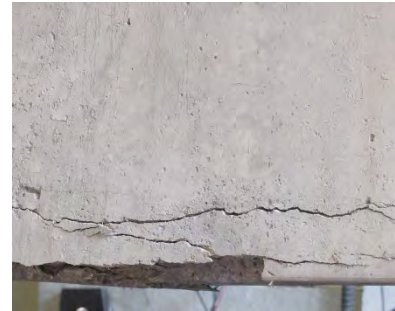
(i) Stem Cracking (CS-4)
