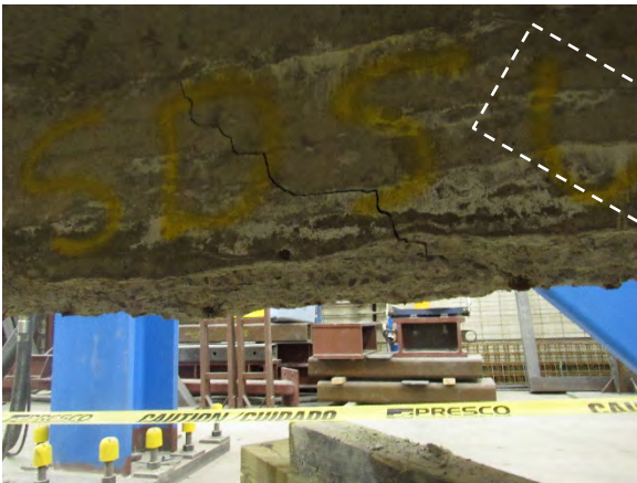
(e) A Major Flexural Crack at Midspan– Stem inside View
