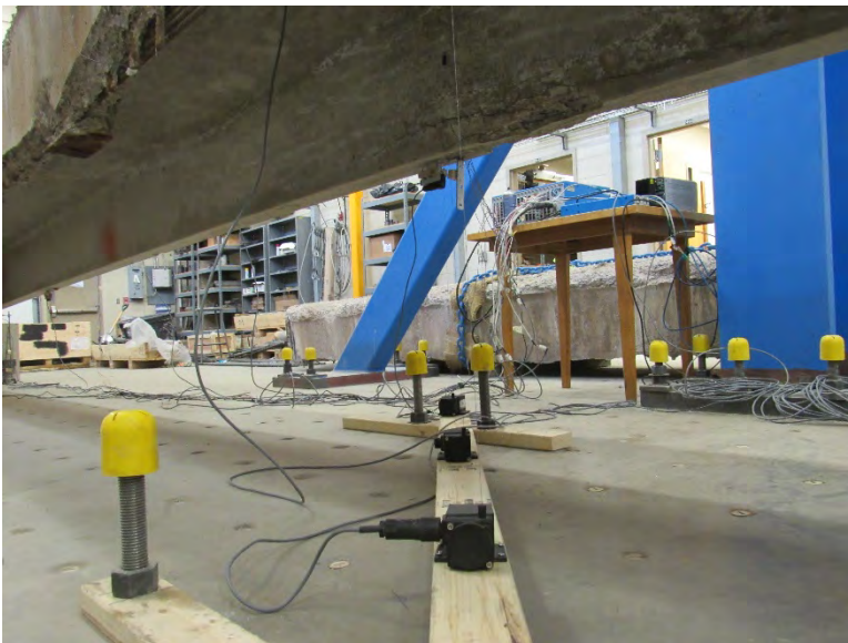
Figure 6.16 – String Pot Installation at Midspan of 50-ft (15.24-m) Long Girder
