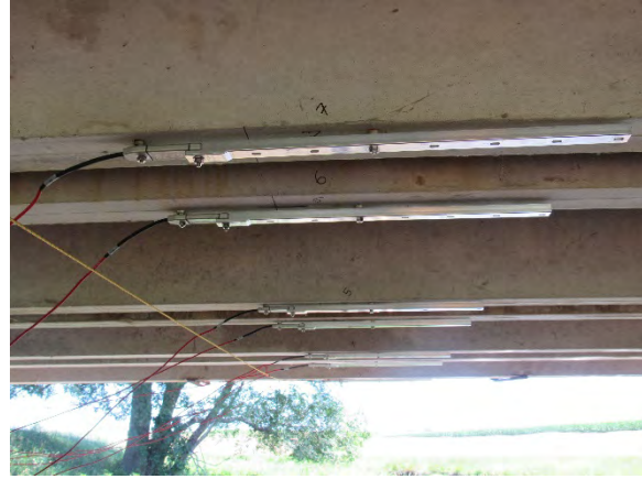
(b) Strain Gauges at Stem Bottom Face
