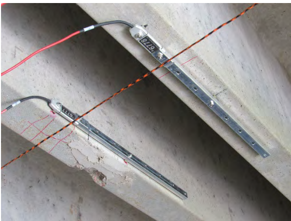
(c) Strain Gauges on Stem Side due to Damage
