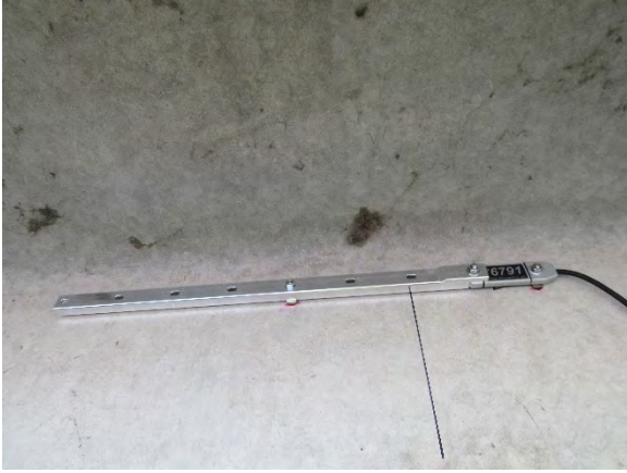
(a) Installation of Strain Gauges with Extension
