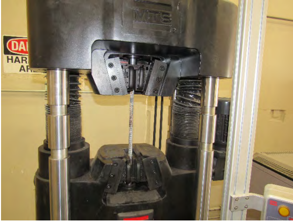
(a) Bar in Tensile Test Machine
