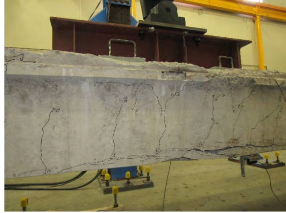
(b) Extension of Flexural cracks
