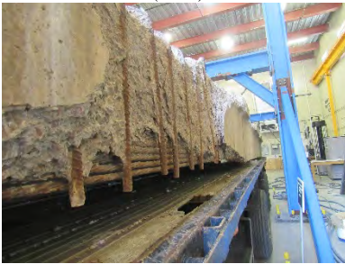
(p) Stem Exposure of Strand (CS-2)
