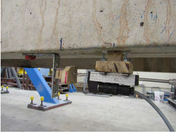
(a) LVDT as Concrete Strain Gauge
