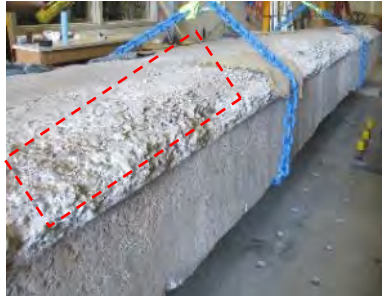
(e) Flange Cover Deterioration (CS-3)
