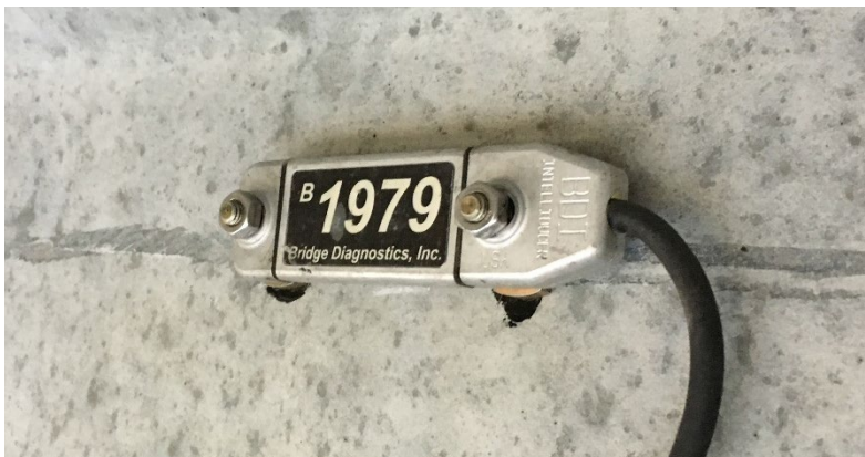
Figure 3.8 Strain transducer attached to the bridge (Pickett 2017)
