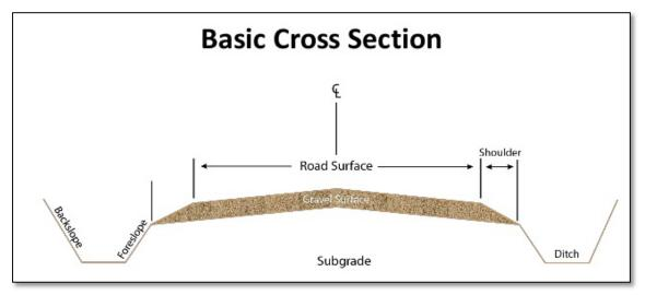
Figure 2.5 Roadway cross section
