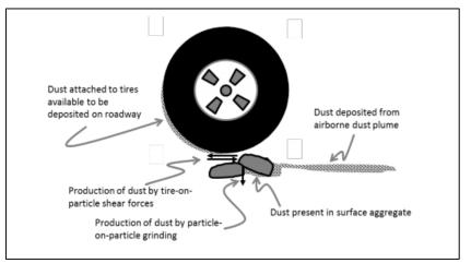
Figure 2.2 Sources of dust on gravel roads (Barnes, 2014)
