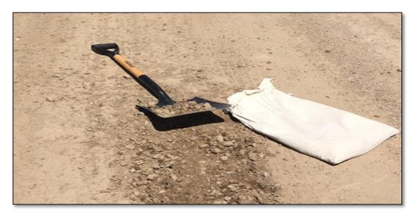
Figure 4.8 Aggregate sampling
