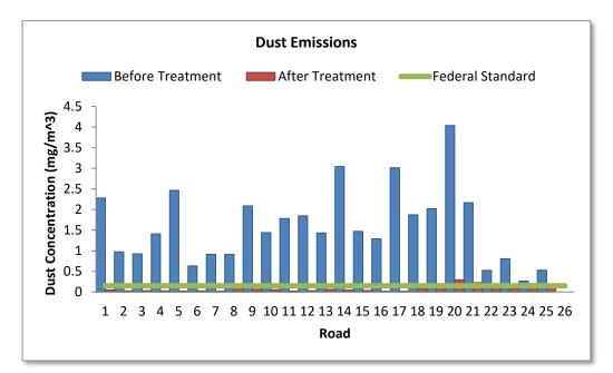
Figure 4.14 Comparing dust emissions before and after treatment
