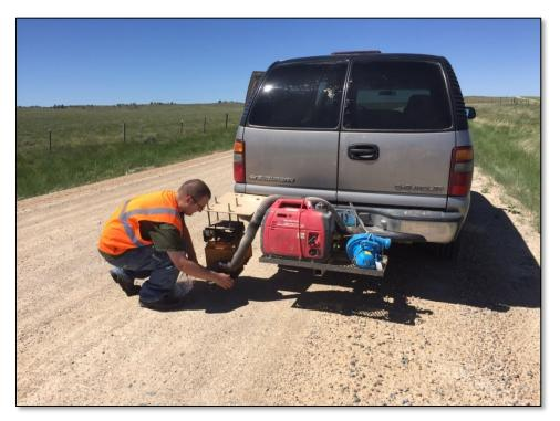
Figure 4.3 CSU-DUSTOMETER
