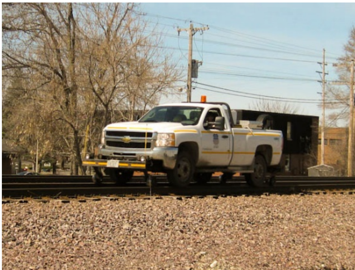
Figure 4.1 A typical hi-rail vehicle
