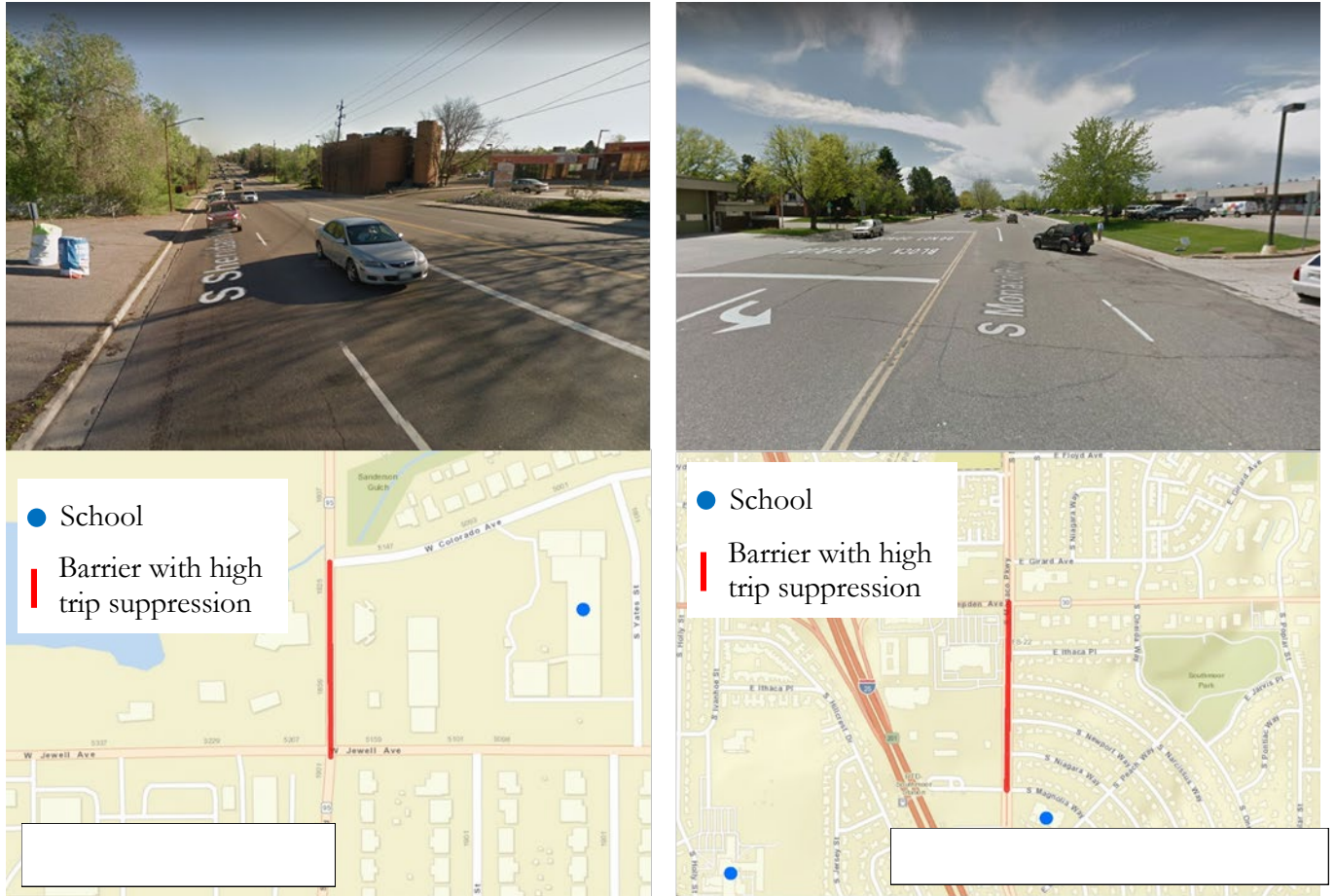
Figure 12.3 Examples of High Trip Suppression around Schools near Major Roads (Sheridan Boulevard on the left; Monaco Parkway on the right)
