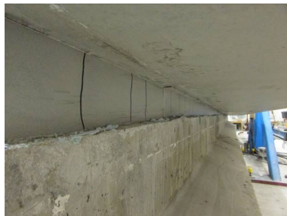
(d) Close Up of Girder B Haunch Region Filled with Non-Shrink Grout
