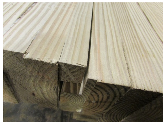
(f) Interlocking Deck Panels
