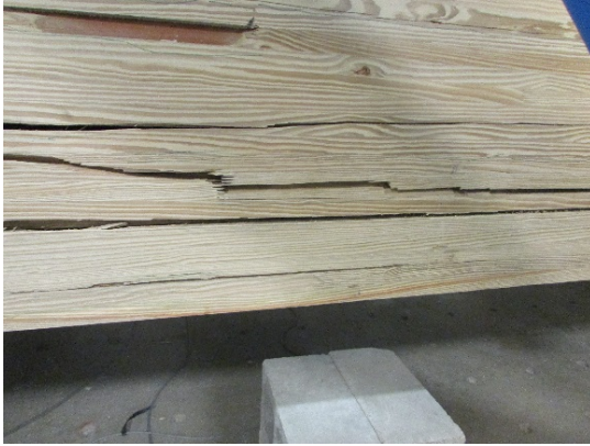
(a) Failure of West Girder
