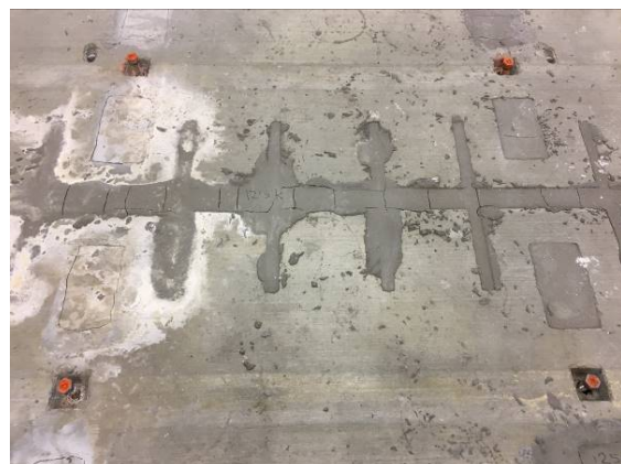
(b) Latex Modified Concrete at 650,000 Cycle
