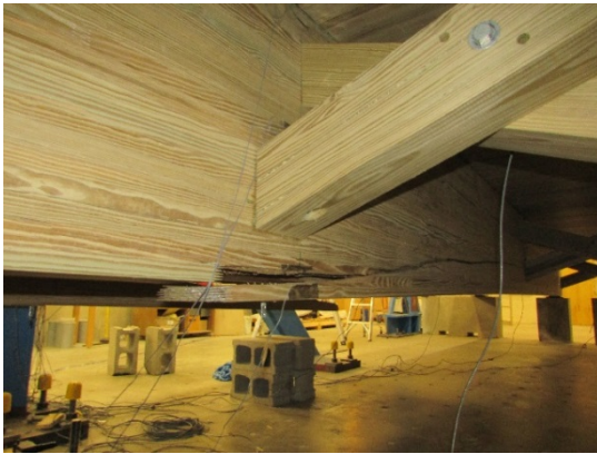
(c) Failure of Interior Girder
