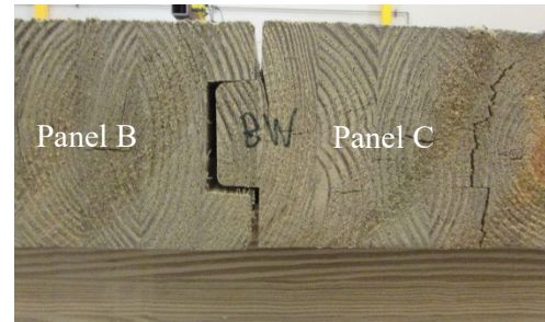
(g) Panel B-to-C Connection after 250,000 Cycles
