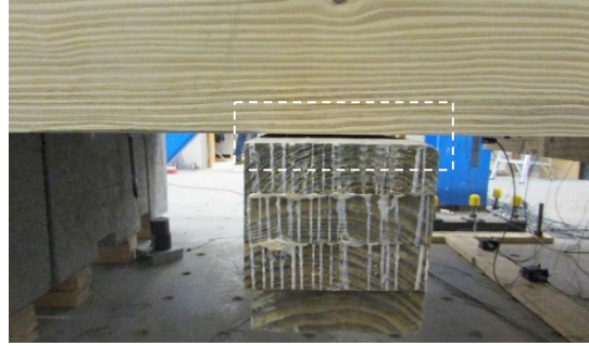
(b) Separation of Deck Panel and Stiffener
