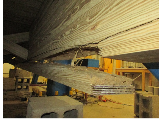
(b) Failure of West Girder
