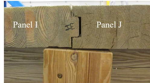
(c) Panel I-to-J Connection at 250,000 Cycles
