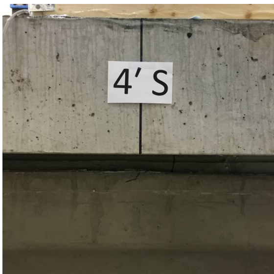
(a) Observed Crack at 25,000-Load Cycle
