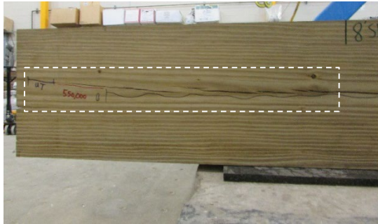
(a) Crack Growth at South Support after Testing
