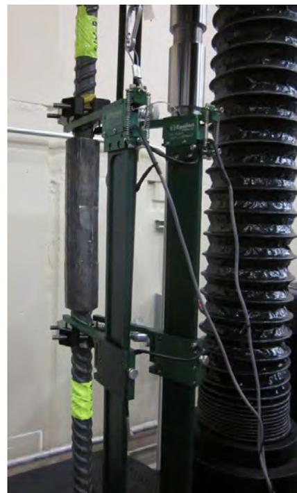
(b) Device with coupler extensometer
