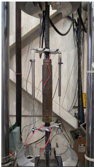
(c) Device with two LVDTs (NCHRP 12-105)
