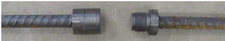
**Figure 2.4** One sample of headed reinforcement couplers
