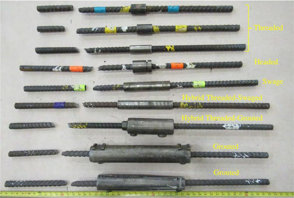
**Figure 2.1** Different mechanical bar splice products and types
