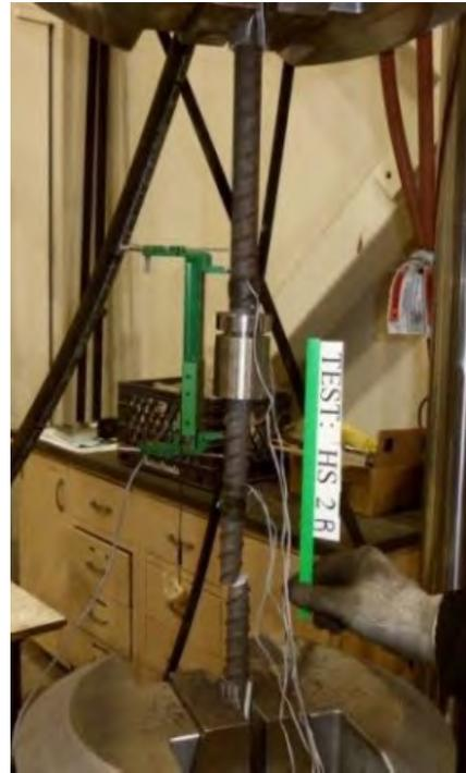
(b) Device with extensometer (Haber et al., 2015)
