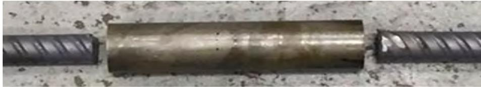
**Figure 2.6** One sample of swaged couplers
