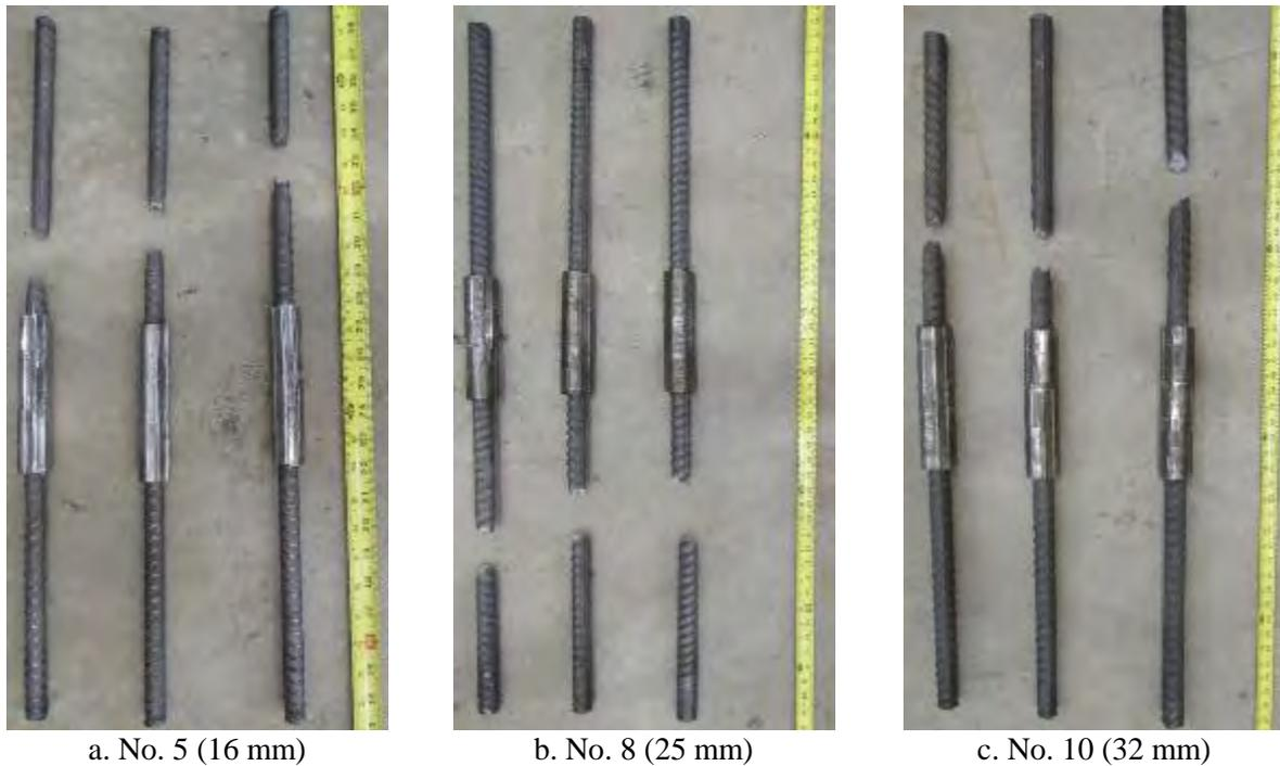
**Figure 4.51** Failure of swaged couplers under cyclic loading
