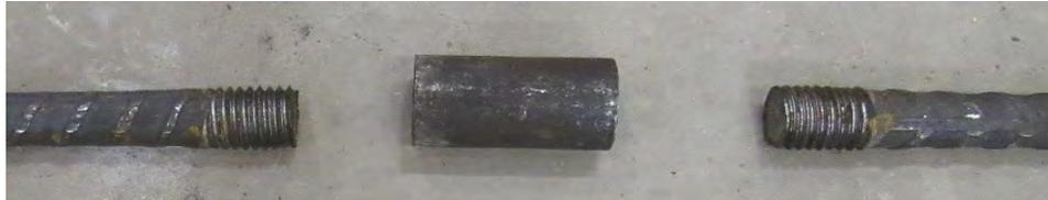
**Figure 2.3** One sample of threaded couplers
