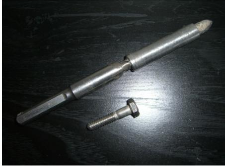
**Figure 4.50** ¼ x 1¼-inch Stainless Steel Hex Bolt and Bit
