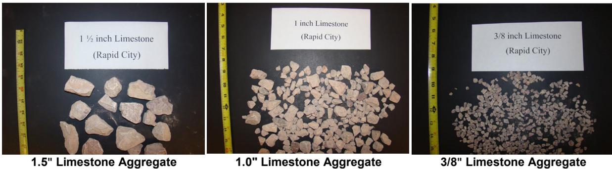
**Figure 3.8** Limestone Coarse Aggregates
