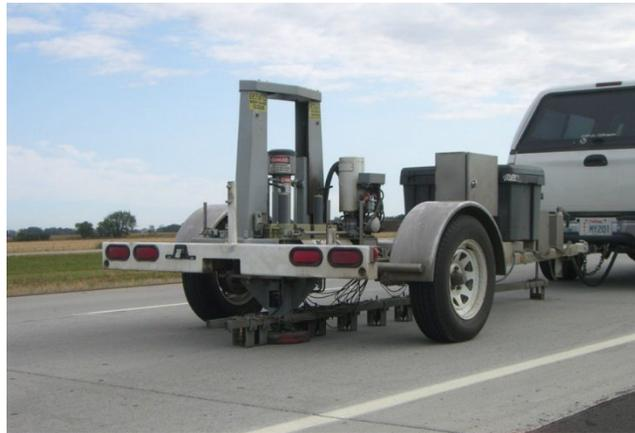
**Figure 4.59** FWD Apparatus
