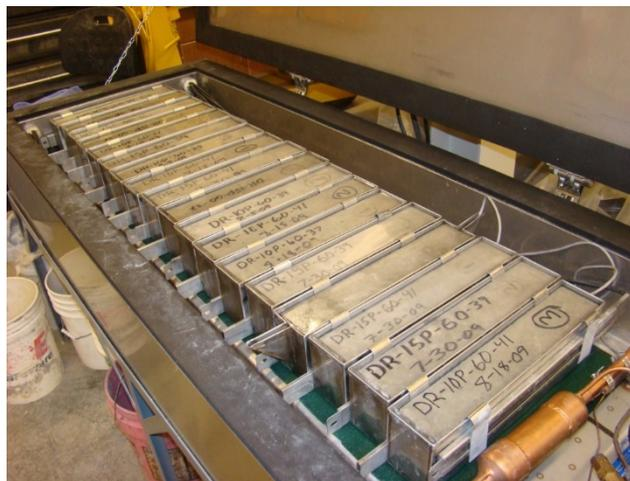
**Figure 3.24** Beam Specimens in the Freeze-Thaw Cabinet
