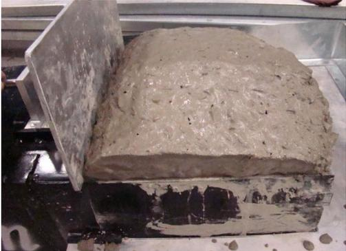
Concrete Overflow at the End of the Test
