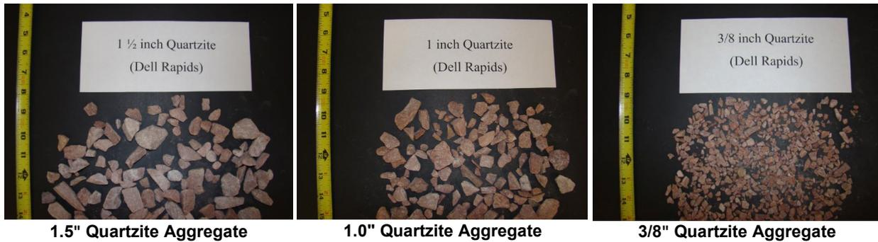
**Figure 3.7** Quartzite Coarse Aggregates
