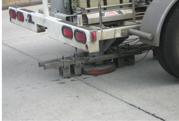
**Figure 4.61** FWD Test at a Transverse Joint
