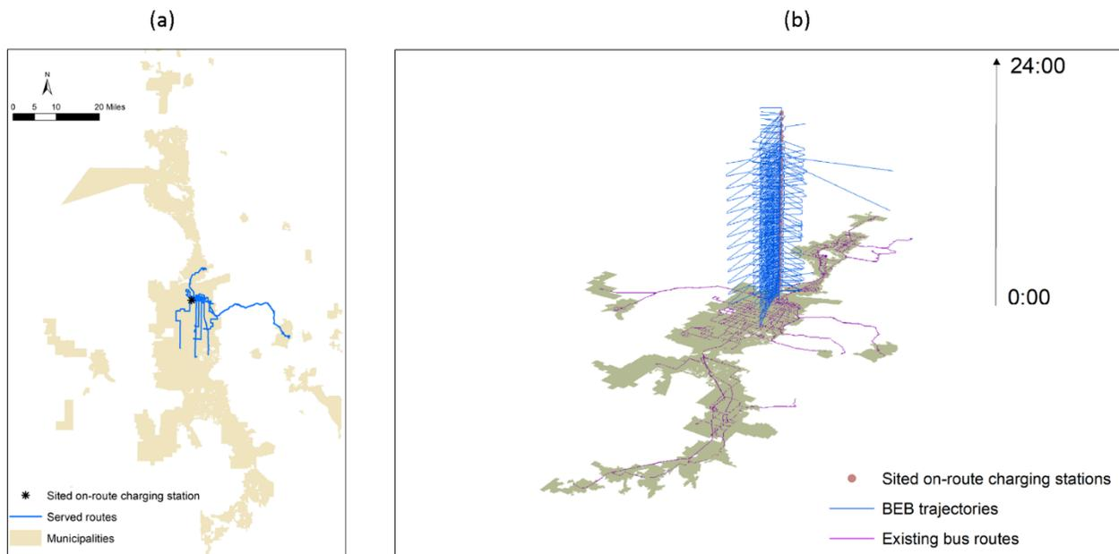
**Figure 4.5** Served Routes and Space-time Trajectories of BEBs When One On-route Charging Station is Built
