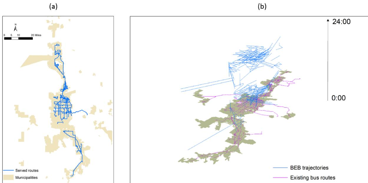
**Figure 4.4** Served Routes and Space-time Trajectories of BEBs When No On-route Charging Station is Built
