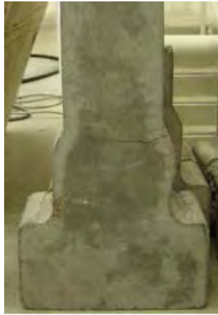
Figure 2.2 Double dog-bone geometry of a uniaxial direct tensile test specimen (Chao et al., 2011)
