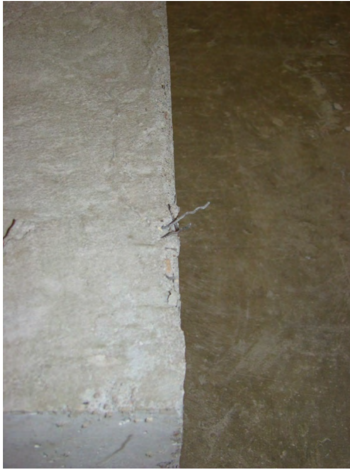
Figure 6.27 Steel fibers sticking out of the concrete surface
