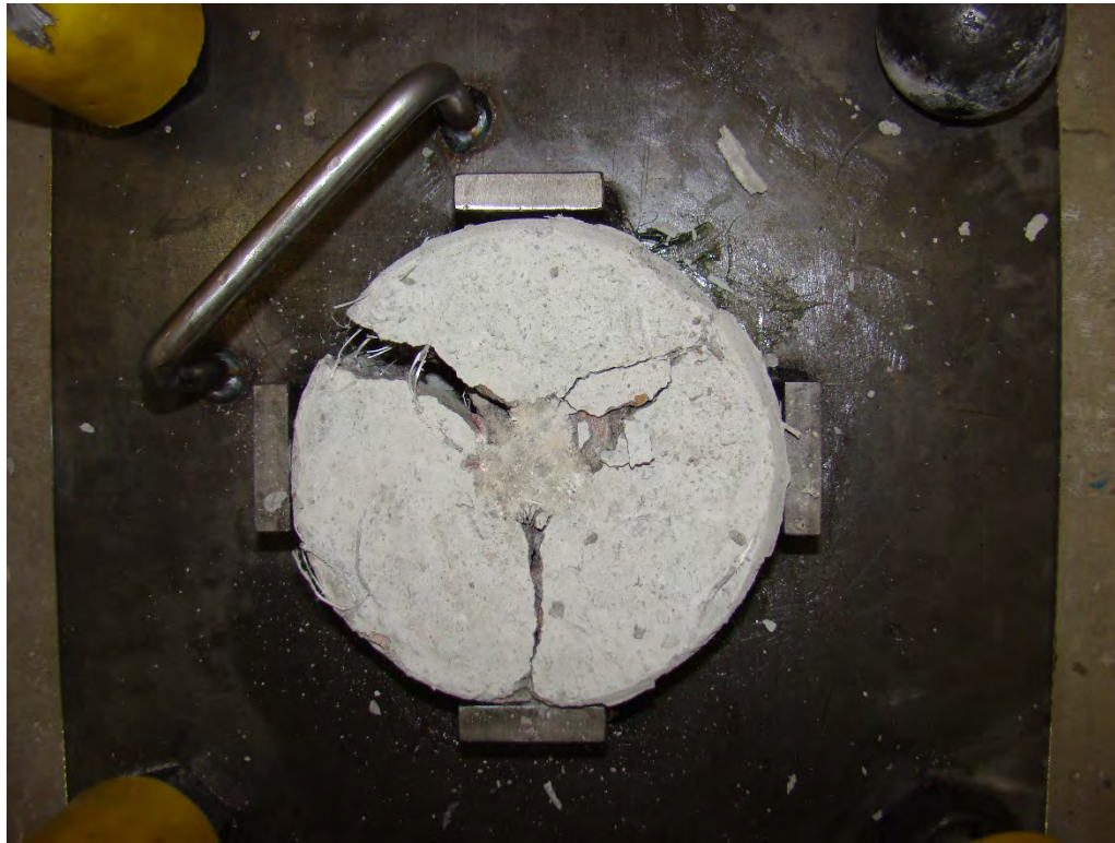
Figure 5.25 Failed impact specimen
