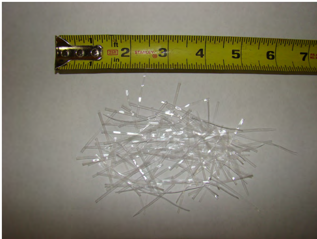
Figure 5.2 Fibermesh 650 fibers, manufactured by Propex
