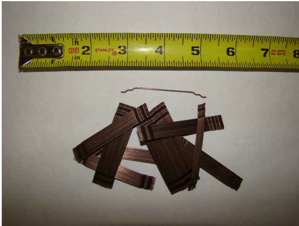
Figure 5.5 Dramix 5D fibers, manufactured by Bekaert
