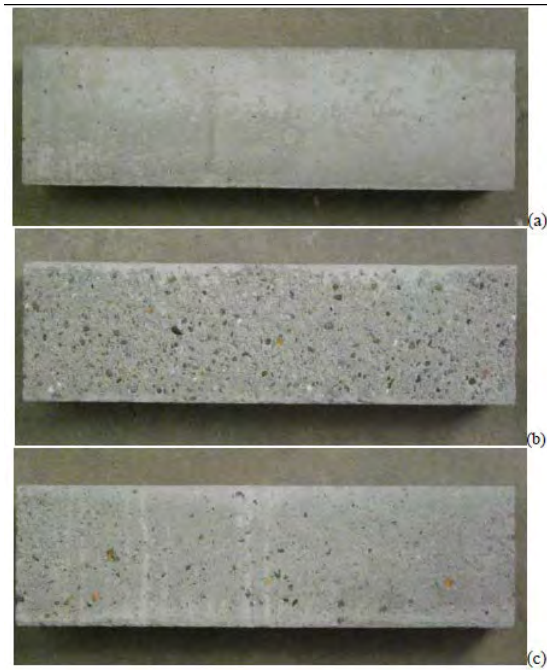
Figure 2.3 Surfaces of freeze-thaw specimens (a) before, (b) plain concrete after, and (c) HyFRC after freeze-thaw cycling (Ostertag and Blunt, 2008)
