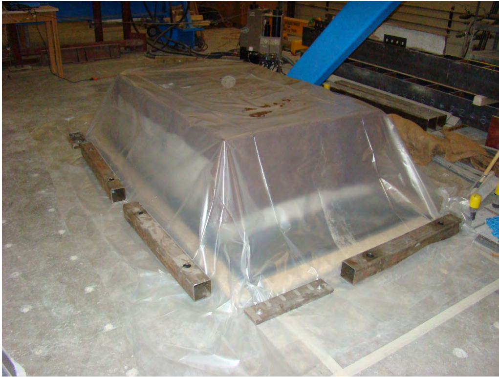
Figure 5.14 Plastic sheet placed over the top of the wet burlap to seal in the moisture
