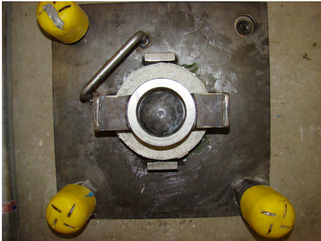
Figure 5.24 Top view of the impact strength testing setup
