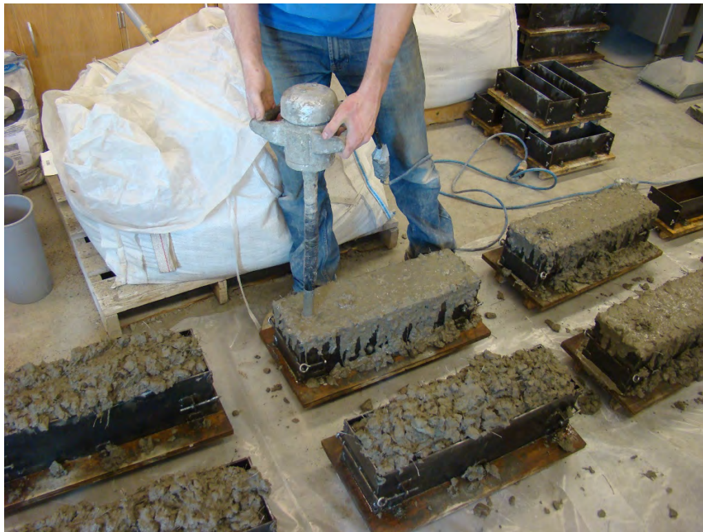
Figure 5.10 Hand-held spud vibrator in use
