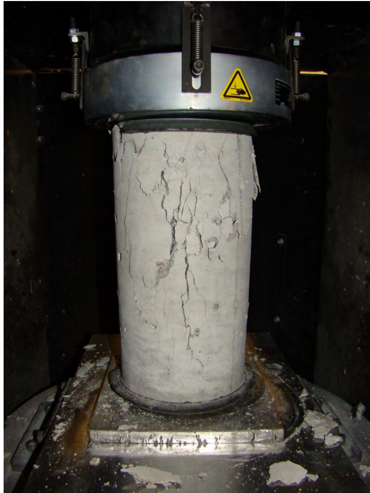
Figure 6.4 FRC compressive strength cylinder at failure
