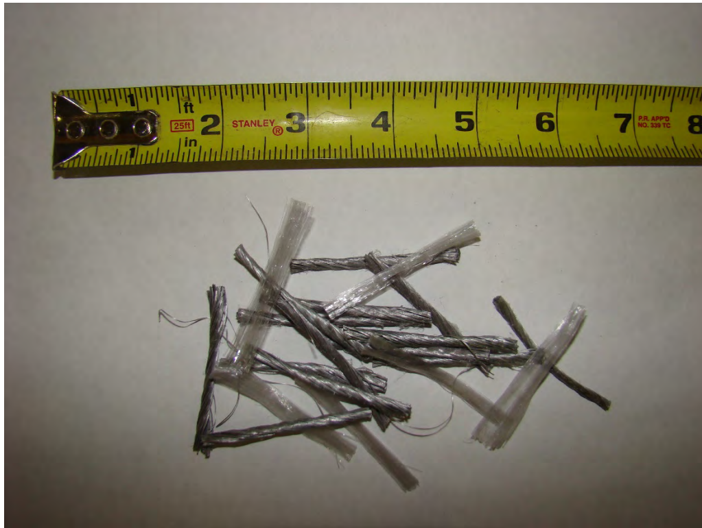
Figure 5.4 FORTA-FERRO fibers, manufactured by Forta Corporation
