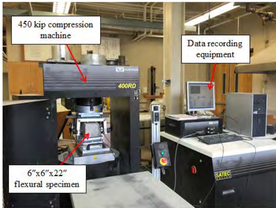
Figure 5.20 Flexural Performance (ASTM C1609) testing setup
