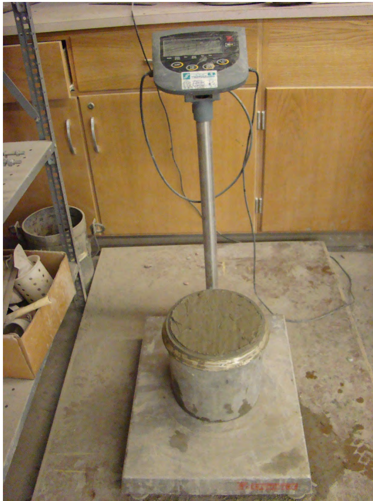
Figure 5.17 Determination of the fresh concrete unit weight, according to ASTM C138
