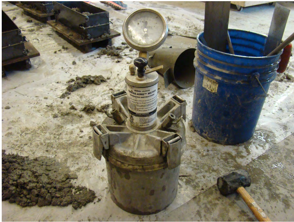
Figure 5.16 Air meter used to determine the concrete's air content, according to ASTM C231
