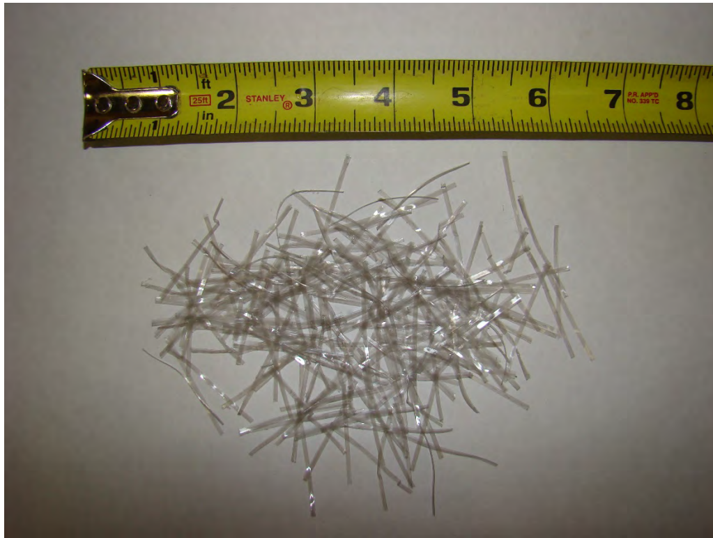
Figure 5.1 Strux 90/40 fibers, manufactured by W.R. Grace
