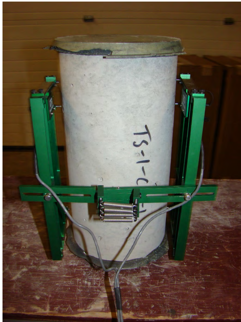
Figure 5.18 8" Extensometer used to measure the compressive strain of a concrete cylinder during testing, according to ASTM C39
