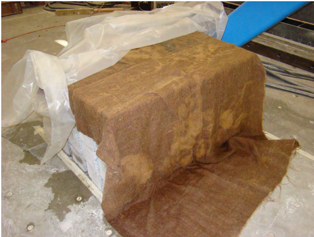
Figure 5.13 Wet burlap placed over the top of the concrete specimens in the curing chamber
