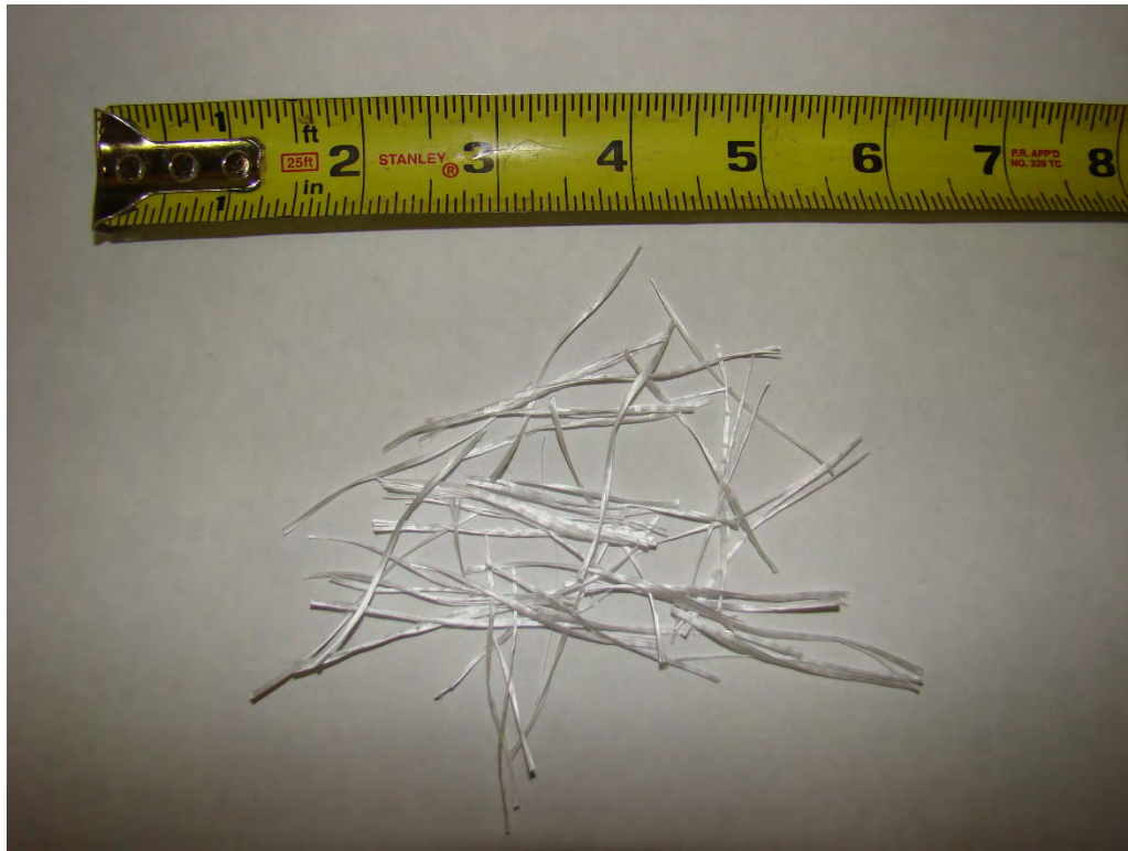
Figure 5.3 TUF-STRAND SF fibers, manufactured by The Euclid Chemical Company
