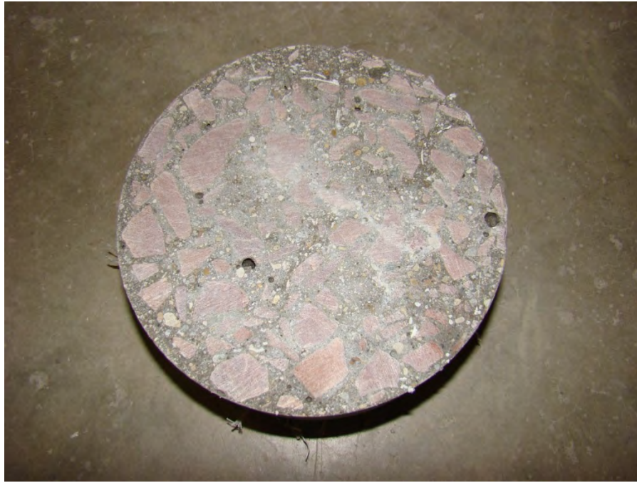
Figure 6.24 Cut surface of a synthetic FRC specimen
