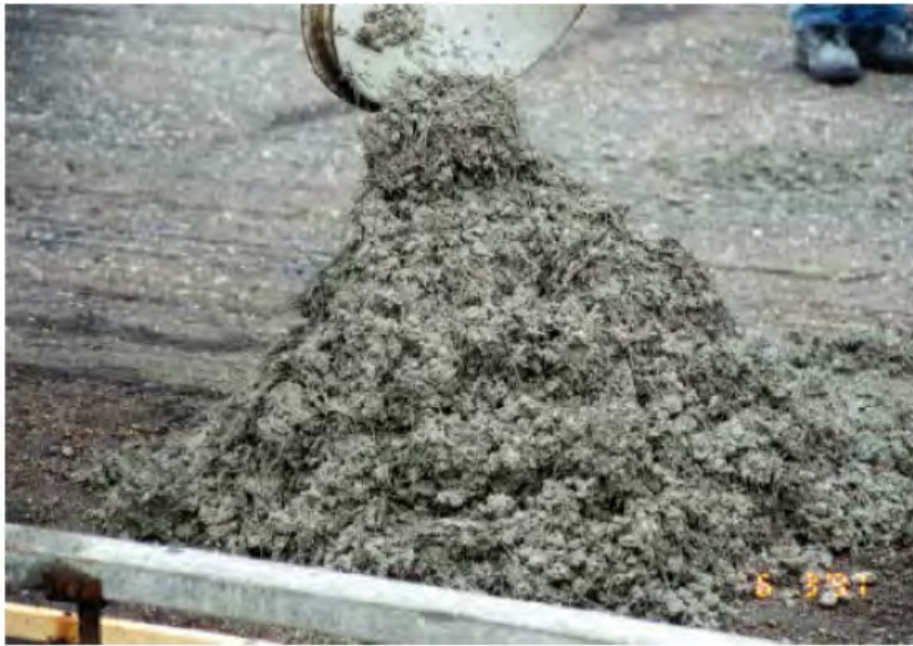
Figure 2.5 Consistency of a polyolefin FRC mix as it is discharged from the mixing truck (Dunn and Wolf, 2001)
