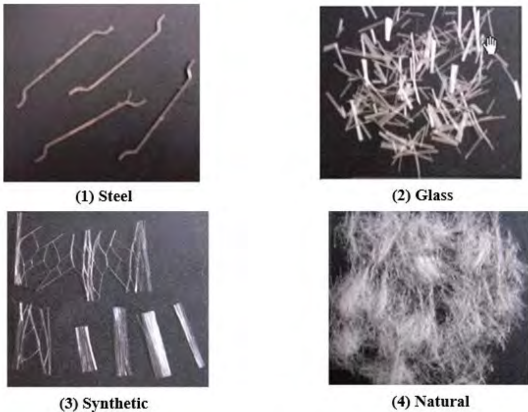
Figure 2.1 An example of each of the four fiber categories, as specified by ASTM C1116
