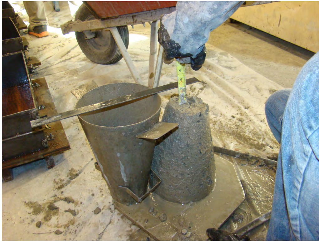
Figure 5.15 Measurement of the concrete slump, according to ASTM C143
