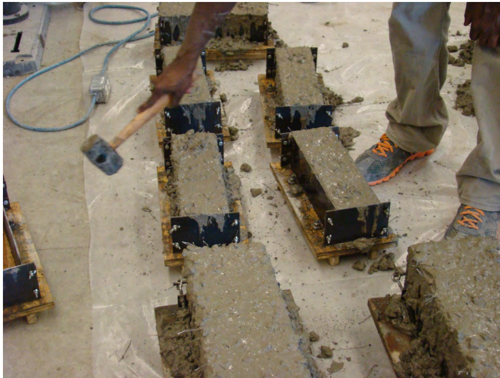
Figure 5.11 Use of rubber mallet to obtain final consolidation efforts of the concrete
