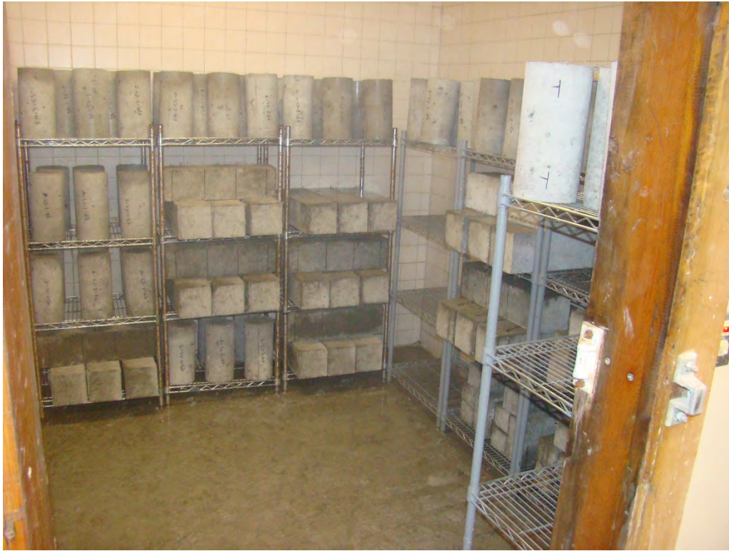
Figure 5.12 Moist cure room used to cure a majority of the testing specimens
