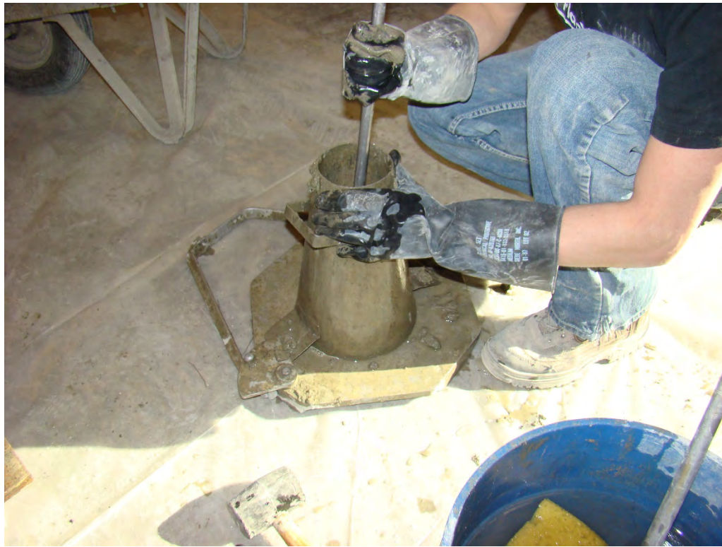
Figure 5.9 Rodding during a concrete slump test
