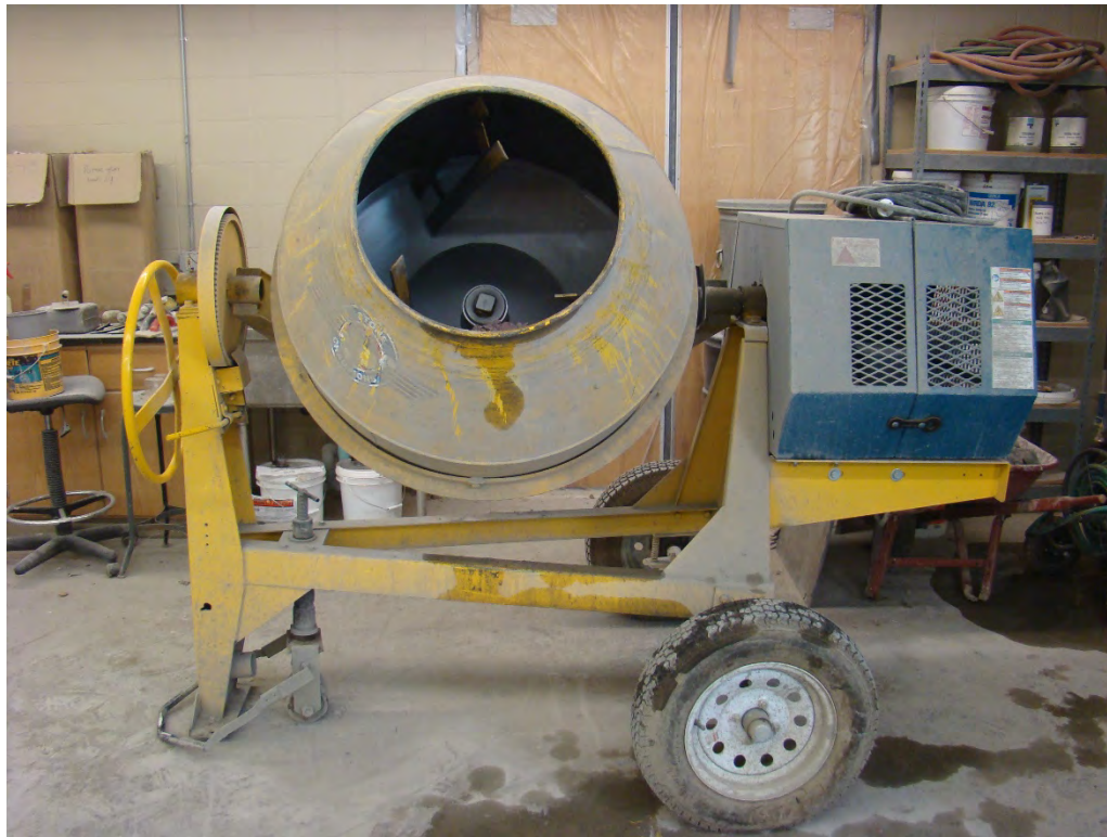
Figure 5.7 1/2-cubic yard capacity concrete drum mixer
