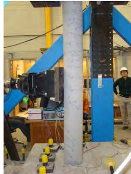
(b) Cracking in the Loaded Column
