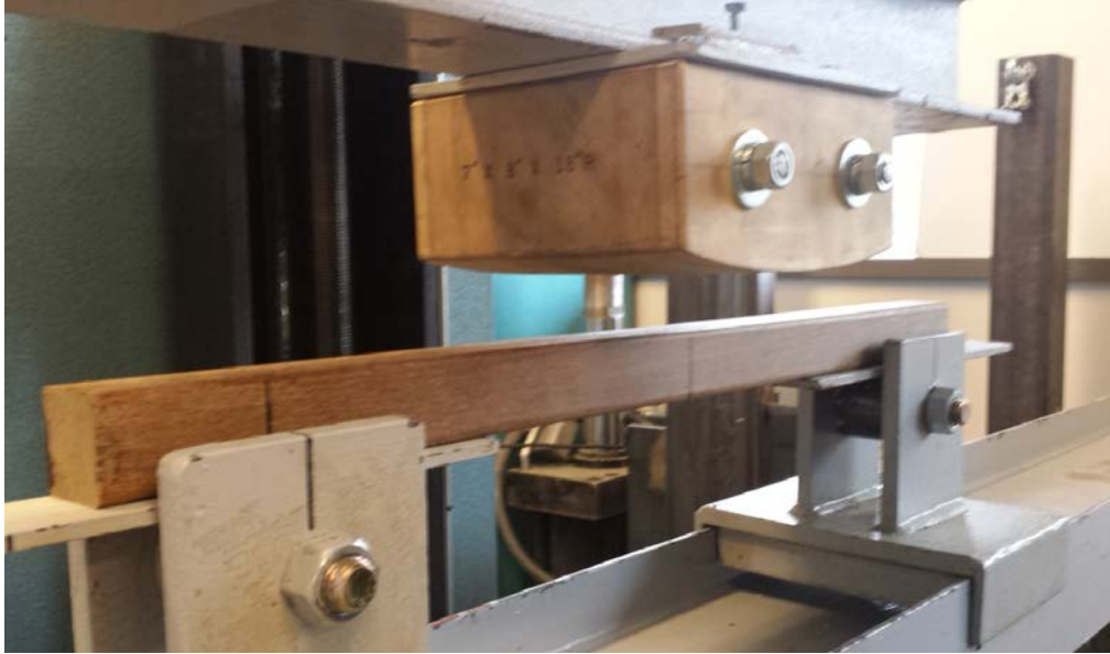
Figure 3.1 Instron UTM with Loading Mechanism and Ipe Specimen
