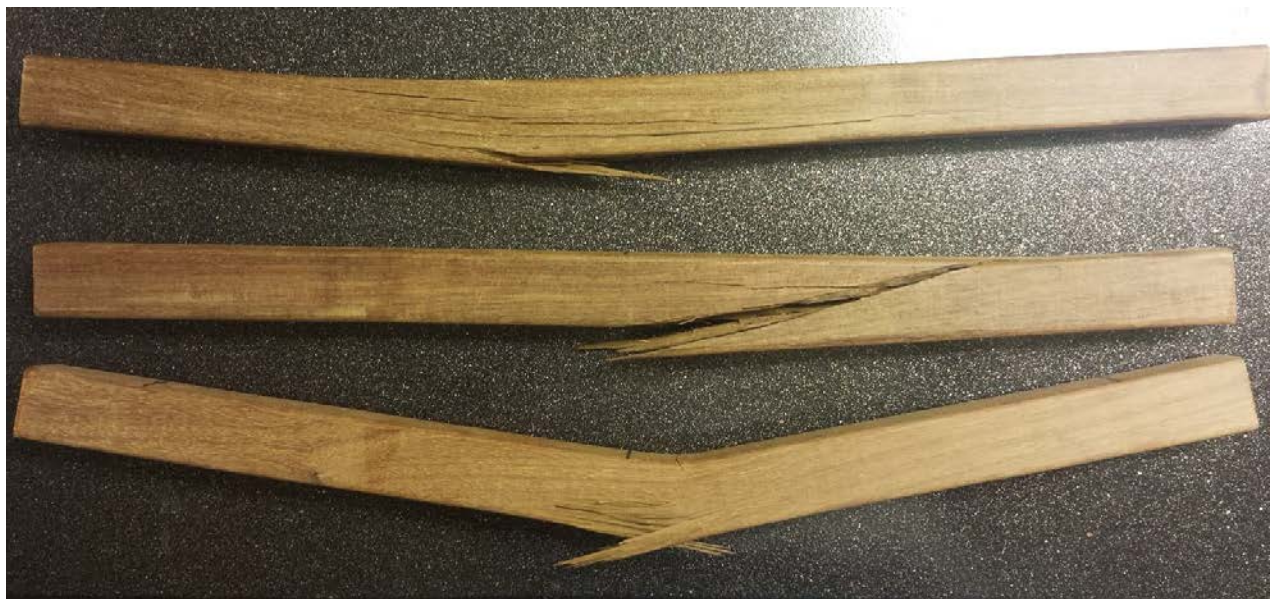
Figure 8 Ipe 3-pt Bending Specimens. (1 on top, 3 on bottom)
