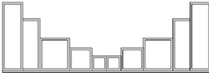
Figure 2.7 Cross-Section of “CGR10” Composite Configuration (Source: Bank 2001)
