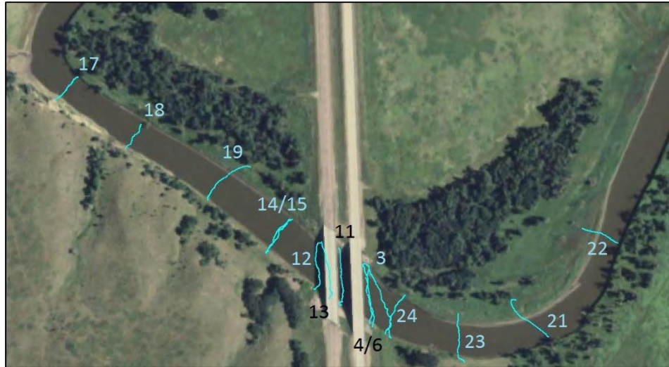
Figure 5.13 Location of ADCP measurements in April 2001 used for validation of 2D flow model
