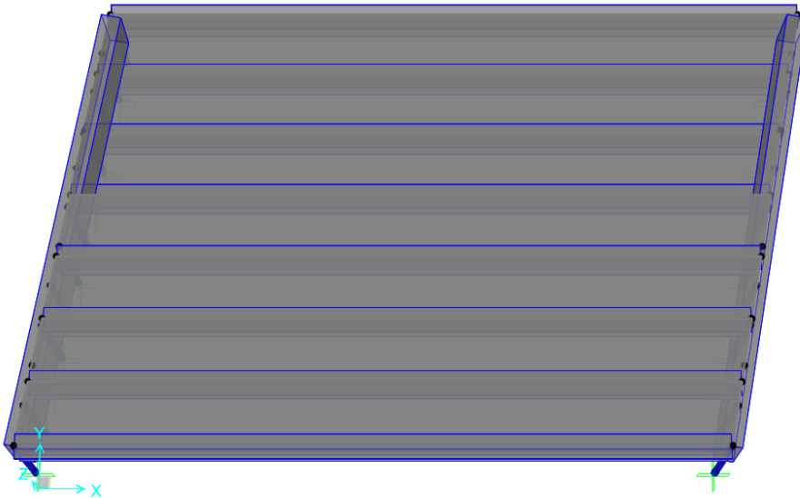
Figure 4.14 Parametric Skew Model with Skew Angle of 10°
