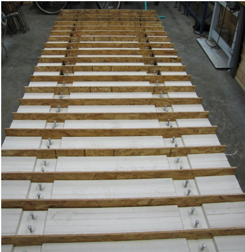
Figure 2.3 Specimens under construction with exposed notch detail
