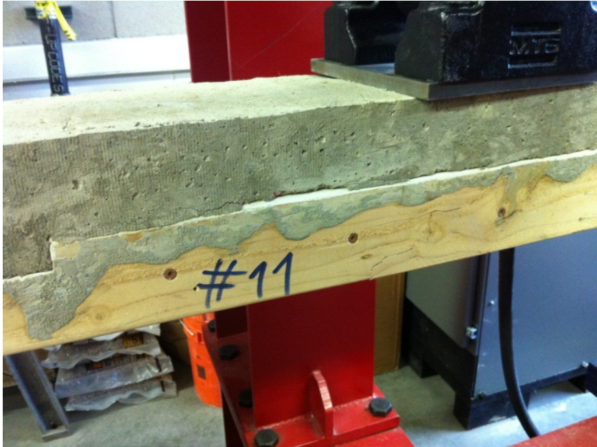
Figure 3.5 Typical tension failure (Specimen F11)
