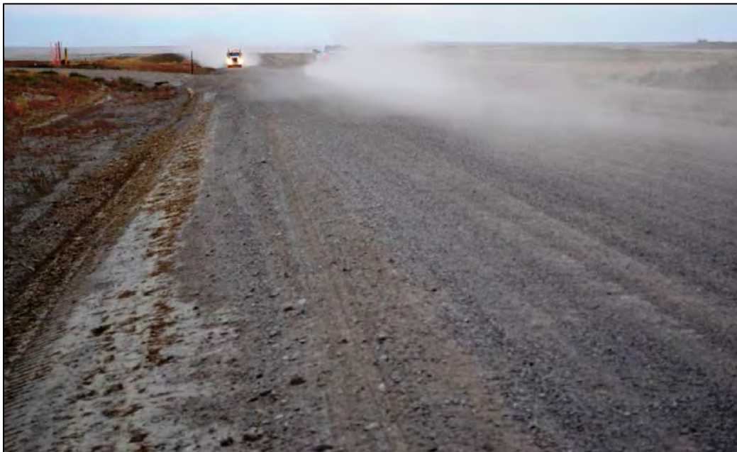
Figure 4.43 Dust from road surface made of reclaimed cement-treated base blended with existing aggregate and treated with magnesium chloride on segment J of Sweetwater County's Crooks Gap Road in September 2011, eight weeks after application of dust suppressants.
