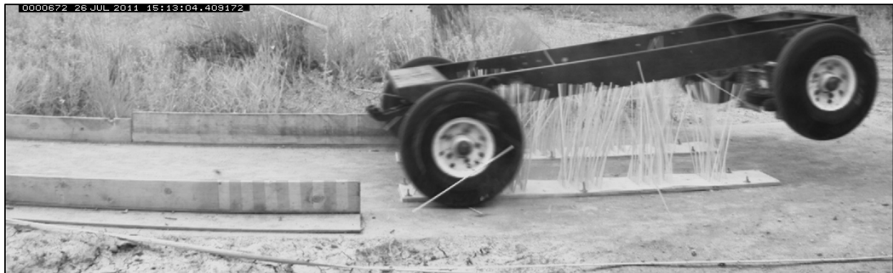
Figure 4.2 Cart lift due to tightly spaced clusters.
