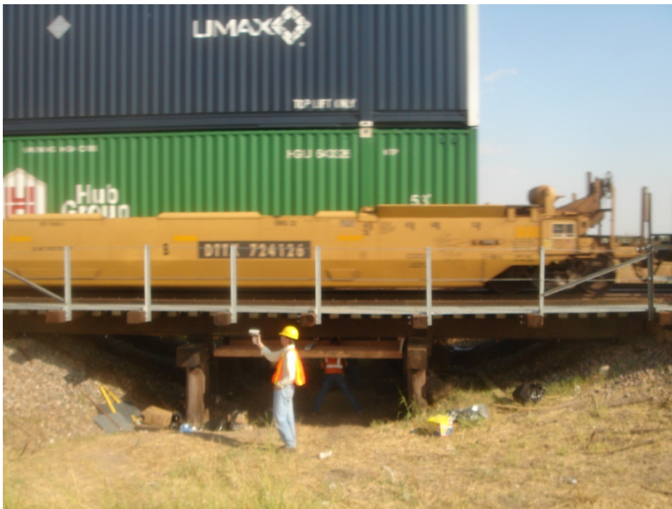
Figure C.50 Speed measured with Speed Gun.
