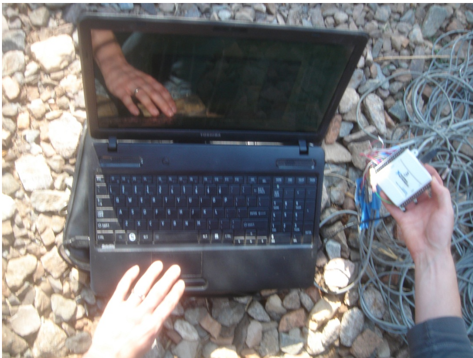
Figure C.30 Laptop and USB DAQ used for data acquisition.
