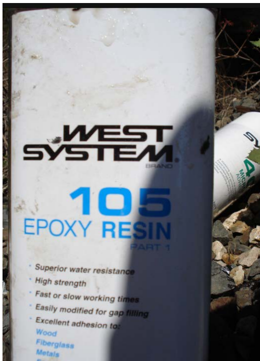
Figure B.6 Epoxy Resin Used for Spiking
