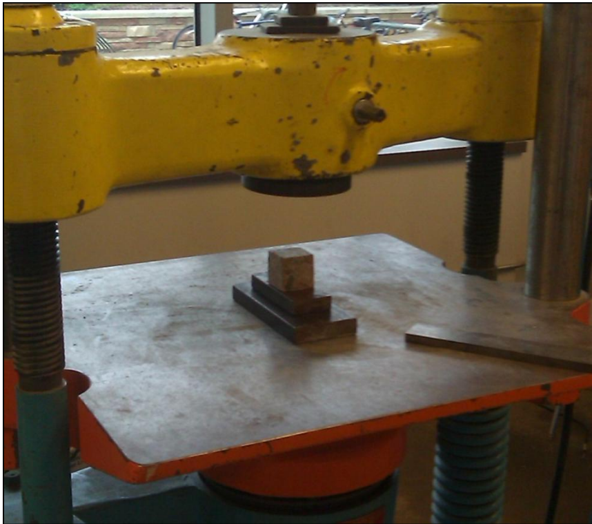
Figure 3.4 Compression test of the 2''x 2'' concrete cube.
