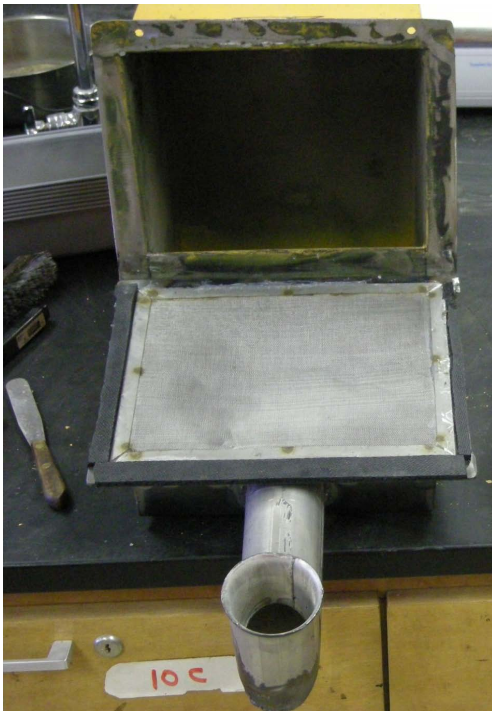
Figure 3.1 CSU Dustometer with Open Filter Box.
