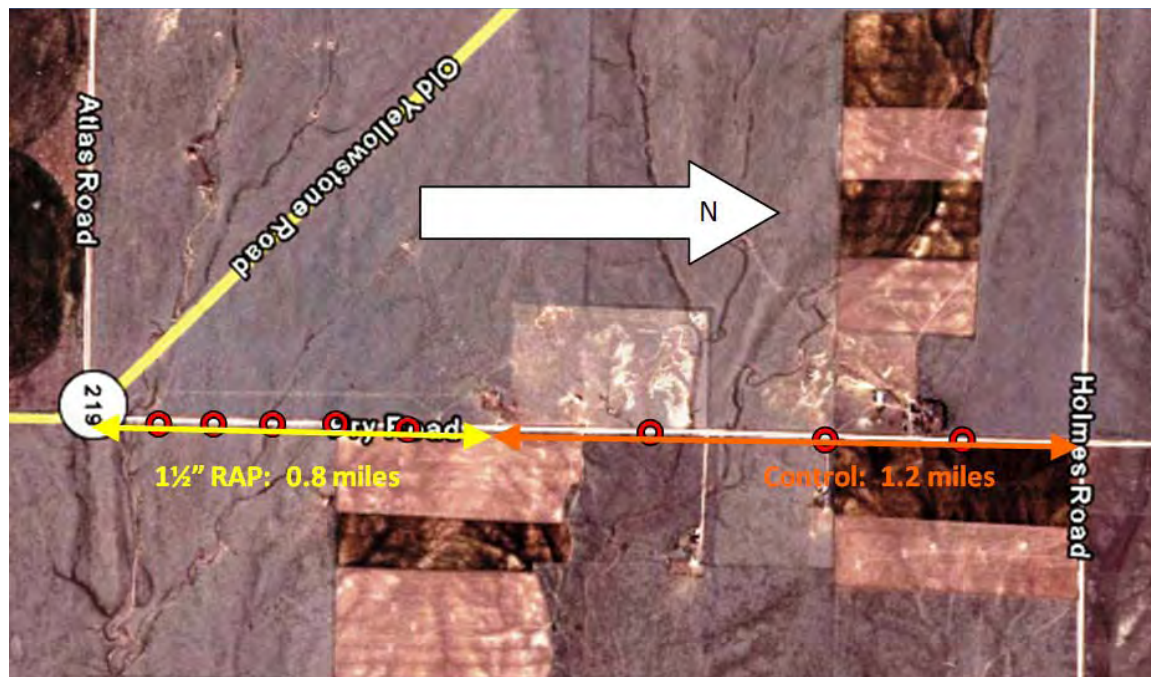
Figure 3.7 Test Sections on Pry Road.
