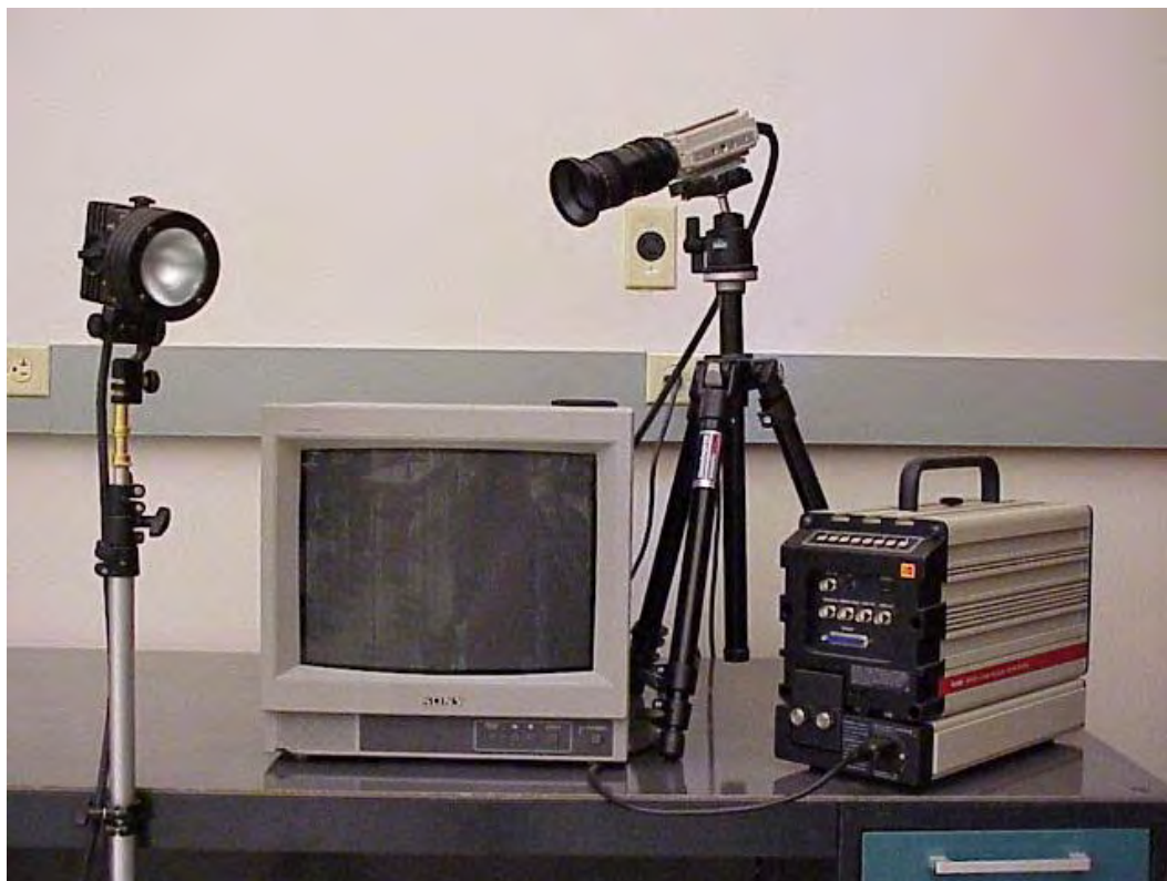
Figure 2.11 Kodak Motion Corder Analyzer PS-110 (Alciatore)
