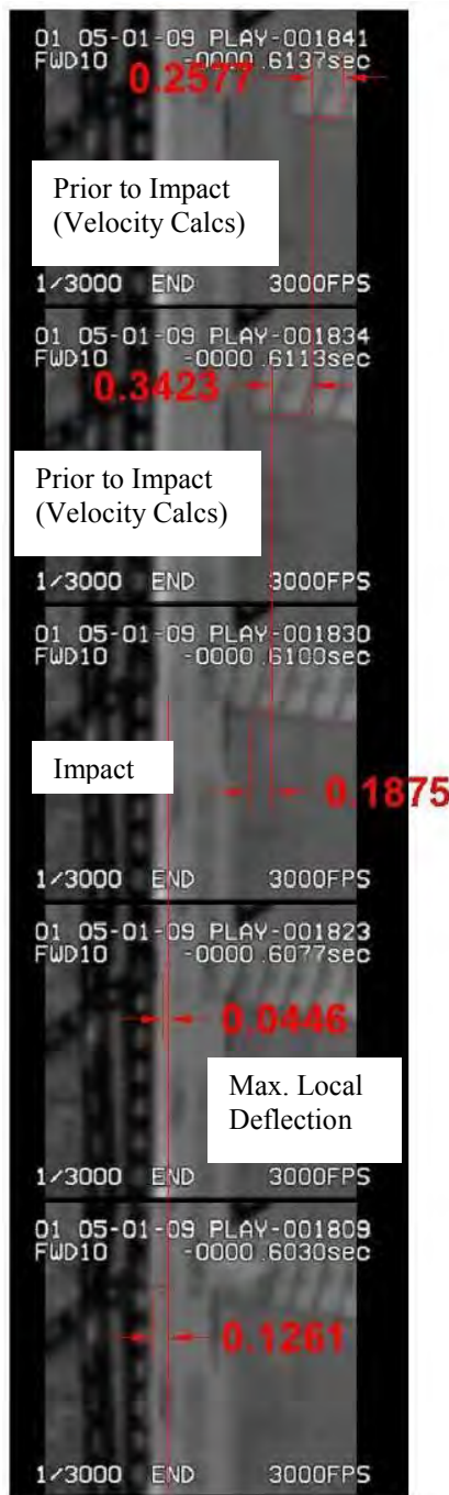
Figure 2.12 Impact Load Deflection Measurement
