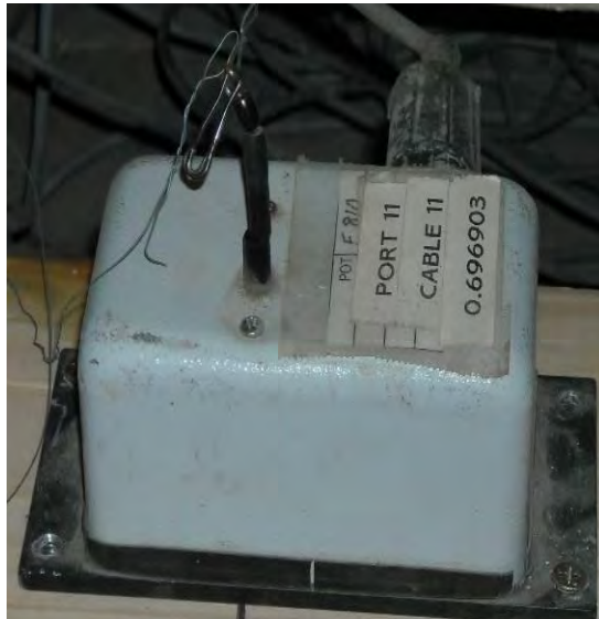
Figure 2.13 String Gauge Deflection Measurement
