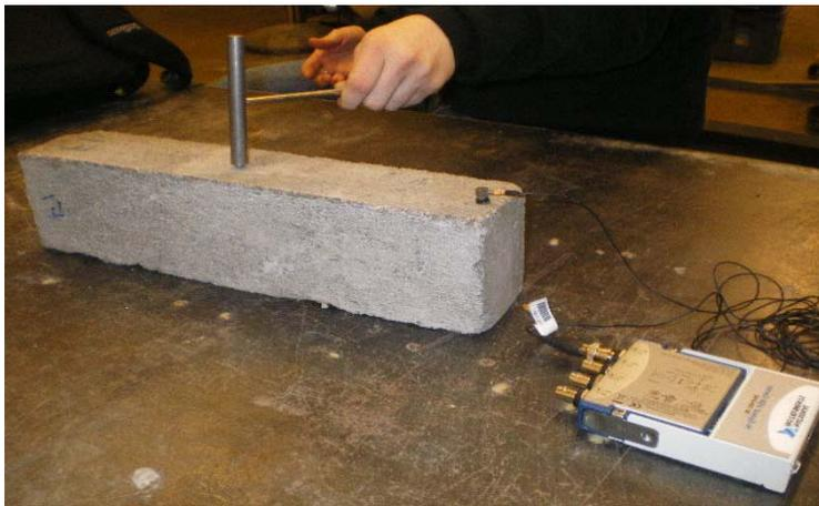
**Figure 3.7** Picture of Apparatus for Frequency Testing
