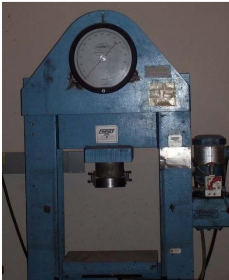
**Figure 3.1** Compression Testing Machine
