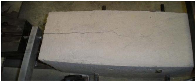
**Figure 4.5** Beam Loaded Indicating Shear Bond Failure
