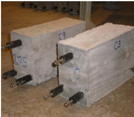
**Figure 3.10 a)** Corrosion Specimens
