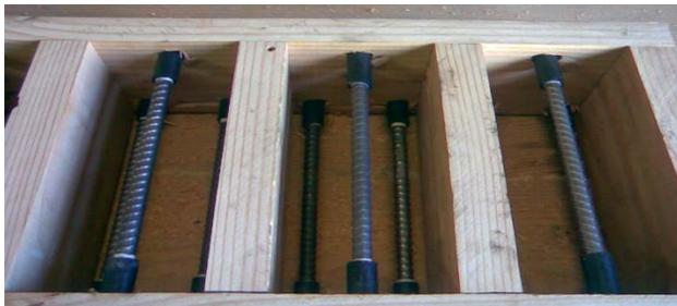
**Figure 3.9** Timber Forms and Rebar for Corrosion Specimens
