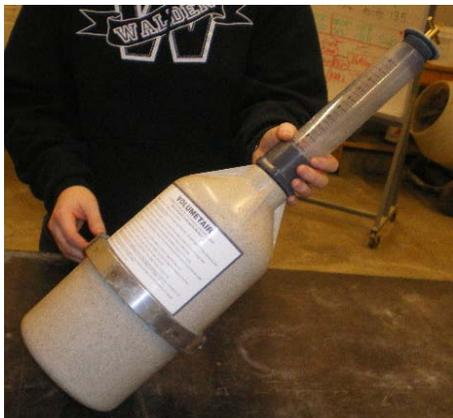
**Figure 3.4** Air Entrainment Testing Apparatus
