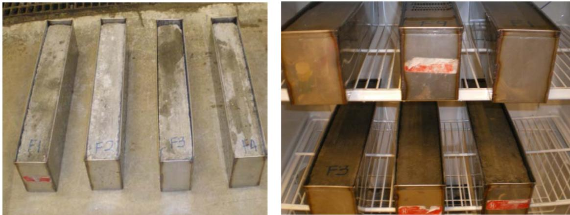
**Figure 3.5** Concrete Prisms for Freeze-thaw Testing
