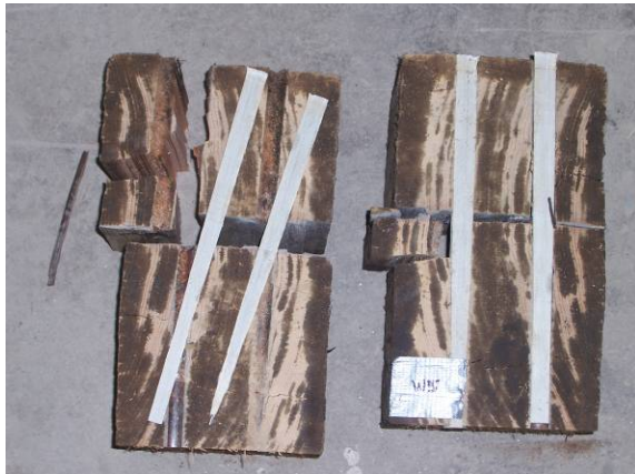
Figure 5.5 Spikes from Specimen 1 after failure (polyester resin)
