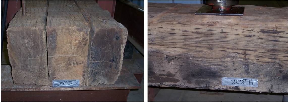
Figure 5.7 (left) Horizontal cracks visible on one end of Specimen 2. (right) No visible damage on the sides of the specimen.
