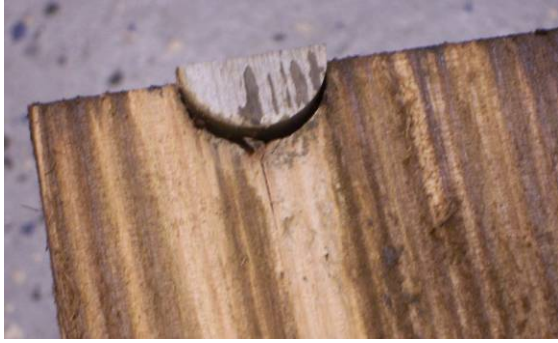
Figure 5.12 End view of dried polyester resin specimen
