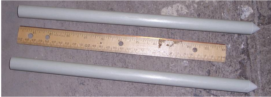
Figure 3.2 Spikes prepared for installation
