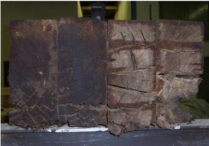
Figure 5.16 Damage to one end of Specimen 3
