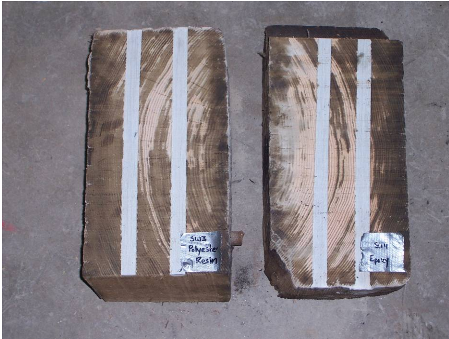
Figure 5.9 Spikes from Specimen 2. (polyester resin: left; epoxy resin: right)
