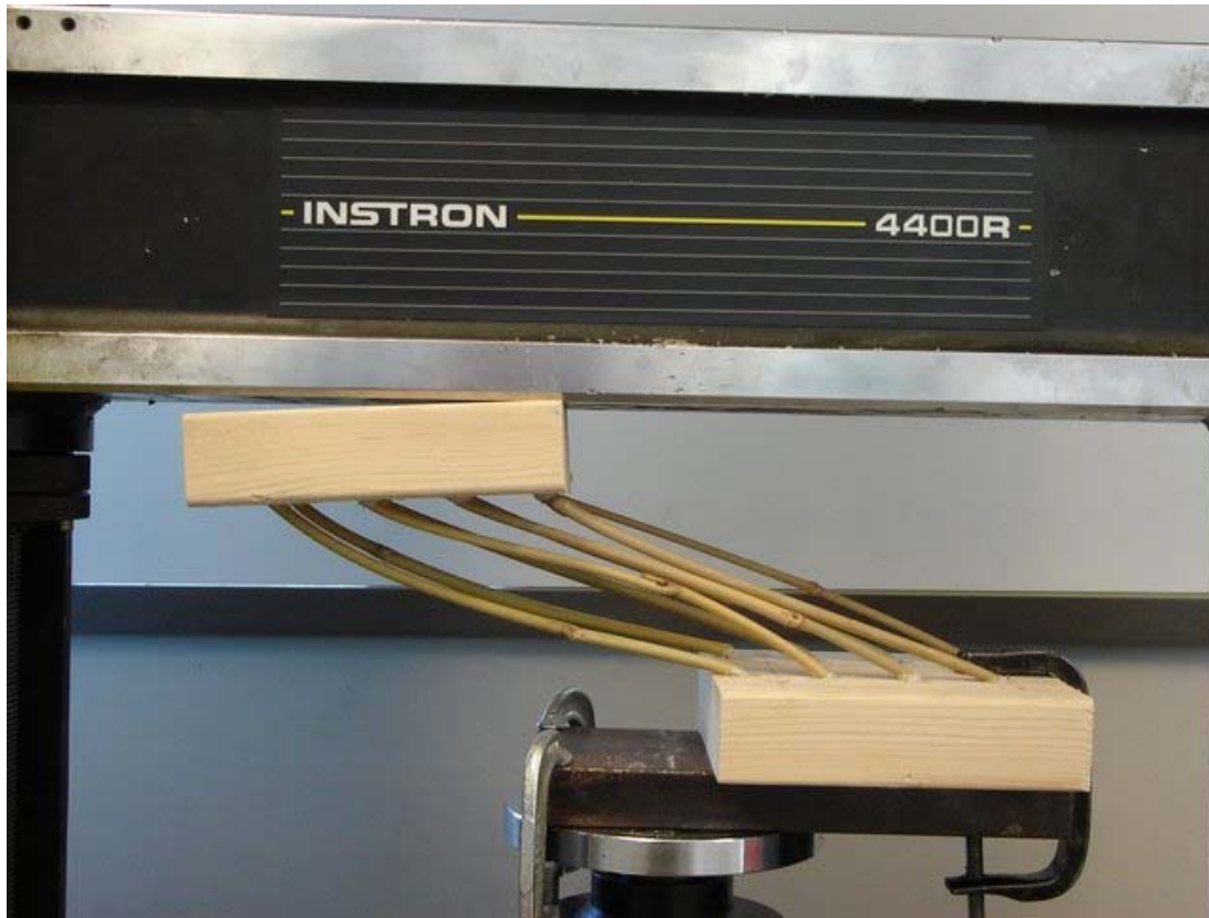
Figure 25 The bamboo model during testing
