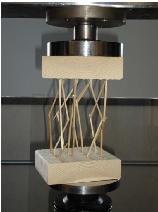
Figure 7 The 6", 12-dowel model during testing
