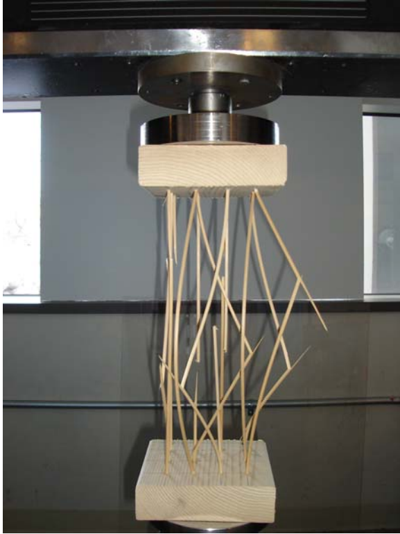
Figure 8 The 12", 12-dowel model during testing
