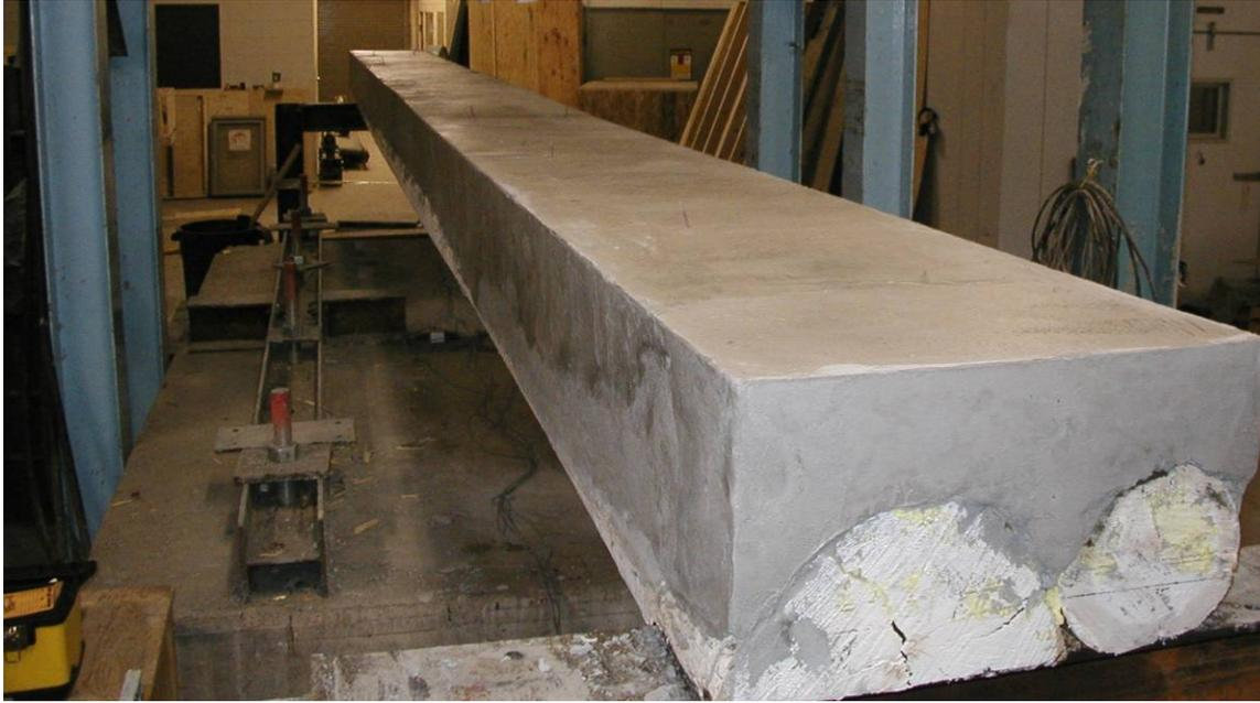
**Figure 3.20** Finished Wood-Concrete Beam
