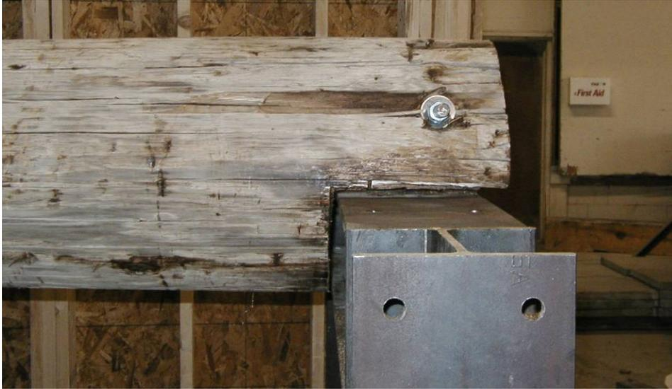
**Figure 3.3** Utility Pole with a 10-inch Notch Resting on Support
