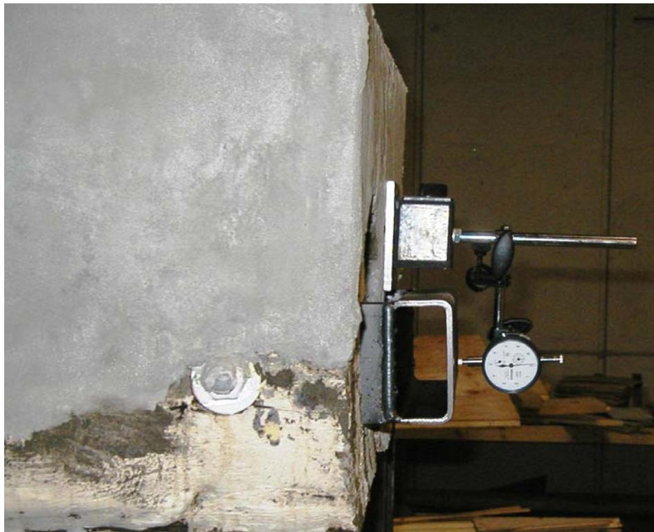
**Figure 3.23** Slip Measurement Fixture Side View
