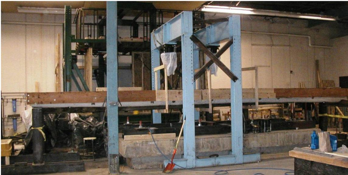
**Figure 3.19** Wood-Concrete Beam and Formwork
