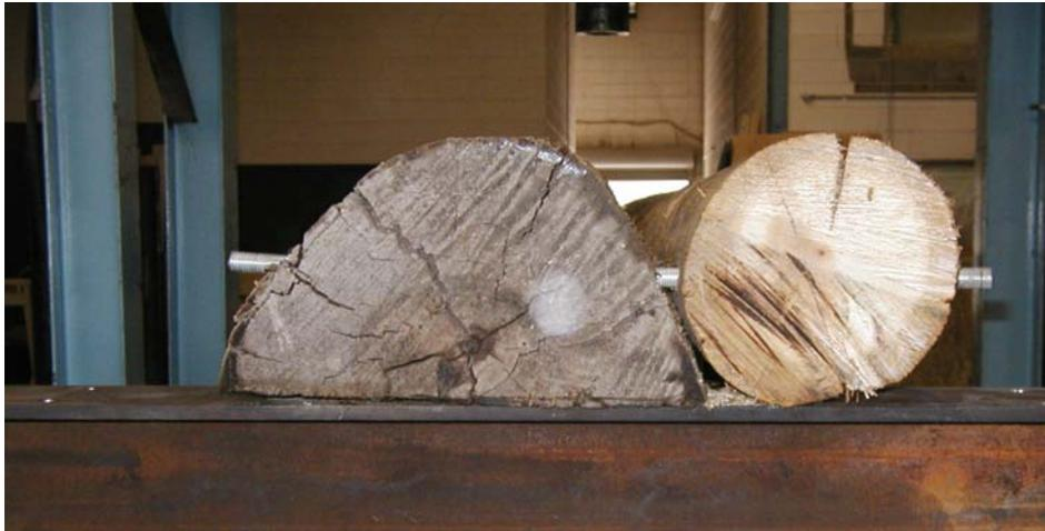
**Figure 3.2** Notch at the Support
