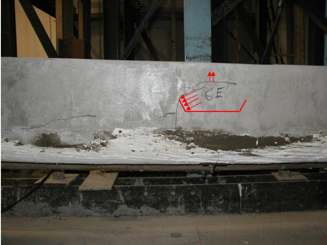
**Figure 4.5** Cracking on the Decompression Side of the Inner Notch – Beam 1
