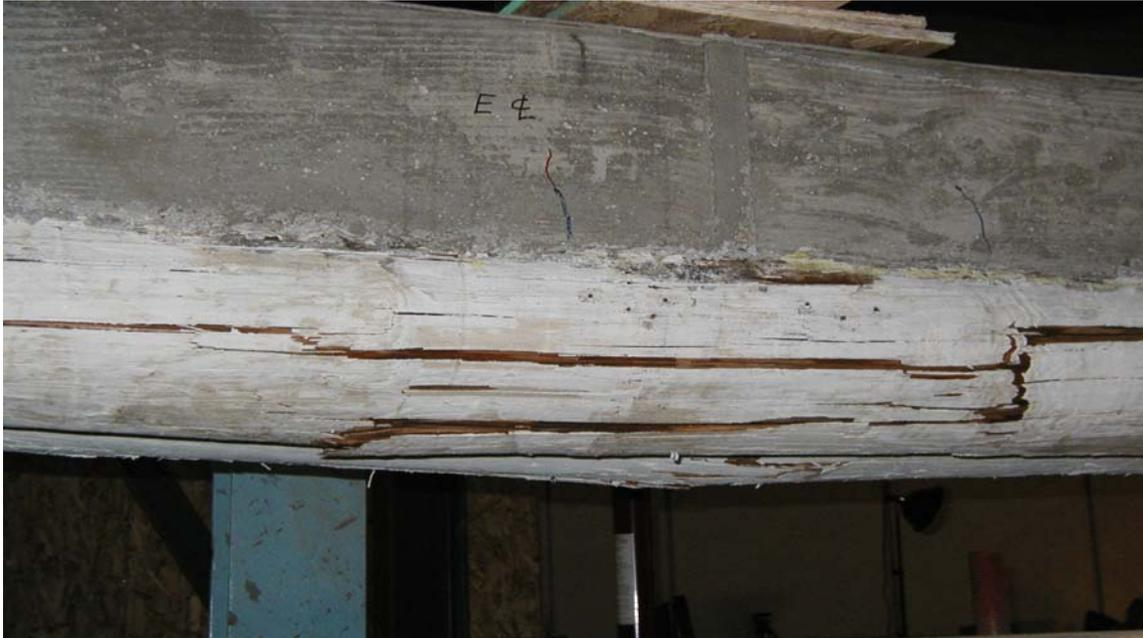
**Figure 4.16** Tear out of the Tension Face – Beam 2
