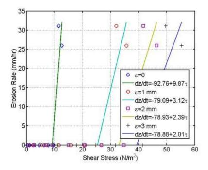
**Figure 6.2** Erosion rate versus shear stress curve for Big Sioux River Bridge; boring B-2 P-12, depth 29.5 to 31.5 ft, organic silt with abundant organic fibers.
