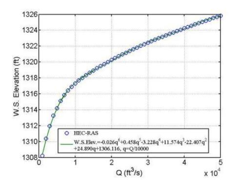
Figure 11.10 Rating curve for computed water surface elevation on upstream face of westbound bridge
