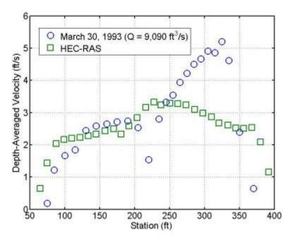
**Figure 7.13** Comparison of measured and computed flow velocities on upstream face of bridge for March 30, 1993. The pier sets are at 98 (bent 4), 219 (bent 3), and 338 (bent 2) ft from the left abutment.
