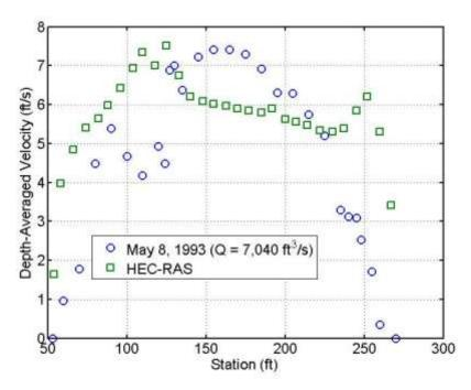
**Figure 9.12** Comparison of measured and computed approach flow velocities on upstream face of bridge for May 8, 1993. The pier sets are located at 128 ft (bent 2), 249 ft (bent 3), 345 ft (bent 4), and 389 ft (bent 5).
