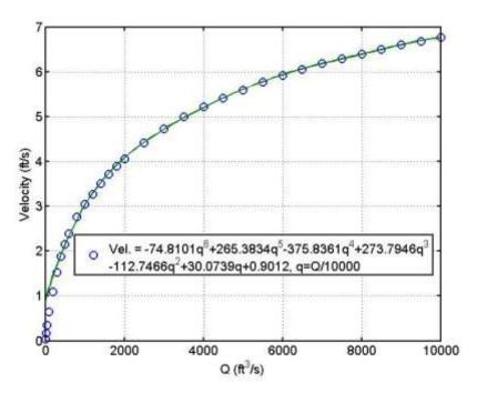
**Figure 9.18** Rating curve for computed approach flow velocity at bent 3 for n = 0.02
