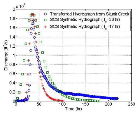
**Figure 8.24** Comparison of transferred hydrograph from Skunk Creek with Soil Conservation Service synthetic hydrographs for the May 8, 1993, flood.
