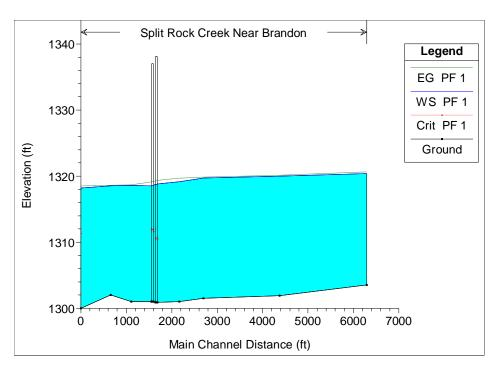
**Figure 8.9** Computed water surface profile at Split Rock Creek bridges for flow discharge of 14,700 ft<sup>3</sup>/s. The water depth downstream is normal depth.
