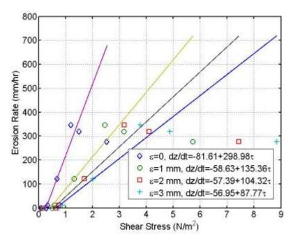
**Figure 6.12** Erosion rate versus shear stress curve for White River Bridge; boring B-10 P-7, depth 16.0 to 18.0 ft, slightly silty very sandy gravel.
