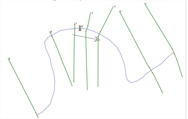
Figure 9.10 River schematic used in HEC-RAS computation
