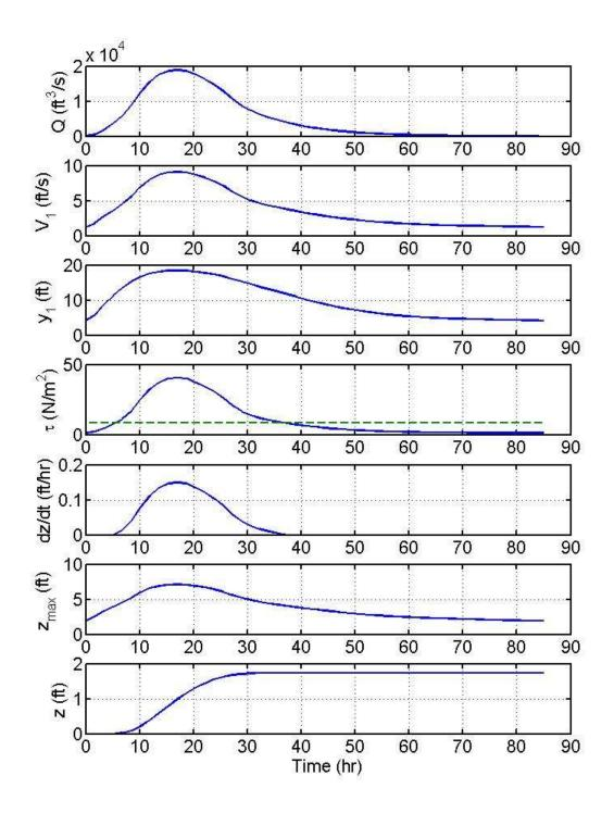
**Figure 8.25** SRICOS simulation for bent 3, May 8, 1993, flood using Soil Conservation Service synthetic hydrograph. The erosion rate versus shear stress curve is for clay with a roughness height of 0 mm. The critical shear stress  $\tau_c$  is shown as a dashed line in the initial bed shear stress plot.
