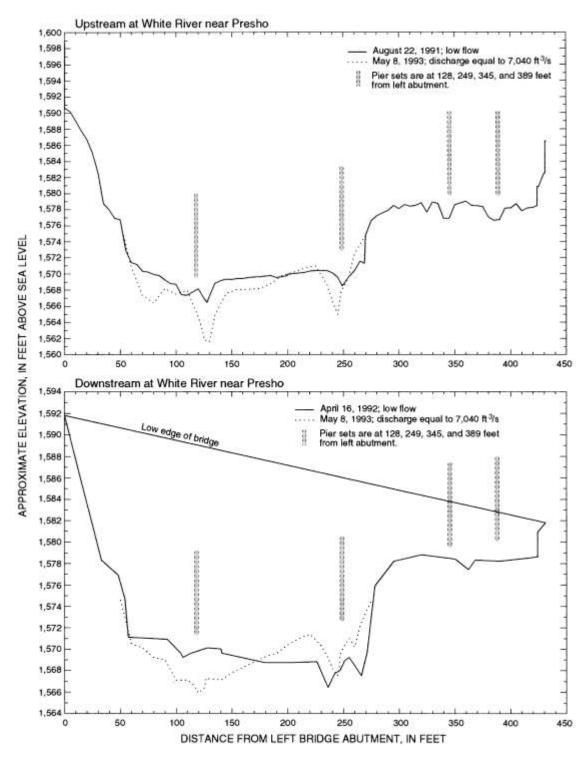
**Figure 9.9** Upstream and downstream cross sections at White River Bridge near Presho (after Niehus 1996). The pier centerline stations are 128 ft (bent 2), 249 ft (bent 3), 345 ft (bent 4), and 389 ft (bent 5) from the left abutment.
