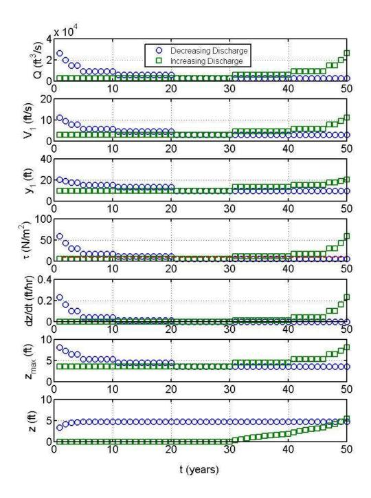
**Figure 11.5** SRICOS simulation for bent 3 at Split Rock Creek bridges, westbound, for two sequences of maximum annual floods arranged in ascending and descending orders. The values of the basic input parameters are given in Table 8.4 for the baseline conditions. The critical shear stress is shown as a dashed line in the initial bed shear stress plot.
