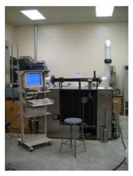
Figure 6.19 Minnesota Department of Transportation erosion function apparatus
