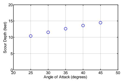
**Figure 10.4** Pier scour while varying the angle of attack (Sensitivity Ranking = 2)
