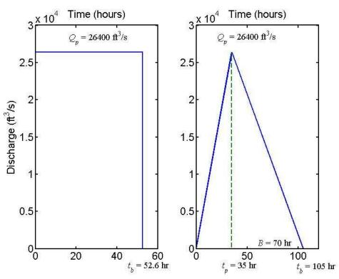
Figure 11.16 Rectangular and triangular hydrographs used in SRICOS simulations
