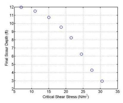
Figure 7.24 Effect of critical shear stress on predicted final scour depth at bent 2
