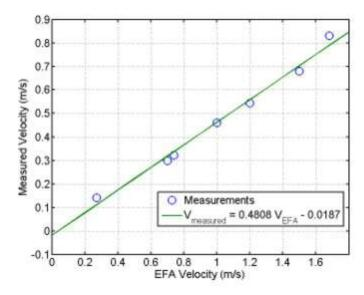
Figure 6.18 Velocity correction for erosion function apparatus
