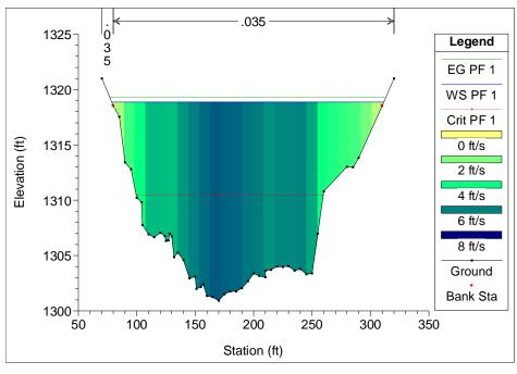
Figure 8.11 Bridge section upstream (River Station 4). Same discharge as in Figure 8.10.
