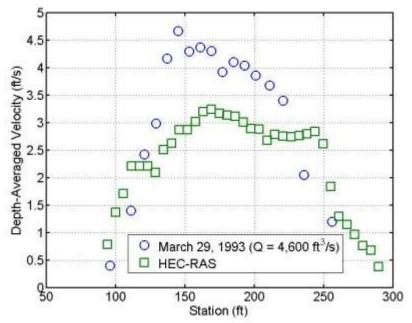
**Figure 8.12** Comparison of measured and computed approach flow velocities on upstream face of westbound bridge for March 29, 1993. The pier sets are at 53 ft (bent 5), 105 ft (bent 4), 175 ft (bent 3), and 264 ft (bent 2) from the left abutment.
