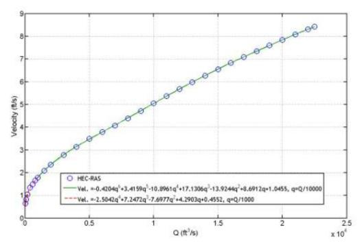
**Figure 8.15** Rating curve for computed approach flow velocity at bent 3 on upstream face of westbound bridge
