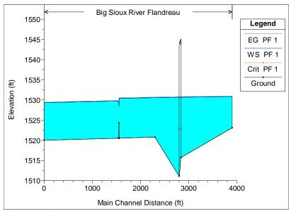
**Figure 7.10** Computed water surface profile at Big Sioux River Bridge for flow discharge of 9,090 ft<sup>3</sup>/s. The water depth downstream is normal depth.
