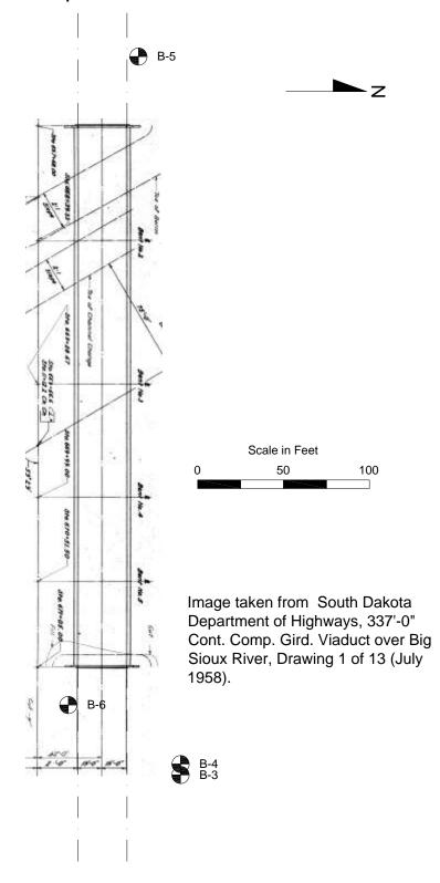
Figure 5.4 Site and exploration plan for the Split Rock Creek study site
