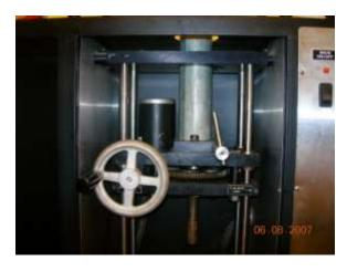
**Figure 2.1** Erosion Function Apparatus. Top plot—water tunnel and observation window; a thin wall tube is mounted perpendicular to the water tunnel. Bottom plot—stepping motor and piston assembly.
