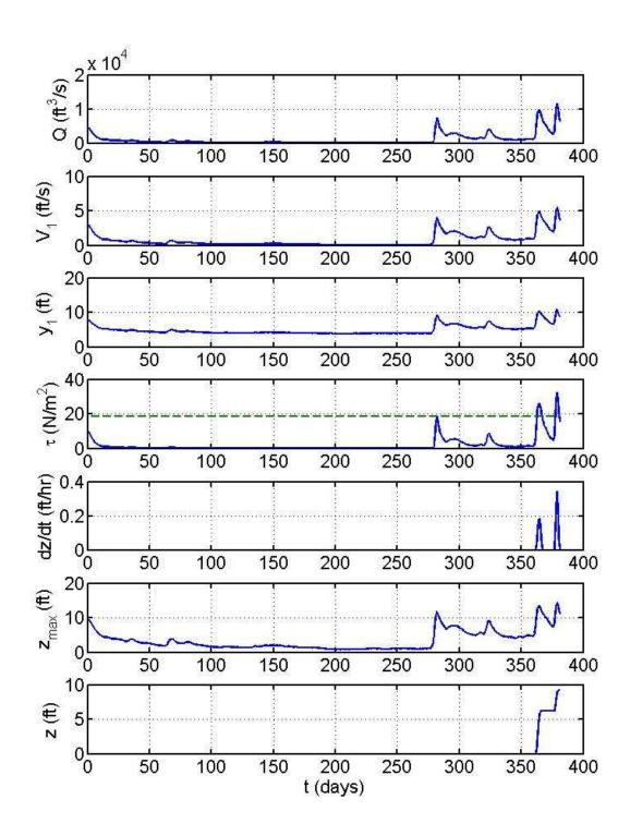
**Figure 7.19** SRICOS simulation for bent 2, June 22, 1992, through July 7, 1993; baseline conditions. The discharge is daily mean flow. The critical shear stress  $\tau_c$  is shown as a dashed line in the initial bed shear stress plot.
