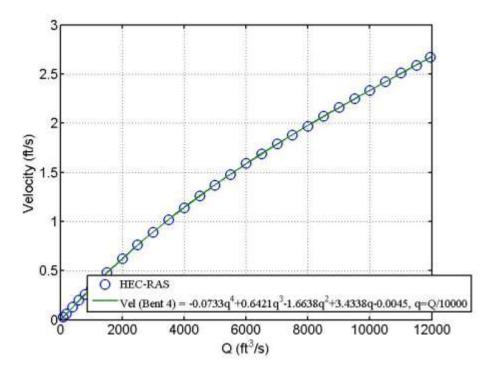
Figure 7.17 Rating curve for computed approach flow velocity at bent 4
