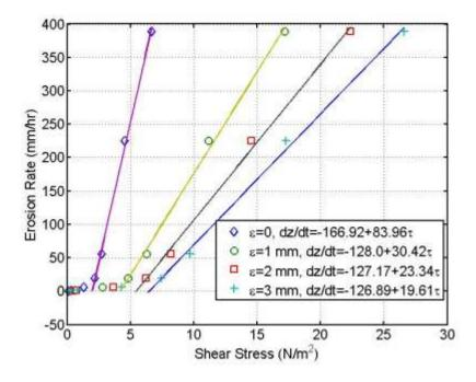
**Figure 6.15** Erosion rate versus shear stress curve for boring B-9 P-1, depth 24.0 to 26.0 ft. The data from TAMU are re-plotted for four different roughness heights.
