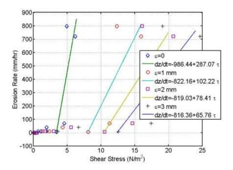
**Figure 6.5** Erosion rate versus shear stress curve for Split Rock Creek bridges; boring B-5 P-10, depth 20.0 to 22.0 ft, slightly silty gravelly sand to slightly gravelly medium sand.
