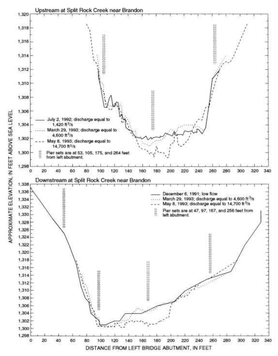
**Figure 8.7** Upstream and downstream cross sections at the Split Rock Creek bridges near Brandon. The ordinate is distance from the left abutment and the abscissa is elevation above mean sea level, in feet (after Niehus 1996). At both bridges, the largest scour depth was found around bent 3 in the main channel.
