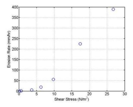
**Figure 6.13** Erosion rate versus shear stress curve from TAMU; boring B-9 P-1, depth 24.0 to 26.0 ft (corresponding to B-7 P-10)
