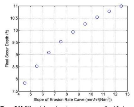
Figure 7.25 Effect of slope of erosion rate curve on predicted final scour depth at bent 2
