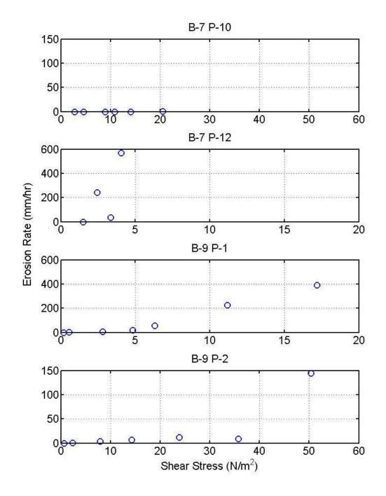
**Figure 6.17** Comparison of measured erosion rate versus shear stress curves from SDSU (borings B-7 P-10 and B-7 P-12) and TAMU (B-9 P-1 and B-9 P-2) for  $\epsilon$  = 1 mm
