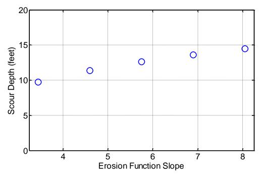
**Figure 10.1** Pier scour while varying the erosion function slope (Sensitivity Ranking = 3)
