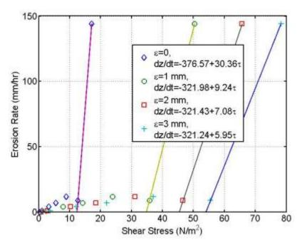
**Figure 6.16** Erosion rate versus shear stress curve for boring B-9 P-2, depth 29.0 to 31.0 ft. The data from TAMU are re-plotted for four different roughness heights.
