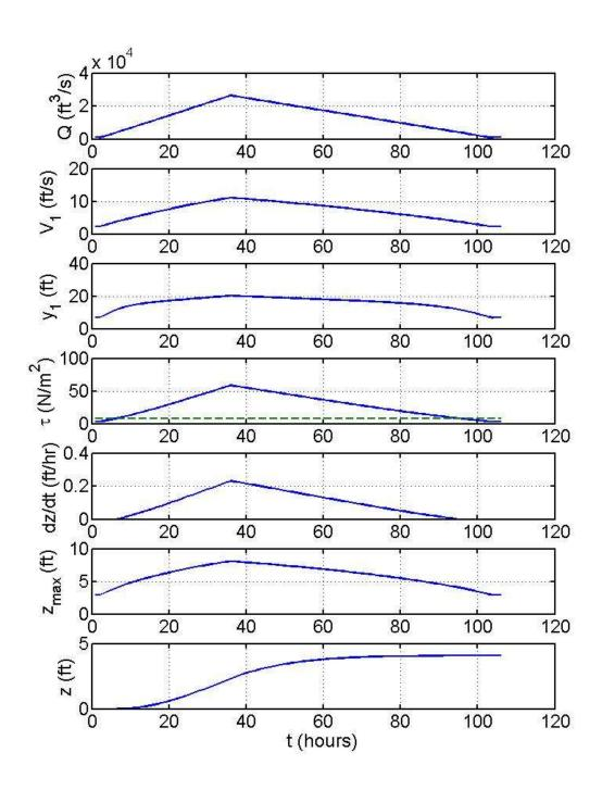
**Figure 11.18** SRICOS simulation for bent 3 at the Split Rock Creek westbound bridge using a triangular hydrograph for a peak flow of 26,400 ft<sup>3</sup>/s and time base of 105 hr. The values of the other input parameters are given in Table 8.4. The critical shear stress is shown as a dashed line in the initial bed shear stress plot.
