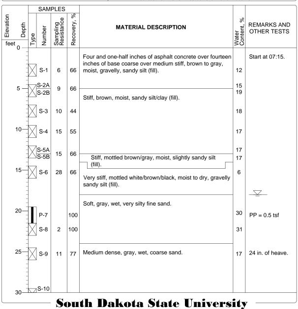
Figure 5.6 Log of boring B-1
