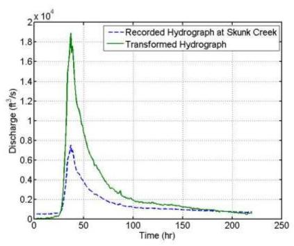
**Figure 8.18** Recorded hydrograph from Skunk Creek at Sioux Falls gauging station and transformed hydrograph for the Split Rock Creek site (May 6 through May 15, 1993)
