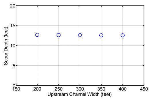
**Figure 10.3** Pier scour while varying the upstream channel width (Sensitivity Ranking = 7)
