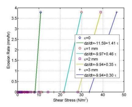
**Figure 6.4** Erosion rate versus shear stress curve for Split Rock Creek bridges; boring B-4 P-2, depth 20.0 to 22.0 ft, clay.
