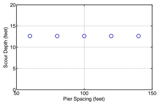
**Figure 10.5** Pier scour while varying the pier spacing (Sensitivity Ranking = 9)
