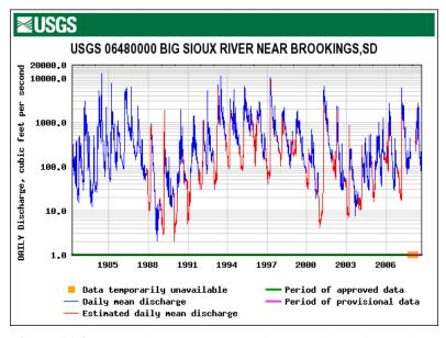
**Figure 11.2** Recorded hydrograph (daily mean flow) from Big Sioux River near Brookings gauging station from 1982 to 2008
