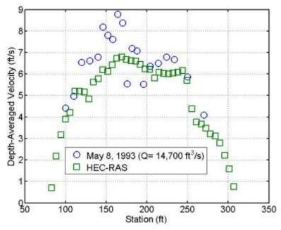
**Figure 8.13** Comparison of measured and computed approach flow velocities on upstream face of westbound bridge for May 8, 1993. Locations of pier sets are the same as in Figure 8.12.
