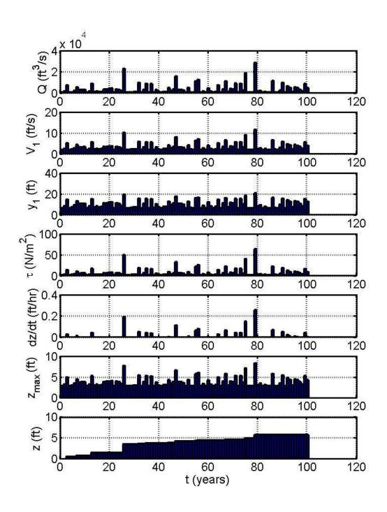
**Figure 11.13** SRICOS simulation for bent 3 at Split Rock Creek bridges, westbound, for one series (trial 3) of maximum annual floods for a period 100 years. The values of the basic input parameters are given in Table 8.4 for the baseline conditions.
