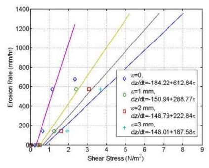
**Figure 6.11** Erosion rate versus shear stress curve for White River Bridge; boring B-10 P-5, depth 12.0 to 14.0 ft, very silty fine sand
