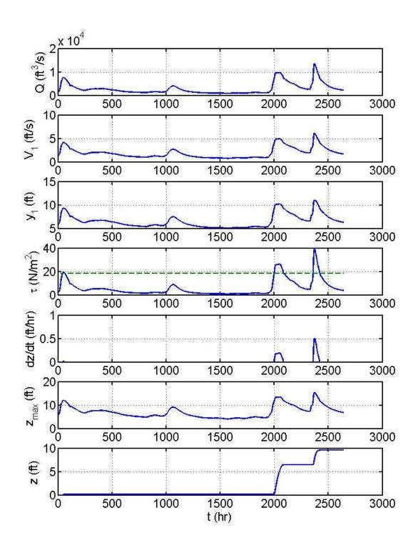
**Figure 7.20** SRICOS simulation for bent 2, March 28 to July 7, 1993; baseline conditions. The discharge is hourly mean flow.
