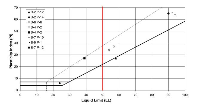
Figure 5.23 Laboratory testing results for atterberg limit testing
