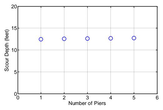
**Figure 10.6** Pier scour while varying the number of piers (Sensitivity Ranking = 7)
