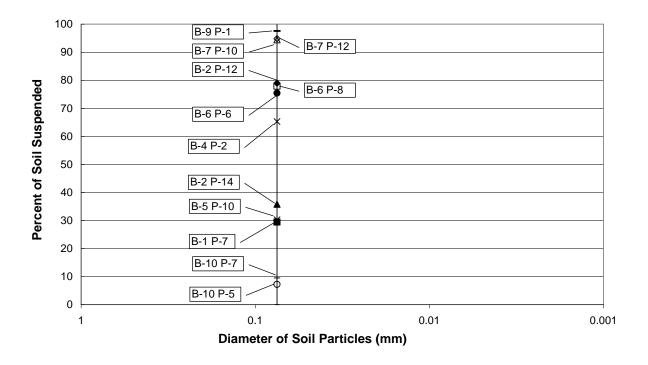
Figure 5.25 Laboratory testing results for No. 200 wash analysis
