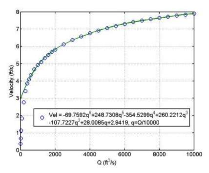
**Figure 9.16** Rating curve for computed approach flow velocity at bent 2 for n = 0.02
