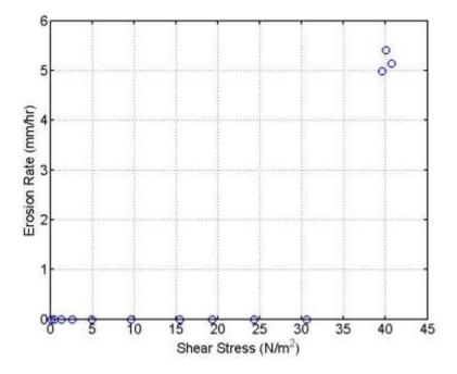
**Figure 6.8** Erosion rate versus shear stress curve for Split Rock Creek bridges; boring B-6 P-8, depth 18.0 to 20.0 ft, very silty fine sand. The bed shear stress is for  $\varepsilon = 1$  mm.
