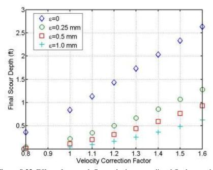
Figure 8.23 Effect of approach flow velocity on predicted final scour depth at bent 3
