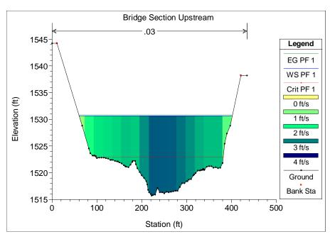
**Figure 7.12** Bridge section upstream. The computed water surface elevation and velocity distribution are for a discharge of 9,090 ft<sup>3</sup>/s.
