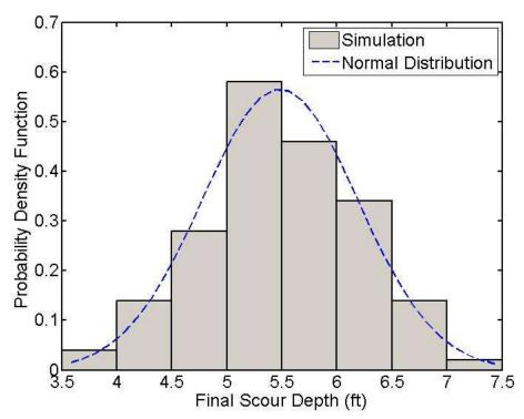
**Figure 11.14** Probability distribution of predicted final scour depth from 100 SRICOS simulations. The final scour depth is compared to a normal distribution. The mean and standard deviation of the predicted final scour depths are 5.48 ft and 0.71 ft, respectively.
