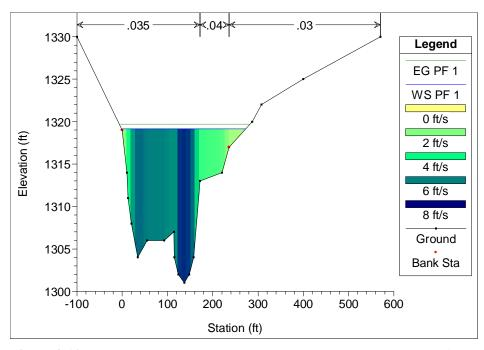
**Figure 8.10** Approach section (River Station 5). The computed water surface elevation and velocity distribution are for a discharge of 14,700 ft<sup>3</sup>/s.
