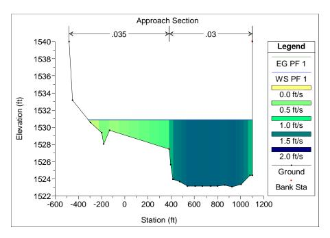
**Figure 7.11** Approach section in HEC-RAS. The computed water surface elevation and velocity distribution are for a discharge of 9,090 ft<sup>3</sup>/s.
