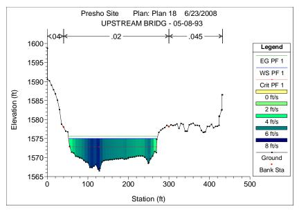
**Figure 9.13** Cross section plot at River Station 6 on upstream face of bridge showing measured ground elevation, computed water surface elevation, and computed flow velocity distribution for a discharge of 7,040 ft<sup>3</sup>/s.
