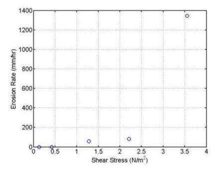
**Figure 6.6** Erosion rate versus shear stress curve for Split Rock Creek bridges; boring B-5 P-12, depth 23.5 to 25.5 ft, gravelly medium sand to slightly sandy gravel. The bed shear stress is for  $\varepsilon = 1$  mm.
