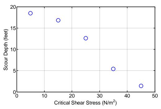
**Figure 10.2** Pier scour while varying the critical shear stress (Sensitivity Ranking = 1)
