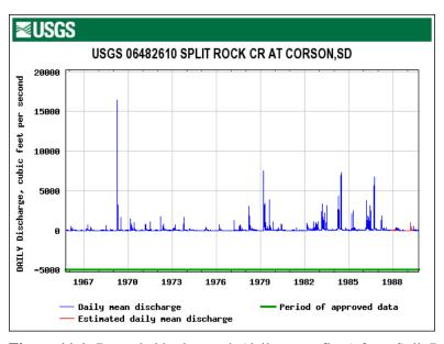
**Figure 11.1** Recorded hydrograph (daily mean flow) from Split Rock Creek at Corson gauging station from 1965 to 1989
