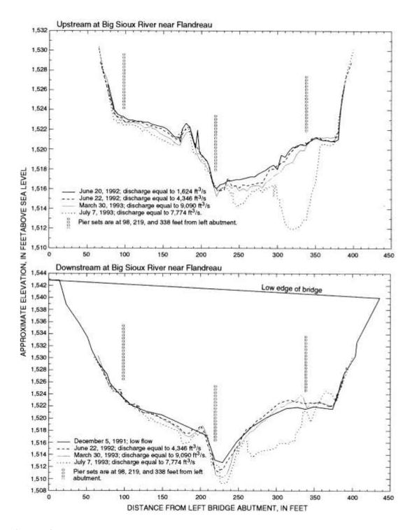
**Figure 7.8** Upstream and downstream cross sections at the Big Sioux River Bridge near Flandreau. The ordinate for the upstream and downstream cross sections is the distance from the left abutment and the abscissa is elevation above mean sea level, in feet (after Niehus 1996).
