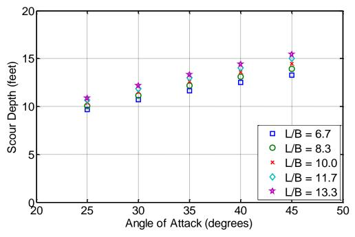
Figure 10.9 Pier scour while varying the flow angle of attack and L/B (Sensitivity Ranking = 4)
