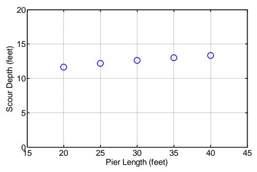
**Figure 10.7** Pier scour while varying the pier length (Sensitivity Ranking = 5)
