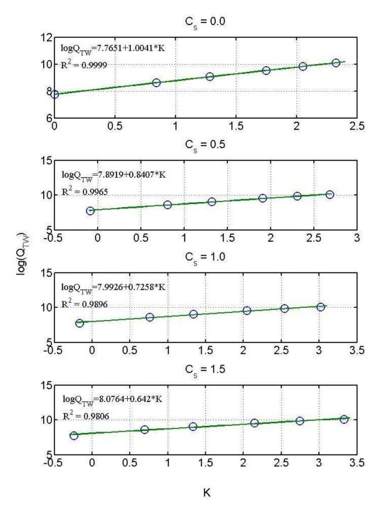
**Figure 11.8** Variation of  $\log(Q_{TW})$  with K for skew coefficient of 0.0, 0.5, 1.0, and 1.5 for Split Rock Creek bridges
