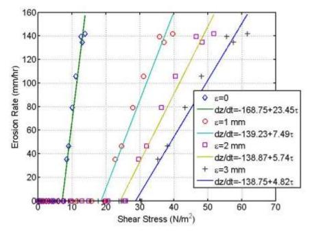
**Figure 2.2** Erosion rate versus shear stress curve for Big Sioux River Bridge; boring B-1 P-7, depth 19.5 to 21.5 ft., very silty fine sand. The applied shear stress has been calculated using four different values of bed roughness height ( $\varepsilon = 0$ , 1, 2. and 3 mm). Note that the critical shear stress and slope of the erosion rate curve vary considerably with the roughness height assumed.
