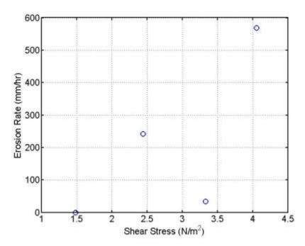
**Figure 6.10** Erosion rate versus shear stress curve for White River Bridge; boring B-7 P-12, depth 29.0 to 31.0 ft, silty sandy gravel. The bed shear stress is for  $\varepsilon = 1$  mm.
