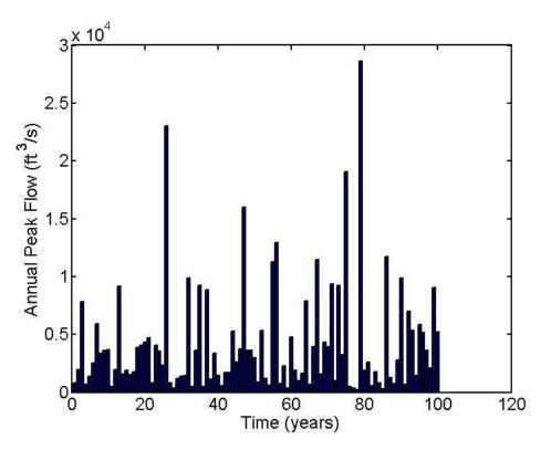
Figure 11.9Constructed hydrograph for maximum annual floods for Split Rock Creek bridges; trial 3
