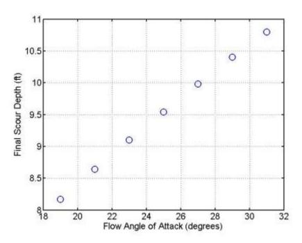
Figure 7.22 Effect of flow angle of attack on predicted final scour depth at bent 2
