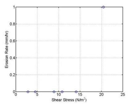
**Figure 6.9** Erosion rate versus shear stress curve for White River Bridge; boring B-7 P-10, depth 24.0 to 26.0 ft, silt. The bed shear stress is for  $\varepsilon = 1$  mm.
