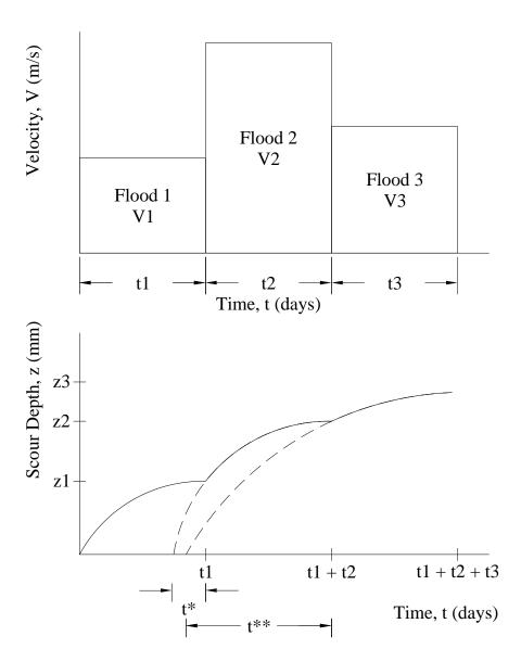
Figure 2.3 Scour due to a sequence of three flooding events.
