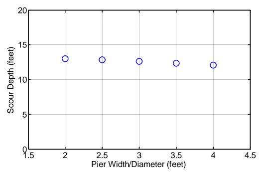
**Figure 10.8** Pier scour while varying the pier width or diameter (Sensitivity Ranking = 6)
