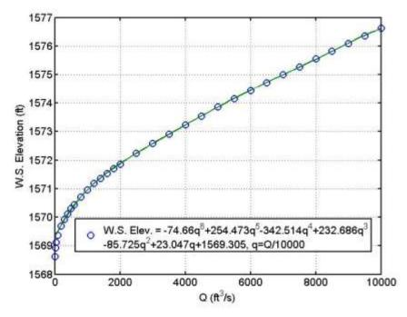
**Figure 9.14** Rating curve for computed water surface elevation on upstream face of bridge for n = 0.02 in the main channel.
