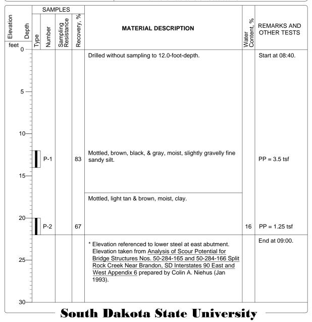
Figure 5.11 Log of boring B-4
