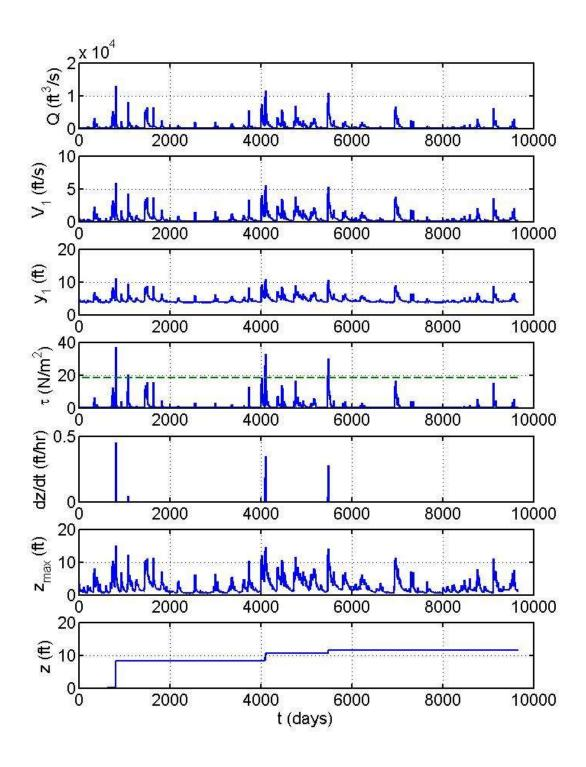
**Figure 11.4** SRICOS simulation for bent 2 at Big Sioux River Bridge from April 1, 1982, to September 11, 2008. The values of other input parameters are given in Table 7.3 for the baseline conditions. The critical shear stress is shown as a dashed line in the initial bed shear stress plot.
