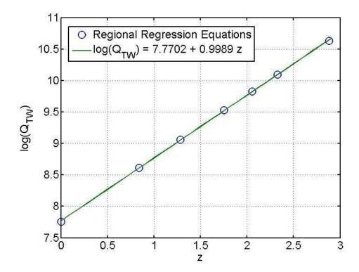
**Figure 11.7** Variation of log  $(Q_{TW})$  with z for Split Rock Creek bridges
