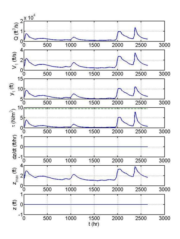
**Figure 7.21** SRICOS simulation for bent 4, March 28 to July 7, 1993; baseline conditions. The discharge is hourly mean flow.
