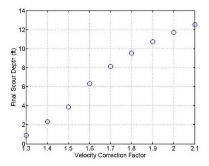
Figure 7.23 Effect of approach flow velocity on predicted final scour depth at bent 2
