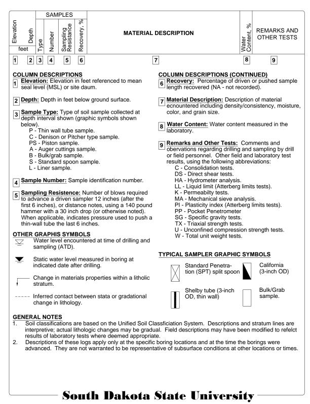
**Figure 5.1** Key to exploration logs
