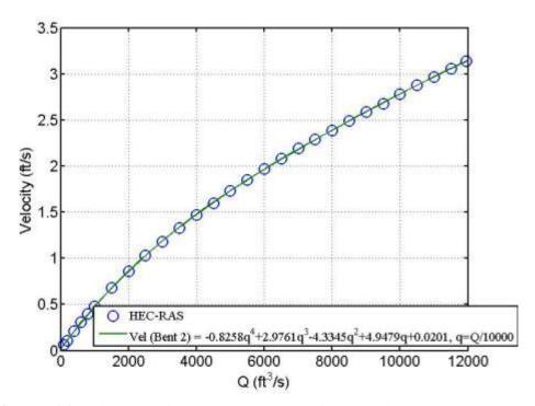
Figure 7.16 Rating curve for computed approach flow velocity at bent 2
