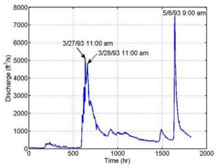
**Figure 8.17** Hourly mean flow data from Skunk Creek at Sioux Falls gauging station for March 1, 1993, through May 15, 1993
