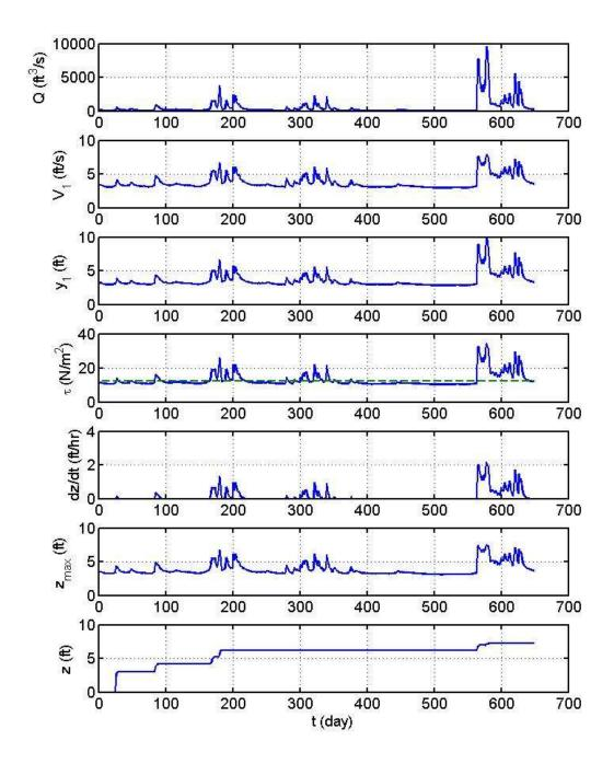
Figure 9.21 SRICOS simulation for bent 2, August 22, 1991, through May 31, 1993. The discharge is daily mean flow. The erosion rate versus shear stress curve is from Figure 6.16 (boring B-9 P-2) with  $\epsilon=0$  which corresponds to a critical shear stress of 12.4 N/m² and slope of erosion rate versus shear stress curve of 30.36 mm/hr/(N/m²). The critical shear stress  $\tau_c$  is shown as a dashed line in the initial bed shear stress plot.
