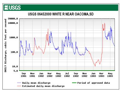
**Figure 9.20** Daily mean discharge from White River near Oacoma streamflow gauging station for August 1, 1991, through May 31, 1993.
