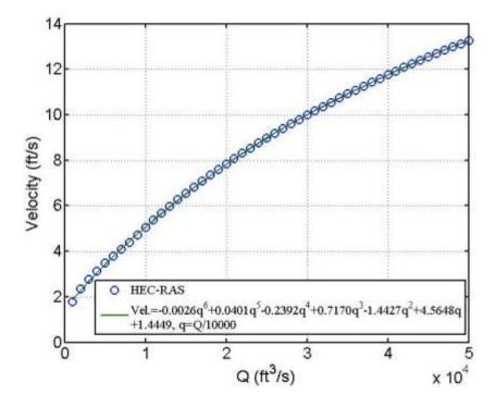
Figure 11.11 Rating curve for approach flow velocity at bent 3 on upstream face of westbound bridge
