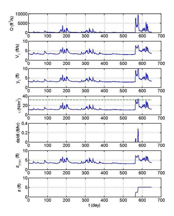
**Figure 9.22** SRICOS simulation for bent 2, August 22, 1991, through May 31, 1993. The discharge is daily mean flow. The critical shear stress is  $31.5 \text{ N/m}^2$  and the slope of erosion rate versus shear stress curve is  $30.36 \text{ mm/hr/(N/m}^2)$ . The critical shear stress  $\tau_c$  is shown as a dashed line in the initial bed shear stress plot.
