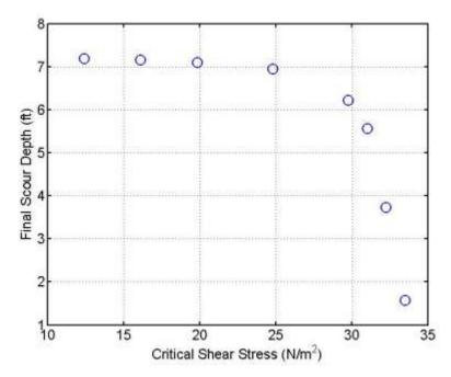
**Figure 9.24** Effect of critical shear stress on predicted final scour depth for bent 2. The slope of the erosion rate versus shear stress curve is kept fixed at 30.36 mm/hr/(N/m<sup>2</sup>).
