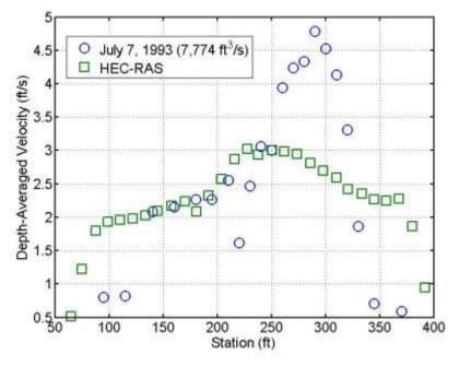
**Figure 7.14** Comparison of measured and computed flow velocities on upstream face of bridge for July 7, 1993. The pier sets are at 98 (bent 4), 219 (bent 3), and 338 (bent 2) ft from the left abutment.
