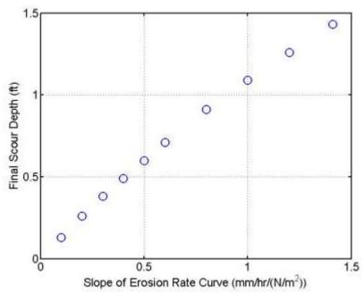
Figure 8.22 Effect of slope of erosion rate curve on predicted final scour depth at bent 3
