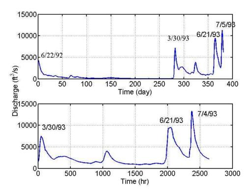
**Figure 7.18** Hydrographs from Big Sioux River near Brookings streamflow gauging station. The upper plot is the daily mean flow from June 22, 1992, to July 7, 1993. The lower plot is the hourly mean flow from March 28, 1993, to July 7, 1993. The measured discharges shown were multiplied by 1.025 in the SRICOS simulation to account for the increase in drainage area between the Brookings station and the bridge site.
