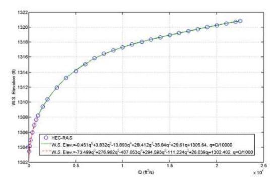
Figure 8.14 Rating curve for computed water surface elevation on upstream face of westbound bridge
