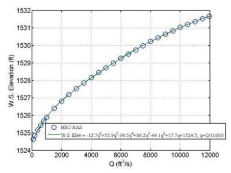
**Figure 7.15** Rating curve for computed water surface elevation on upstream face of Big Sioux River Bridge
