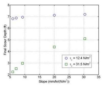
**Figure 9.25** Effect of slope of erosion rate versus shear stress curve on predicted final scour depth for bent 2
