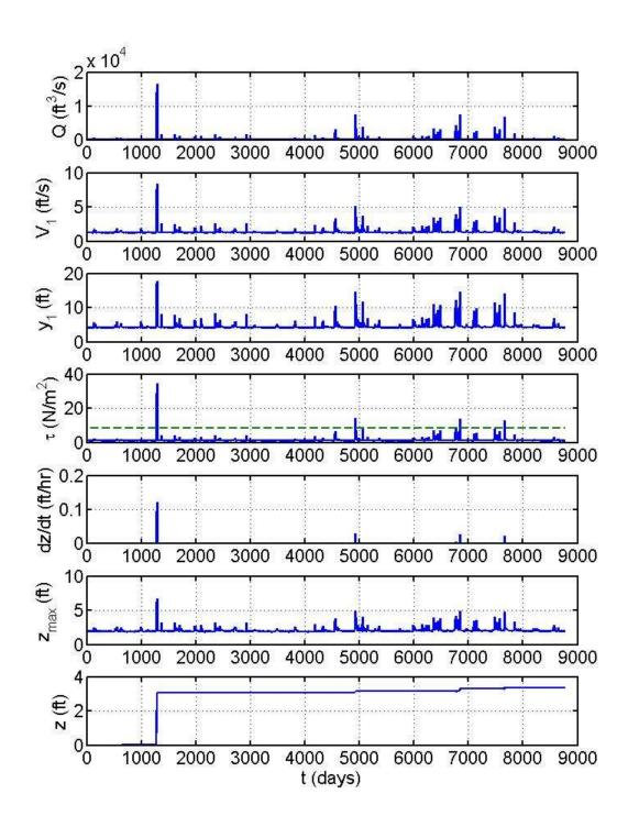
**Figure 11.3** SRICOS simulation for bent 3 at Split Rock Creek bridges, westbound, from October 1, 1965, to September 30, 1989. The values of other input parameters are given in Table 8.4 for the baseline conditions. The critical shear stress is shown as a dashed line in the initial bed shear stress plot.
