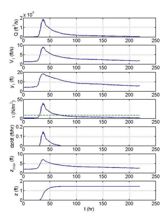
**Figure 8.19** SRICOS simulation for bent 3, May 6 through May 15, 1993; baseline conditions. The discharge is hourly mean flow. The erosion rate curve is for clay with a roughness height of 0 mm. The critical shear stress  $\tau_c$  is shown as a dashed line in the initial bed shear stress plot.
