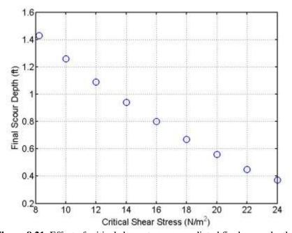
**Figure 8.21** Effect of critical shear stress on predicted final scour depth at bent 3
