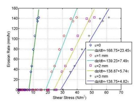
**Figure 6.1** Erosion rate versus shear stress curve for Big Sioux River Bridge; boring B-1 P-7, depth 19.5 to 21.5 ft, very silty fine sand, tests 1 and 2
