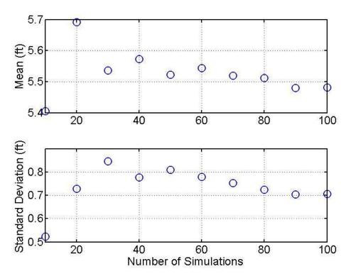
**Figure 11.15** Mean and standard deviation of predicted final scour depth calculated using increasing number of simulations
