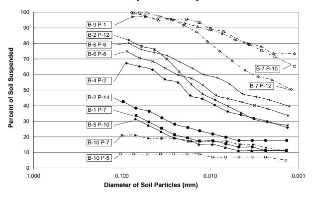
Figure 5.24 Laboratory testing results for hydrometer analysis testing
