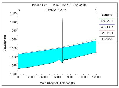
**Figure 9.11** Computed water surface profile for  $Q = 7,040 \text{ ft}^3/\text{s}$  and n = 0.02 (main channel). The channel cross section and slope are nearly uniform downstream of the bridge crossing.
