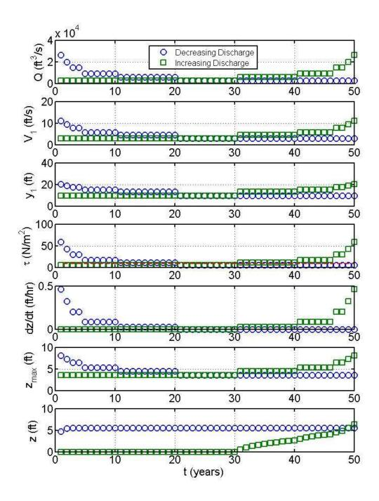
**Figure 11.6** SRICOS simulation for bent 3 at Split Rock Creek bridges, westbound, for two sequences of maximum annual floods arranged in ascending and descending orders. The input parameters are the same as in Figure 11.5 except that the slope of the erosion rate versus shear stress curve has been increased from 1.41 to 2.82 mm/hr/(N/m²). The critical shear stress is shown as a dashed line in the initial bed shear stress plot.
