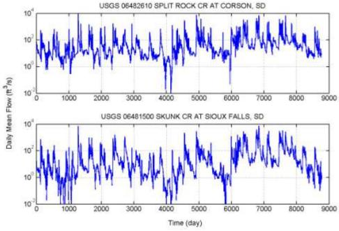
**Figure 8.16** Daily mean flow data from Split Rock Creek near Corson and Skunk Creek at Sioux Falls gauging stations for January 1, 1965, through December 31, 1989.
