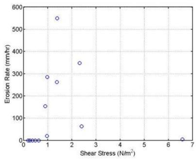
**Figure 6.3** Erosion rate versus shear stress curve for Big Sioux River Bridge; boring B-2 P-14, depth 34.0 to 36.0 ft, silty fine sand. The bed shear stress is for  $\varepsilon = 1$  mm.
