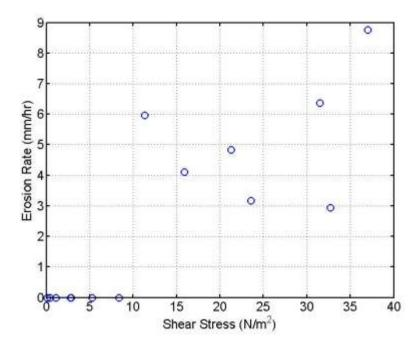
**Figure 6.7** Erosion rate versus shear stress curve for Split Rock Creek bridges; boring B-6 P-6, depth 14.5 to 16.5 ft, silty clay. The bed shear stress is for  $\varepsilon = 1$  mm.
