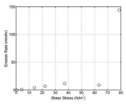
**Figure 6.14** Erosion rate versus shear stress curve from TAMU; boring B-9 P-2, depth 29.0 to 31.0 ft (corresponding to B-7 P-12)
