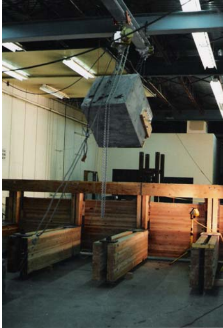
Figure 20 Pendulum test set-up
