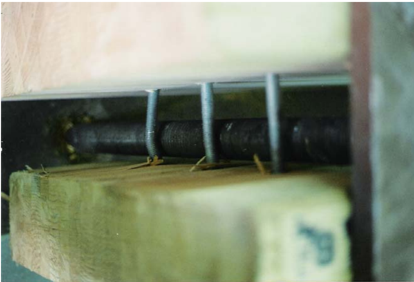
Figure 27 Deformation of steel rods
