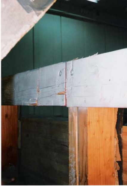
Figure 26 Imprint on rail from pendulum impact
