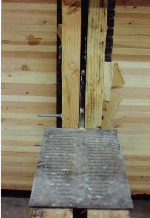
Figure 5 Nailed hanger flange
