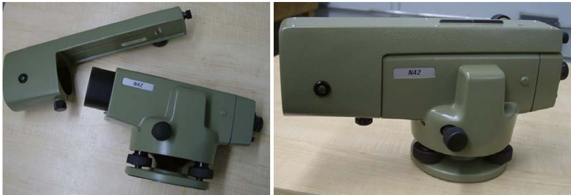
Figure 6.1: Leica NA2 Auto Level and Leica GMP3 Optical Micrometer
