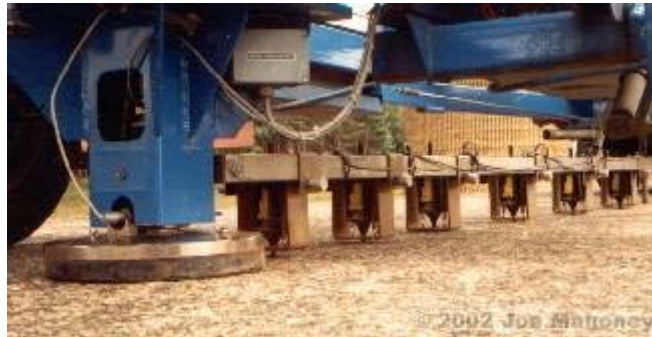
Figure 2.9 FWD Impulse Loading Mechanism
