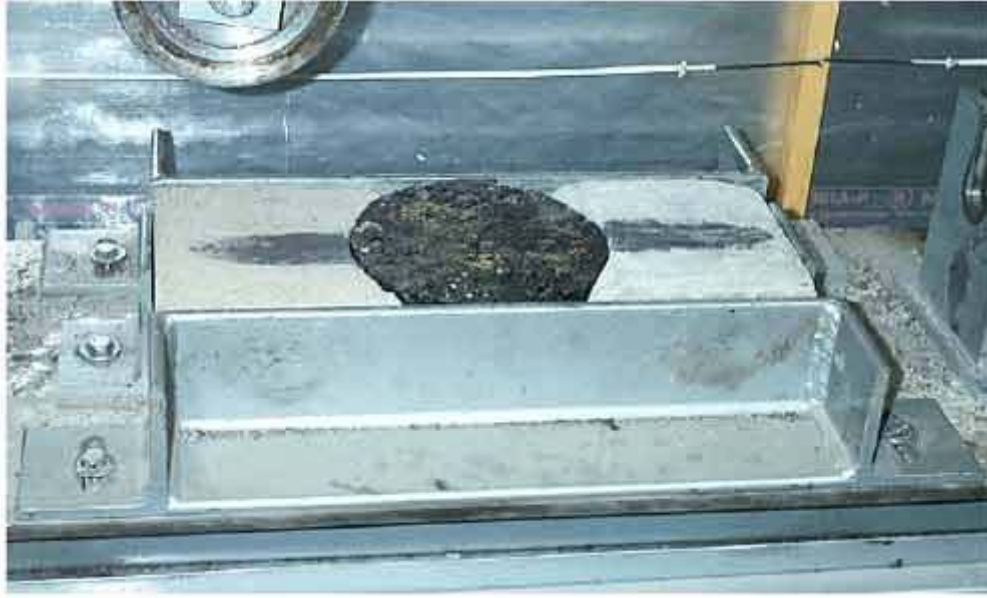
Figure 2.8 GLWT Specimen Held Firm using Concrete Frame
