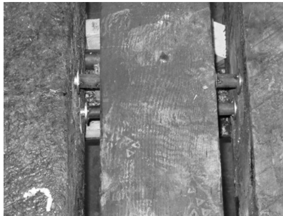
Figure 4.7: Plan view of beams with spacers
