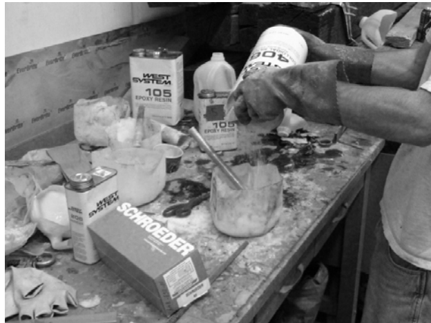
Figure 4.15: Adding silica to epoxy mix
