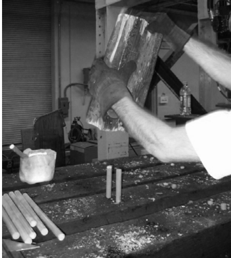
Figure 4.17: Installation of the Z-spikes
