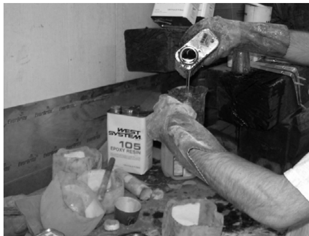
Figure 4.14: Adding resin to epoxy mix
