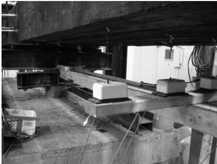
Figure 4.19: String potentiometer setup
