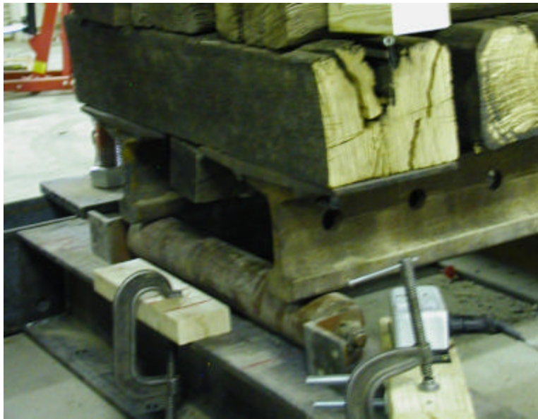
Figure 5. End supports for the test specimen
