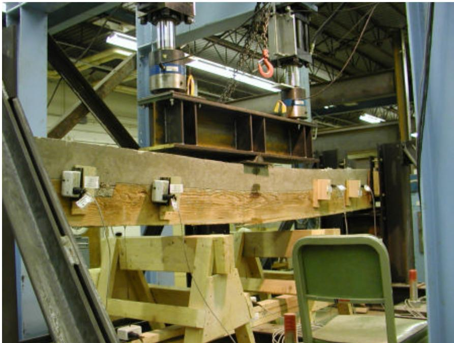
**Figure 2.1 Deep Beam Test Setup**
