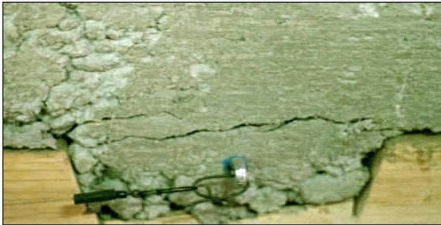
**Figure 3.14 Notch #4 Failure of Wide Beam Specimen #4**
