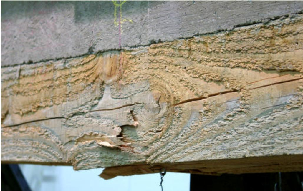
**Figure 3.3 Deep Beam 1 Failure at Mid-Span**
