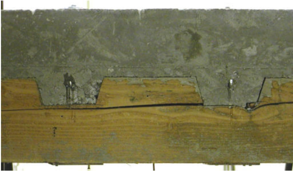
**Figure 3.4 Deep Beam 2 Failure at Notch Connections**
