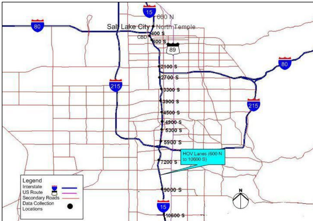
Figure 1.1: HOV Lanes in the Salt Lake Valley showing the data collection locations
