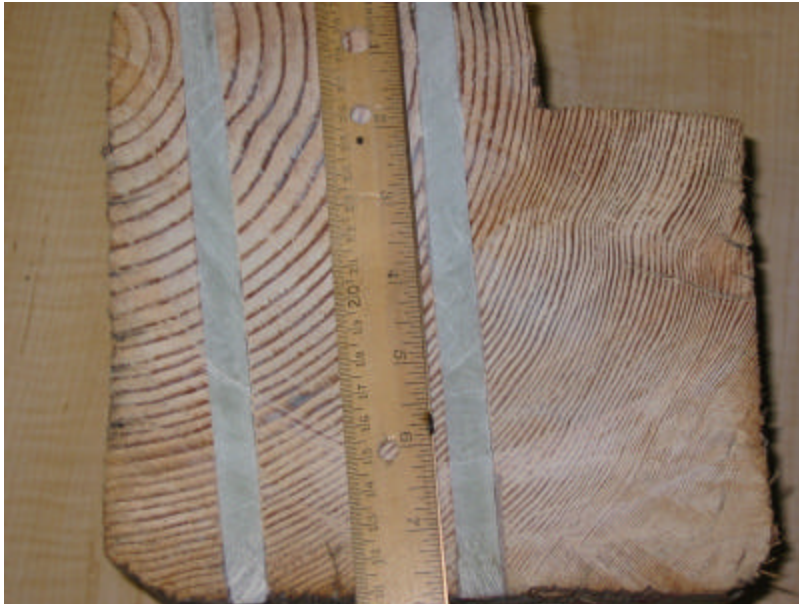
Left - Constant 12.7mm (0.5 in.) diameter hole throughout the depth of the beam Right - Constant 12.7mm (0.5 in.) diameter hole throughout the depth of the beam with 14.3mm (0.5625 in.) diameter countersink.
