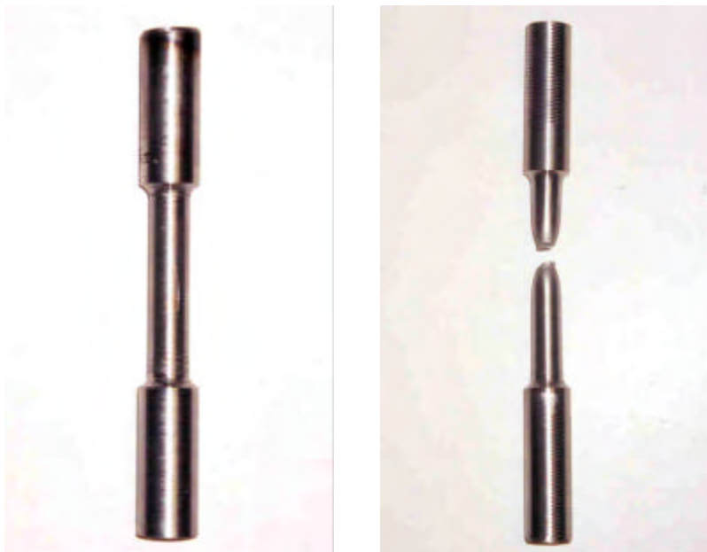
Figure 2.3.1.2 Flange Samples of HPS70W for Uniaxial Tensile Tests - Perpendicular to Rolling Direction
