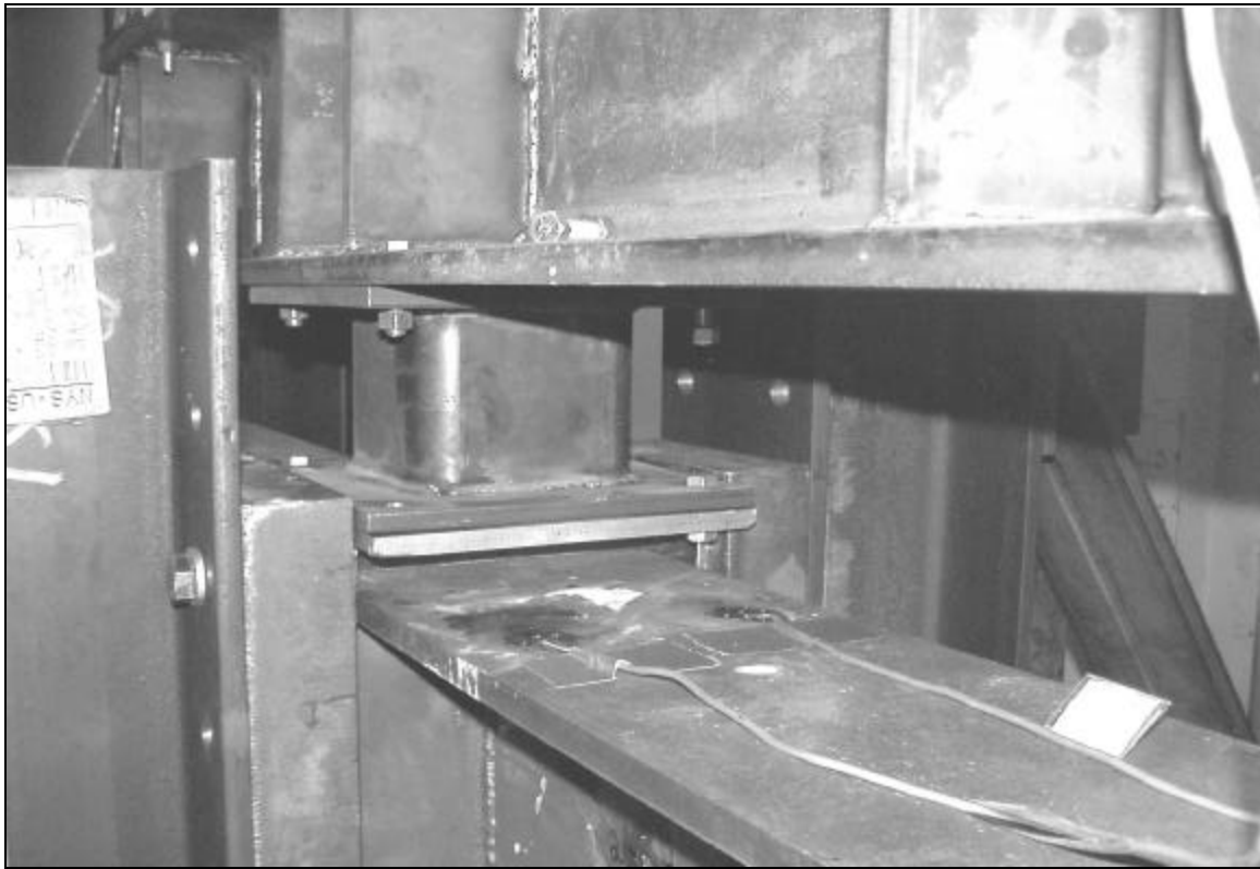
Figure 2.2.2.3 Load Bearing Point
