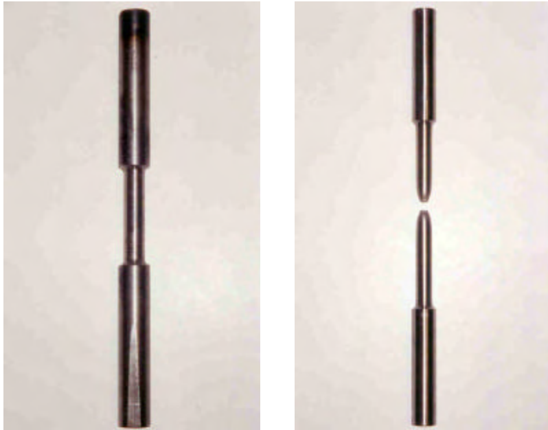
Figure 2.3.1.1 Flange Samples of HPS70W for Uniaxial Tensile Tests - Parallel to Rolling Direction
