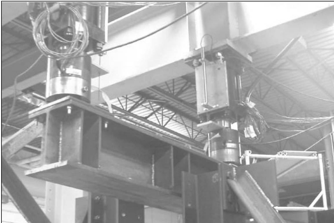
Figure 2.2.2.2 LVDTs, Actuators, Distributor Beam, and the Load Frame Bracing
