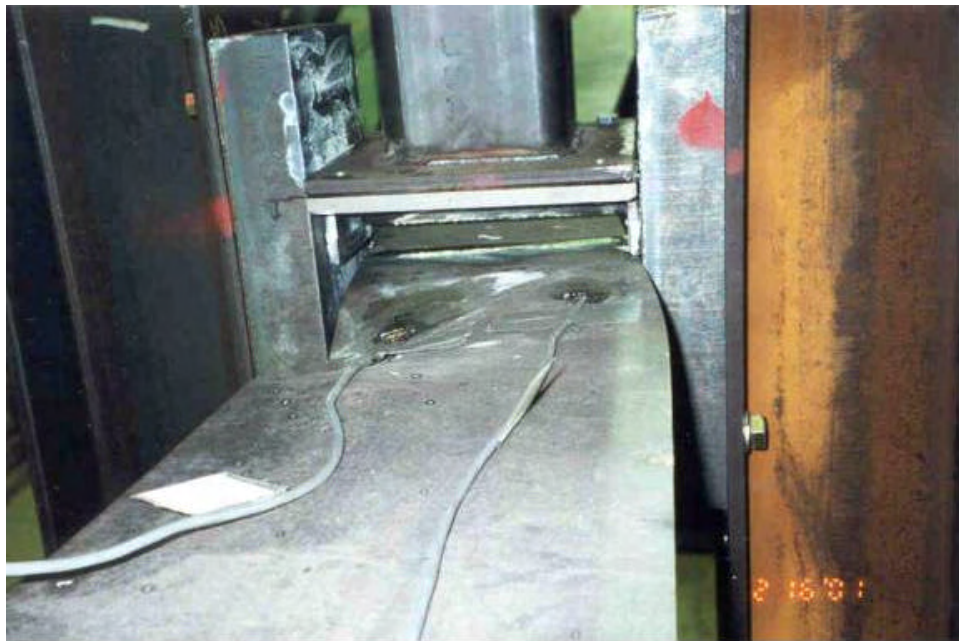
Figure 2.2.4.3 Final Deformed Shapes of Specimen #2 (February 15, 2001)
