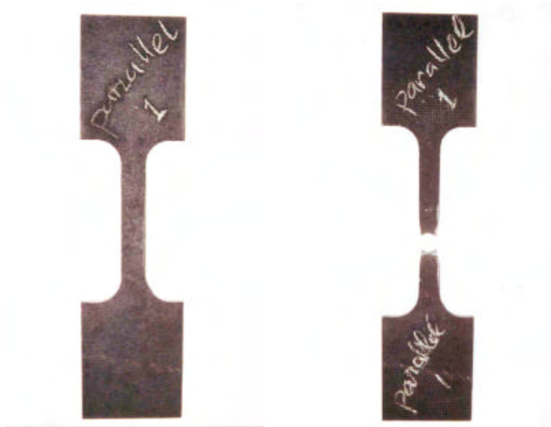
Figure 2.3.1.3 Web samples of HPS70W for Uniaxial Tensile Tests - Parallel to Rolling Direction
