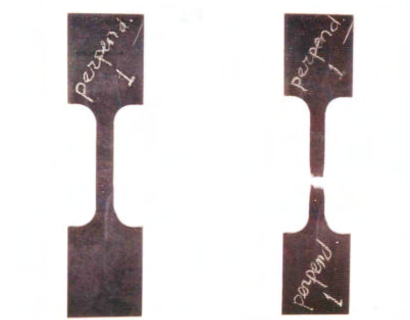
Figure 2.3.1.4 Web Samples of HPS70W for Uniaxial Tensile Tests - Perpendicular to Rolling Direction
