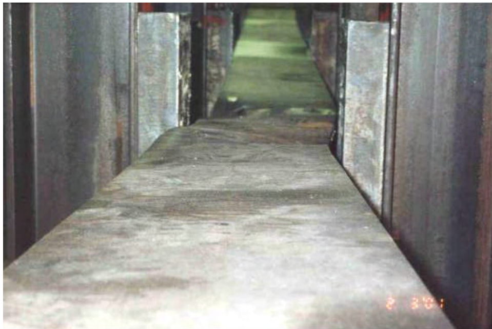
Figure 2.2.4.2 Final Deformed Shapes of Specimen #1 (February 1, 2001)
