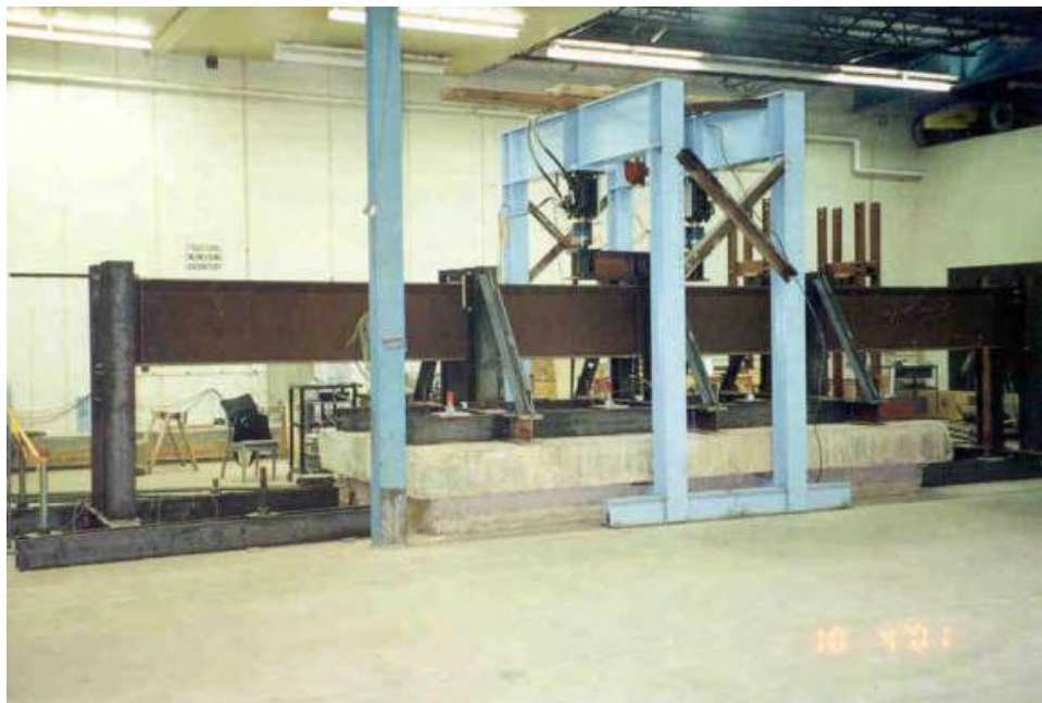
Figure 2.2.4.4 Above: Midspan Deformed Shape of Specimen #3 (August 1, 2001) Below: Specimen #4 after first tested (October 4, 2001)
