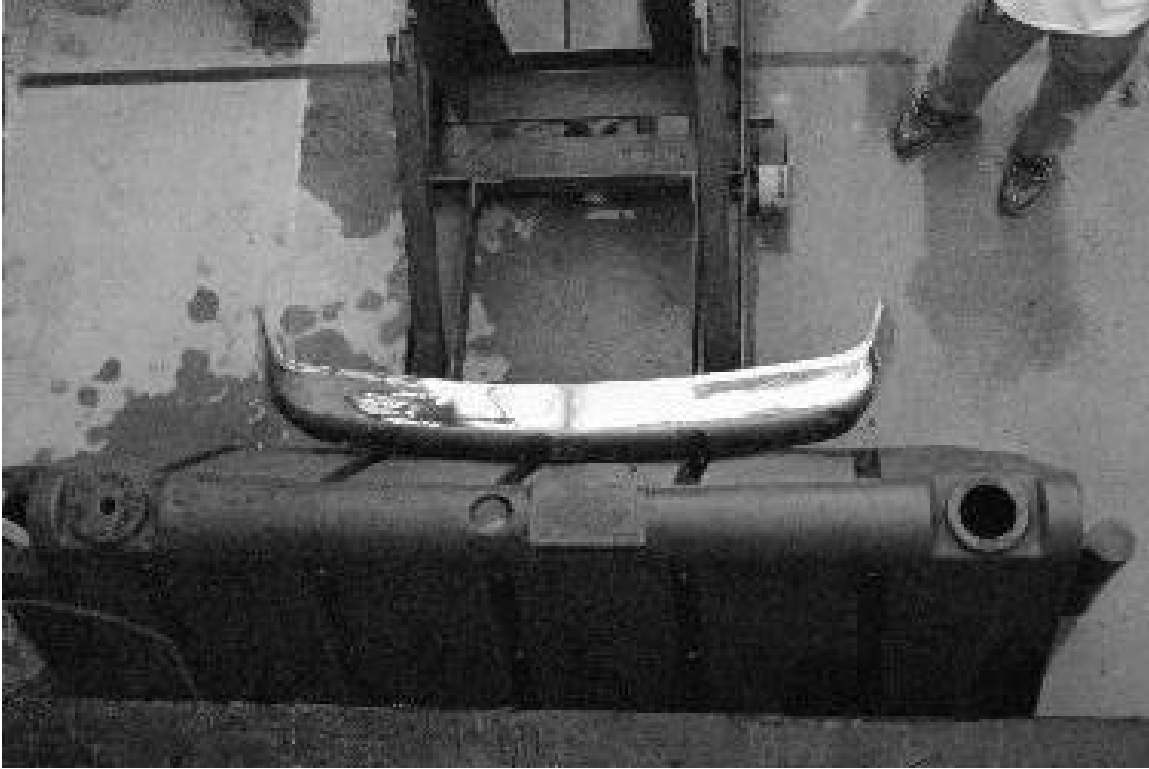
Figure 4.2: Position of the unloaded surrogate test vehicle and single test specimen following the trial run.
