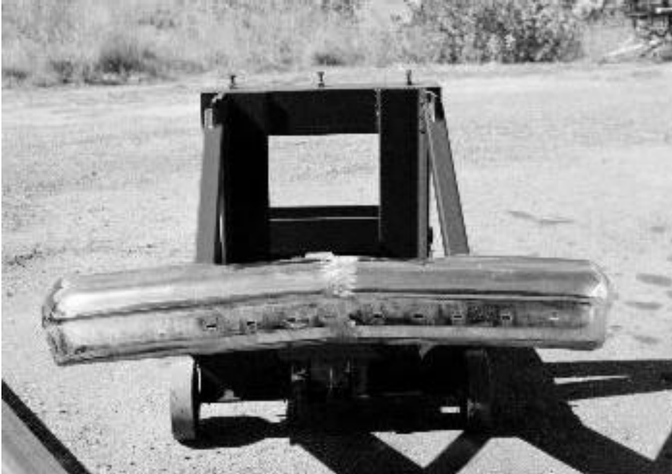
Figure 3.7: Ford light truck bumper installed on surrogate test vehicle.
