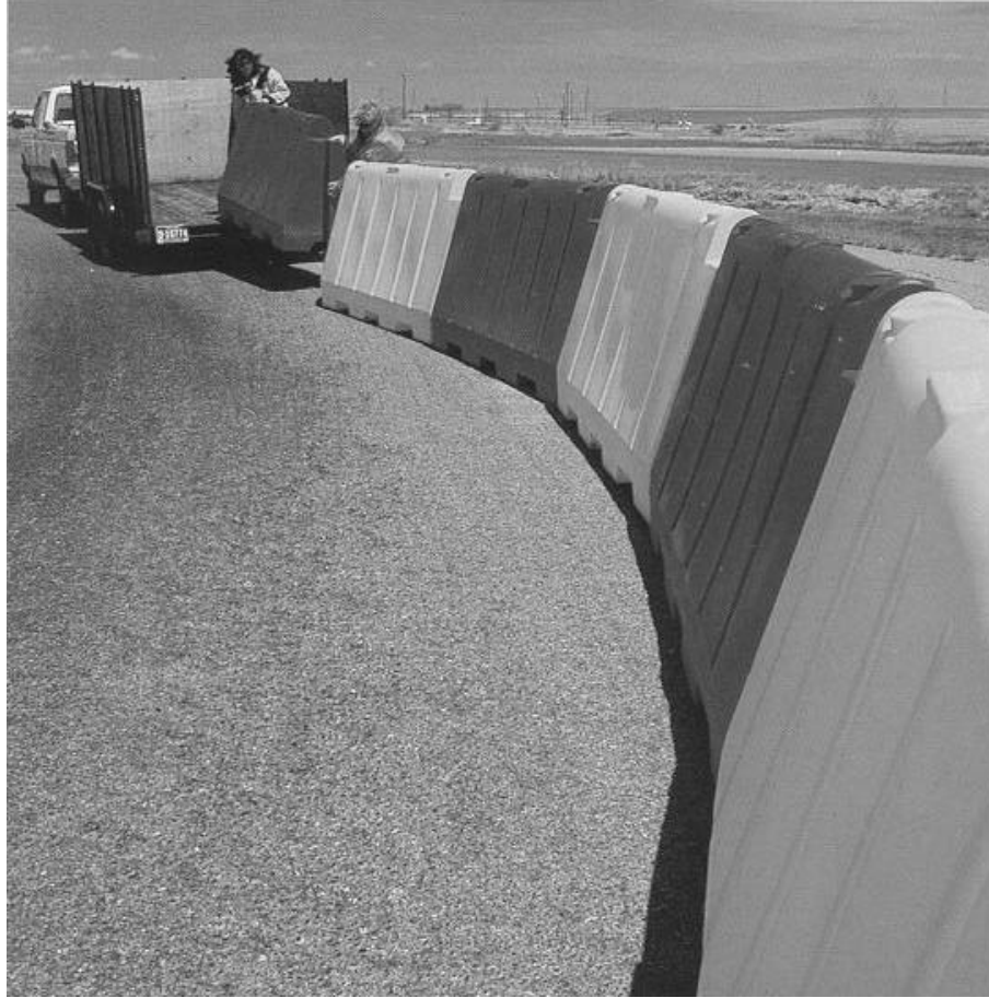
Figure 3.11: Assembly of an interconnected line of barrier specimens in the field.
