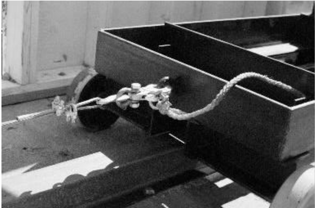
Figure 3.9: Quick-release connecting the winch cable to the surrogate test vehicle.
