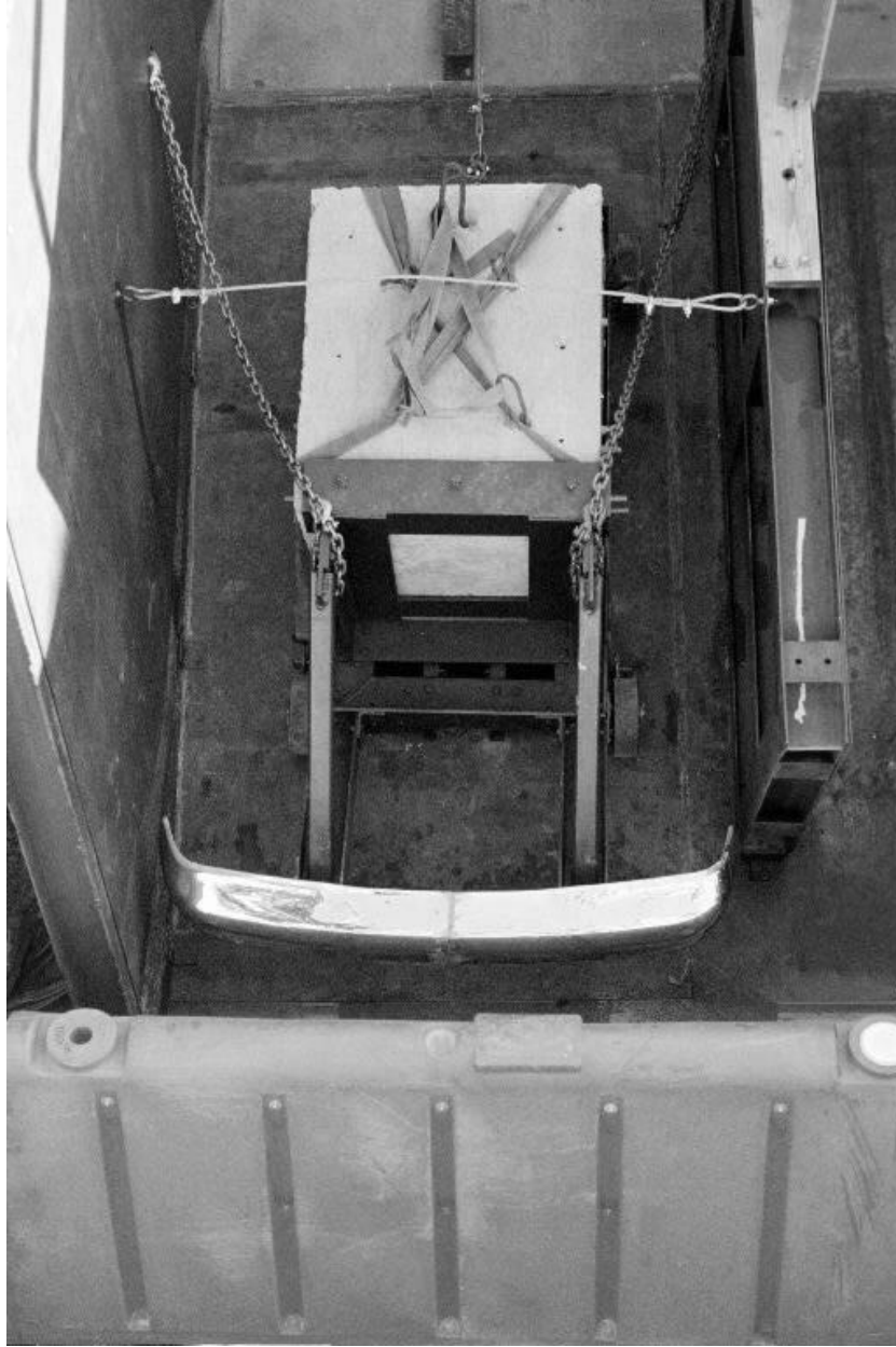
Figure 4.3: Surrogate test vehicle loaded with the concrete block and chained to the flume to permit safe barrier placement. Also visible are the safety cable, tiedown straps, and the end of the guide rail.
