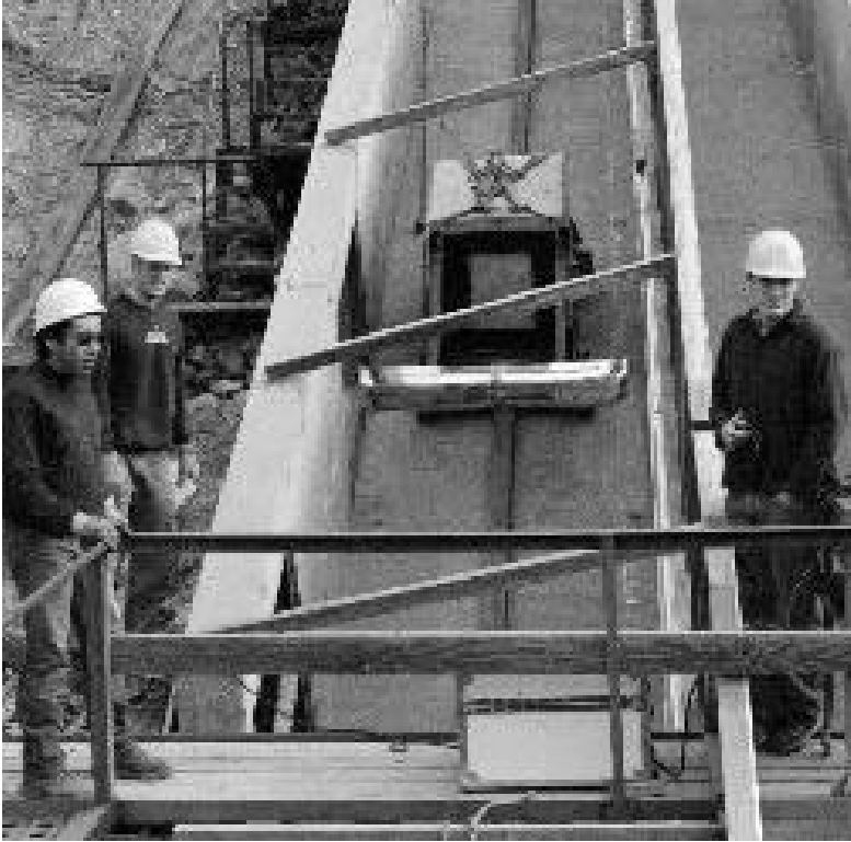
Figure 4.5: Surrogate test vehicle hoisted to the release height for test level 2.
