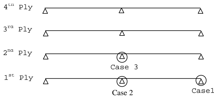
Figure 1.67: Locations of Unsupported Plies – 2-Span Bridge Chord
